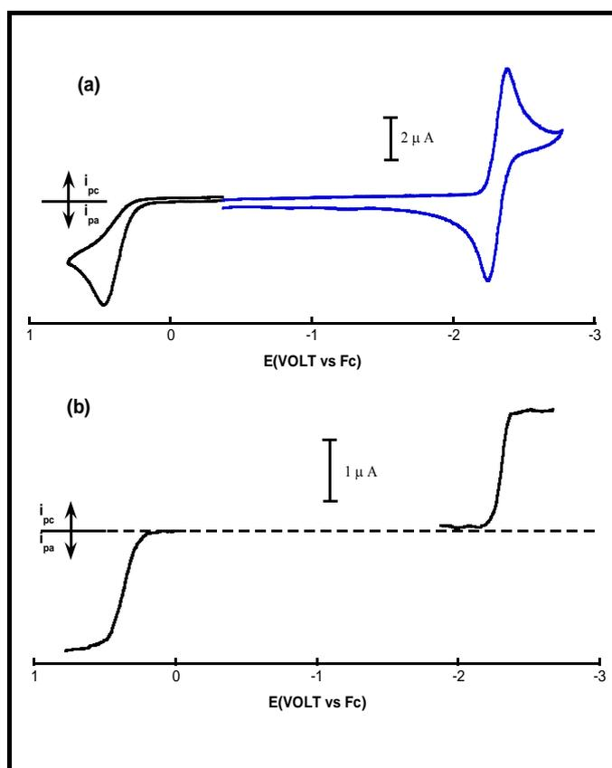
**Figure 4.** (a) Cyclic voltammograms of 1.3 mM **1** in THF/0.05 M  $[\text{NBu}_4][\text{B}(\text{C}_6\text{F}_5)_4]$  at scan rate of 200 mV/s, 298K and 1 mm GC disk electrode. (b) Linear sweep voltammograms recorded under the same conditions, scan rate of 5 mV/s.
