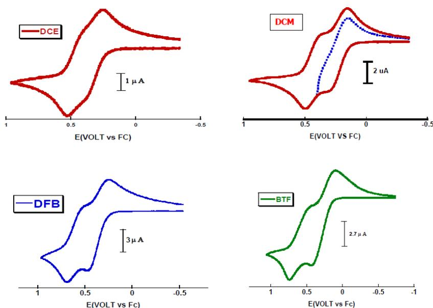
**Figure 3.** Cyclic voltammograms obtained at scan rate of 0.1 V/s and 1mm GC disk electrode for oxidation of  $\sim 1.5$  mM  $\text{CpCo}(\text{CO})_2$  using designated solvent and 0.05 M  $[\text{NBu}_4][\text{B}(\text{C}_6\text{F}_5)_4]$ .
