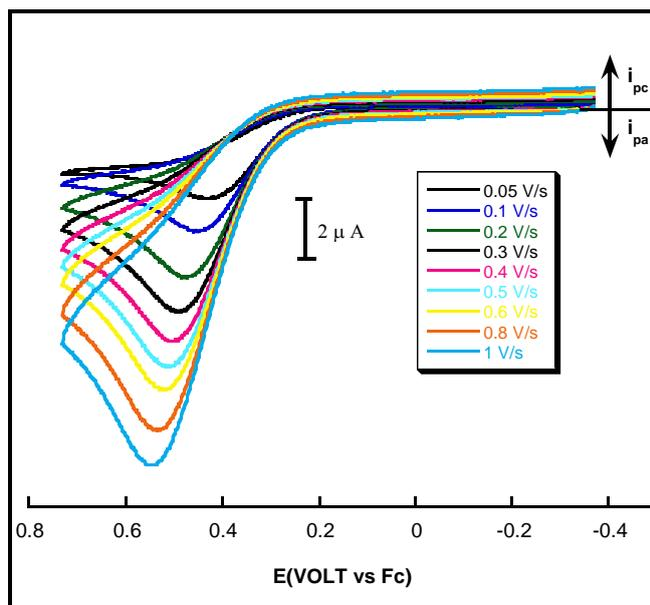
**Figure 5.** Cyclic voltammograms of 1.3 mM **1** in THF/0.05 M [NBu<sub>4</sub>][B(C<sub>6</sub>F<sub>5</sub>)<sub>4</sub>] at different scan rates, 298K and 1 mm GC disk electrode.
