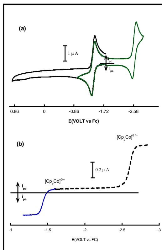
**Figure 8.** (a) Cyclic voltammograms recorded after back electrolysis of 1.3 mM **1** in THF/0.05 M  $[\text{NBu}_4][\text{B}(\text{C}_6\text{F}_5)_4]$  at  $E_{\text{app}} = -1.6$  V, scan rate = 200 mV/s, 298K and 1 mm GC disk electrode. (b) Linear sweep voltammograms recorded under the same conditions, scan rate of 5 mV/s.
