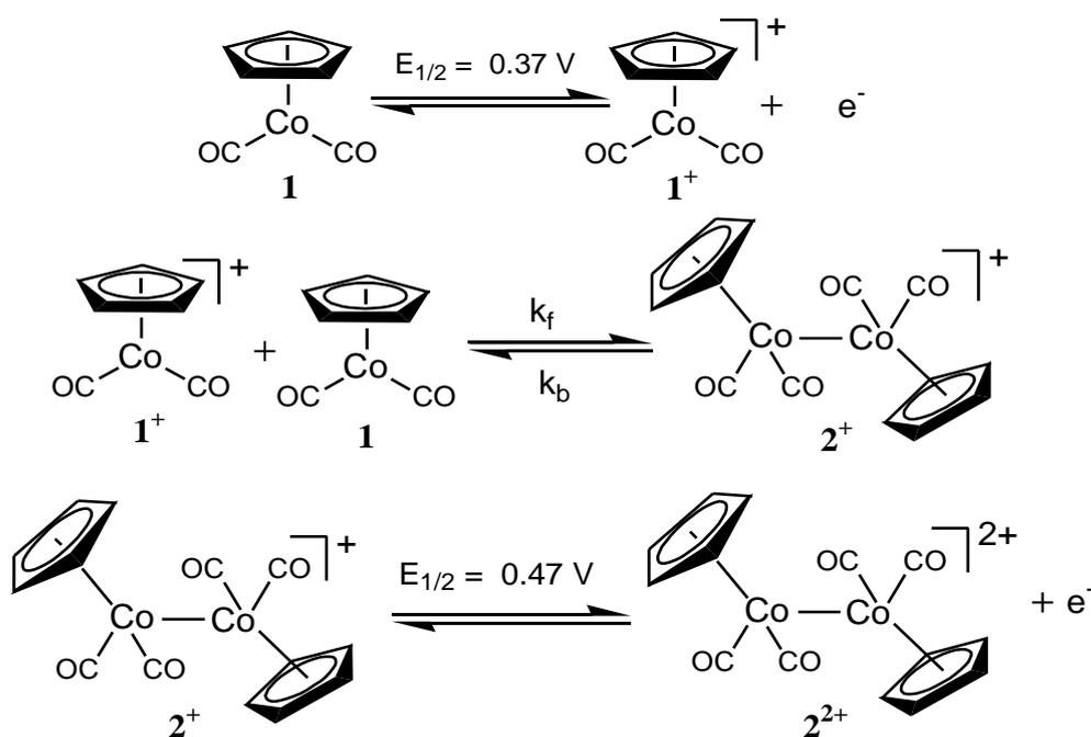
**Scheme 1.** R-S dimerization reaction of **1**
