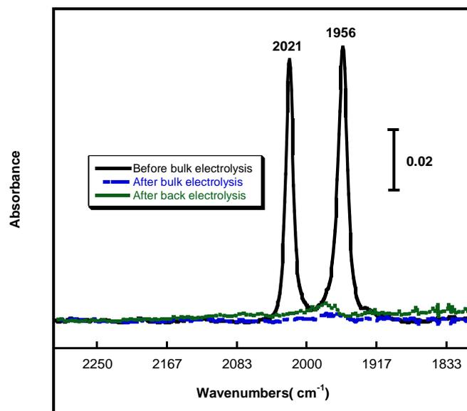
**Figure 7.** IR spectra of 1.3 mM **1** in THF/0.05 M  $[\text{NBu}_4][\text{B}(\text{C}_6\text{F}_5)_4]$  obtained before and after bulk electrolysis and after back electrolysis.
