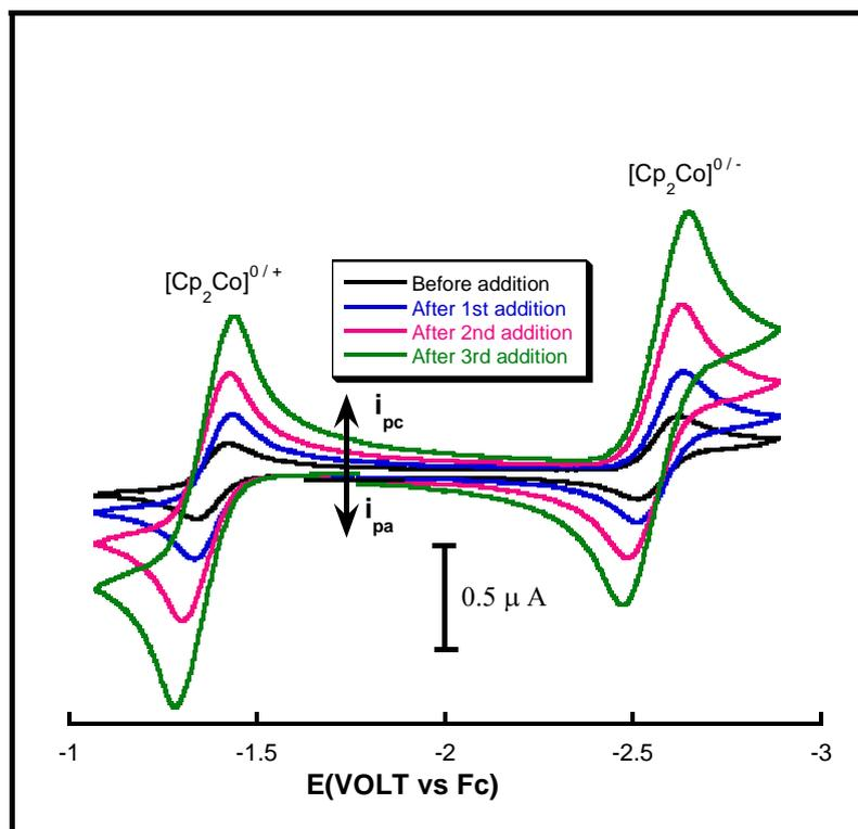
**Figure 9.** Cyclic voltammograms recorded after back electrolysis of 1.3 mM **1** in THF/0.05 M  $[\text{NBu}_4][\text{B}(\text{C}_6\text{F}_5)_4]$  at  $E_{\text{app}} = -1.6$  V, scan rate = 200 mV/s, 298K and 1 mm GC disk electrode and after addition of successive amounts of  $\text{Cp}_2\text{Co}$ .
