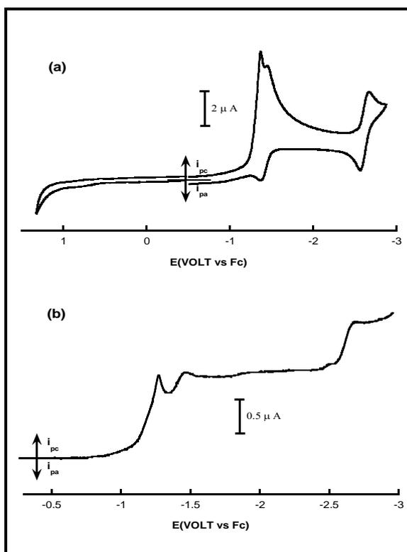
**Figure 6.** (a) Cyclic voltammograms recorded after bulk electrolysis of 1.3 mM **1** in THF/0.05 M  $[\text{NBu}_4][\text{B}(\text{C}_6\text{F}_5)_4]$  at  $E_{\text{app}} = 0.75$  V, scan rate = 200 mV/s, 298K and 1 mm GC disk electrode. (b) Linear sweep voltammograms recorded under the same conditions, scan rate of 5 mV/s.
