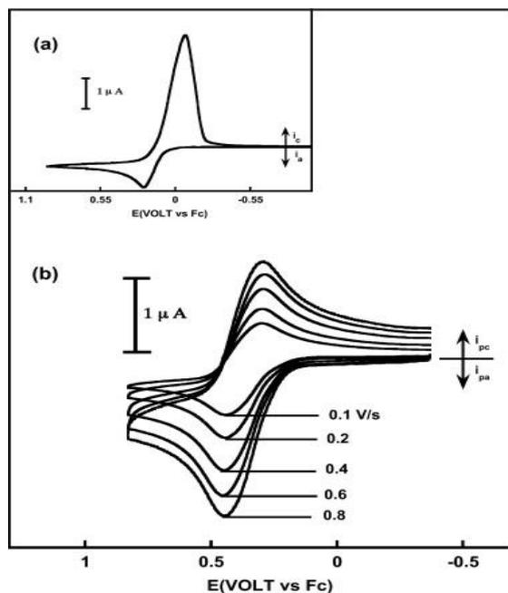
**Figure 1.** (a) Cyclic Voltammogram of 2 mM **1** in  $\text{CH}_2\text{Cl}_2/0.1 \text{ M } [\text{NBu}_4][\text{PF}_6]$  at scan rate of 0.1 V/s, 298 K on a 1mm GC disk. (b) Cyclic voltammograms of 0.25 mM **1** in  $\text{CH}_2\text{Cl}_2/0.05 \text{ M } [\text{NBu}_4][\text{B}(\text{C}_6\text{F}_5)_4]$  at different scan rates, 298 K on a 1mm GC disk.
