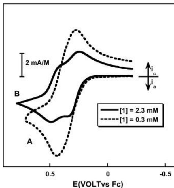
**Figure 2.** Cyclic voltammograms of **1** in  $\text{CH}_2\text{Cl}_2/ 0.05 \text{ M } [\text{NBu}_4][\text{B}(\text{C}_6\text{F}_5)_4]$  at 298 K, 1 mm GC disk and scan rate of 0.5 V/s at two different concentrations; y-axis is concentration-normalized current.
