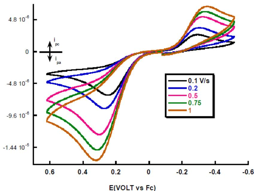
**Figure 10.** Cyclic voltammograms of 1.5 mM **1** in  $\text{CH}_3\text{NO}_2/0.05 \text{ M } [\text{NBu}_4][\text{B}(\text{C}_6\text{F}_5)_4]$  at designated scan rates, 298K and 1 mm GC disk electrode.
