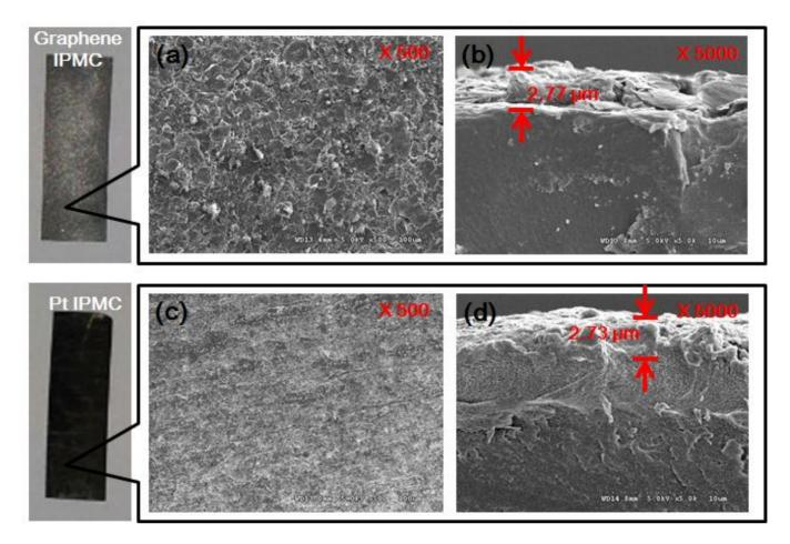
Figure 3. SEM image comparison of graphene based IPMC and platinum based IPMC. (a) Surface SEM image of graphene based IPMC. (b) Cross sectional SEM image of graphene based IPMC. (c) Surface SEM image of platinum based IPMC. (d) Cross sectional SEM image of platinum based IPMC.
