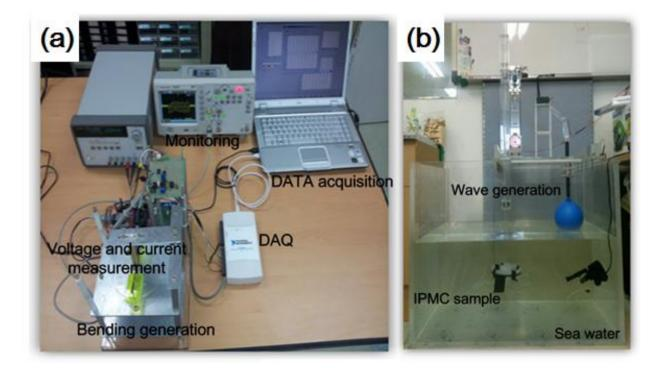
**Figure 1.** (a) An experimental apparatus in air and (b) an experimental simulator in seawater for evaluating the conversion performance from kinetic energy to electrical energy with graphene-based IPMC and Pt-based IPMC.
