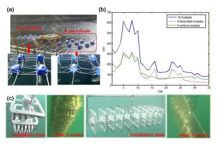
**Figure 6.** Performance of the ocean kinetic energy harvesting module with the conductive graphenebased solution IPMC. (a) Photograph of the ocean kinetic energy harvesting module. (b) History of the electrical energy harvested with the ocean kinetic energy harvesting module from ocean currents and waves. (c) Photographic comparison of the vertical and horizontal components between the day of installation and after 3 weeks.
