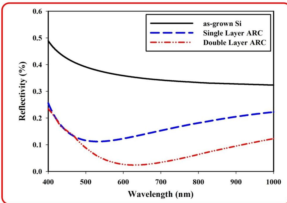
Figure 5. Shows the reflectance spectra for SLAR and DLAR coatings with the as-grown Si sample.
