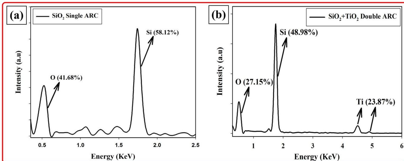
**Figure 2.** EDX spectra (a) SiO<sub>2</sub> film, (b) SiO<sub>2</sub>/TiO<sub>2</sub> film.
