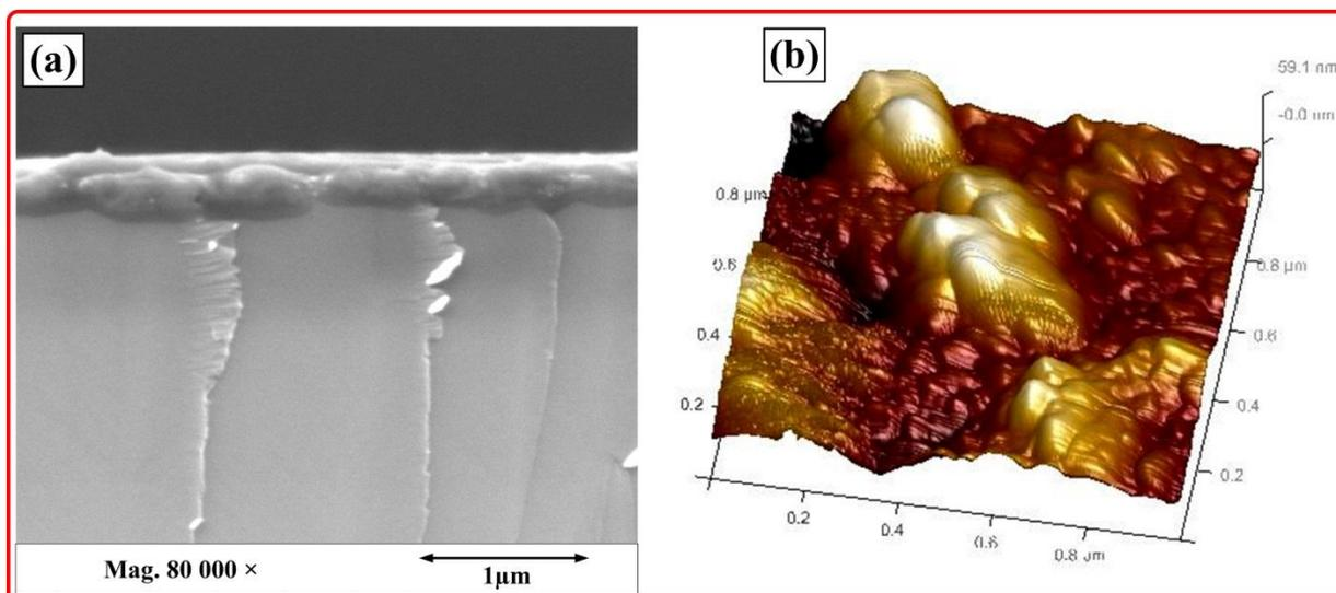
**Figure 3.** Al-alloyed p<sup>+</sup> layer (a) FESEM cross sectional view (b) AFM back side view.
