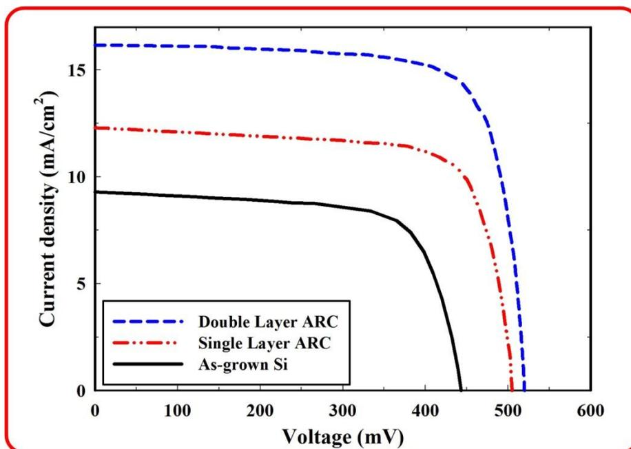
Figure 6. Shows the *I-V* graphs formed with SLAR (SiO<sub>2</sub>) and DLAR (SiO<sub>2</sub>/TiO<sub>2</sub>) coatings with the as-grown Si solar cell.
