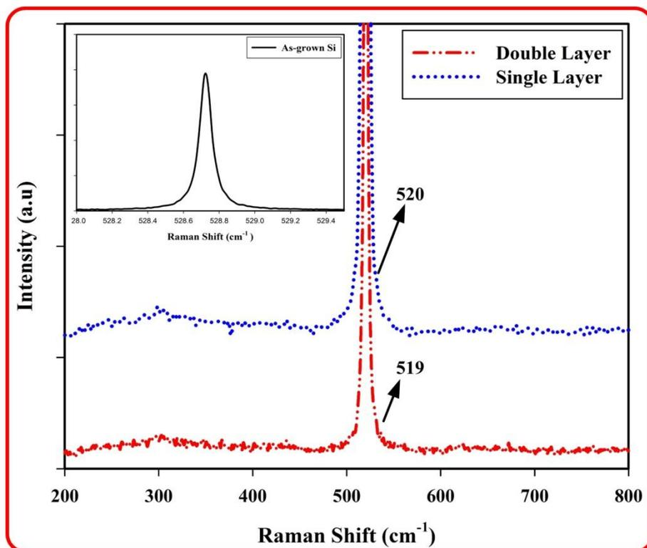
**Figure 4.** Raman spectra of the  $\text{SiO}_2$  and  $\text{SiO}_2/\text{TiO}_2$  coatings deposited on the c-Si  $p$ -type (100).
