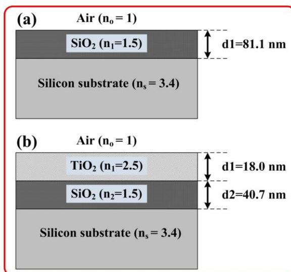
**Figure 1.** Schematic diagram of antireflection coatings (a) SLAR (SiO<sub>2</sub>) (b) DLAR (SiO<sub>2</sub>/TiO<sub>2</sub>).
