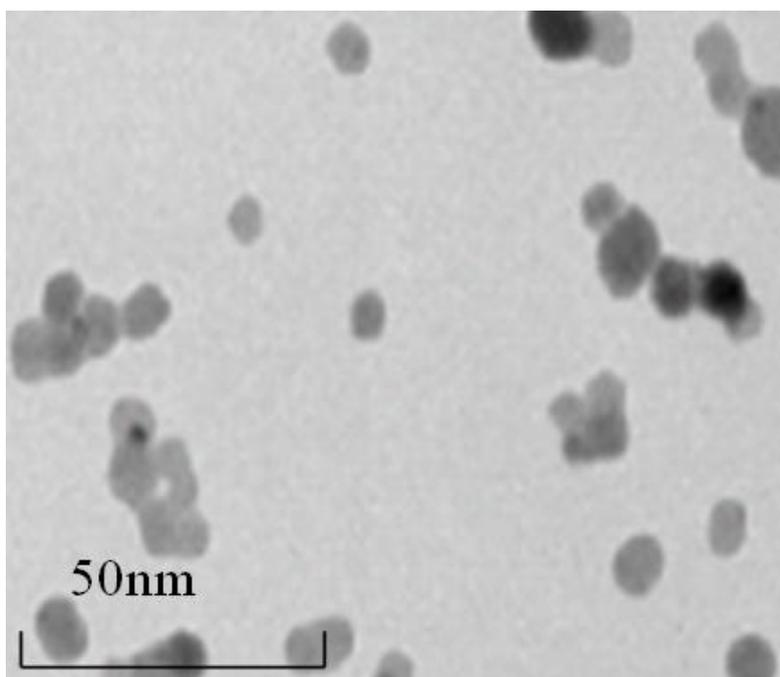
**Figure 2.** TEM image of the synthesized PdS nanoparticles
