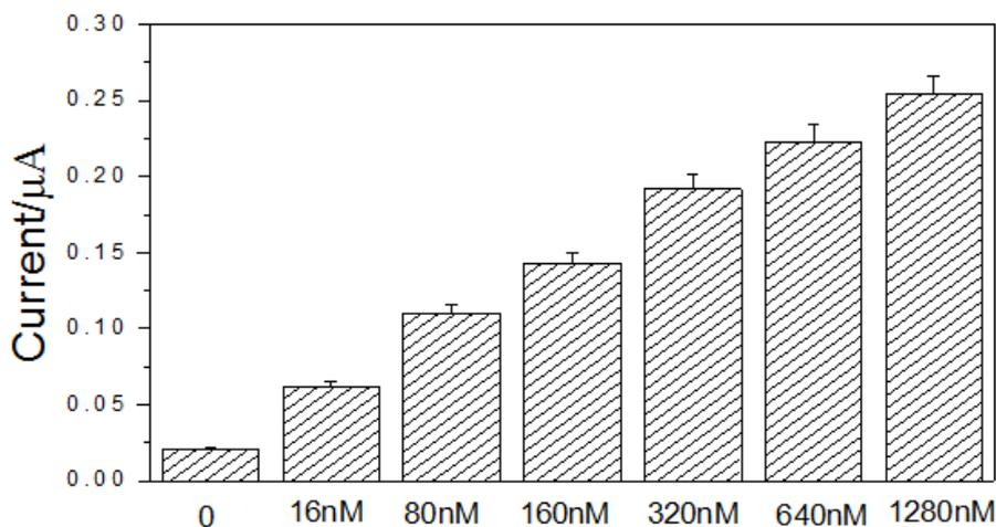
**Figure 4.** Graph of average DPV signal intensity as a function of the Hg<sup>2+</sup> concentration in buffer.
