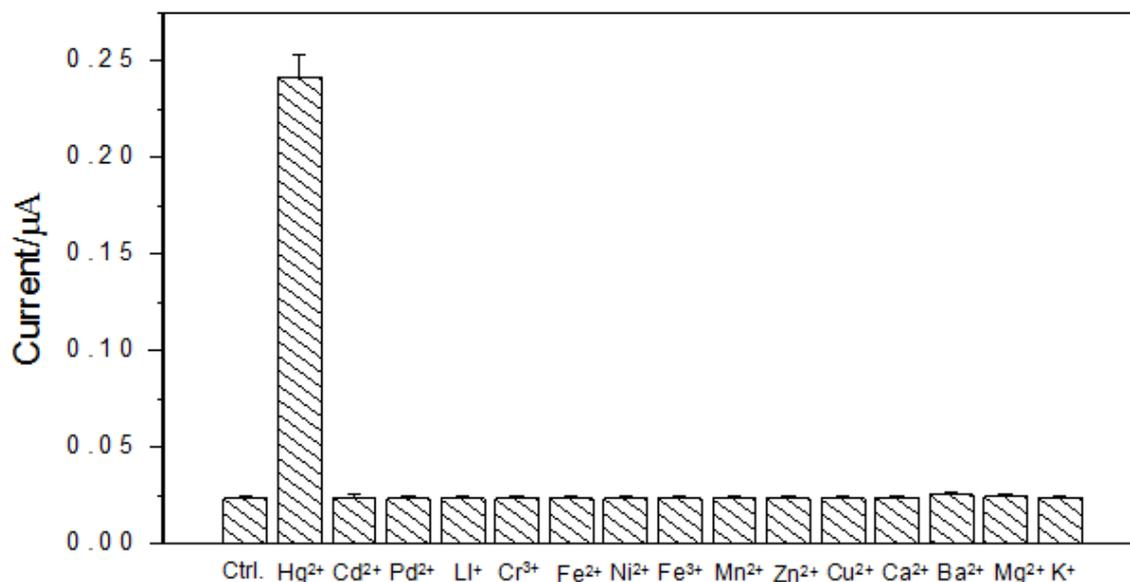
**Figure 5.** DPV response of the assay in the presence of various metal ions ( $[\text{M}^{x+}] 1 \mu\text{mol L}^{-1}$ ).
