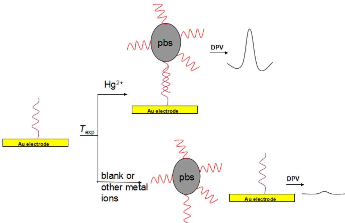
**Figure 1.** Schematic representation of the procedure to prepare electrochemical biosensor for the determination of mercury (II).
