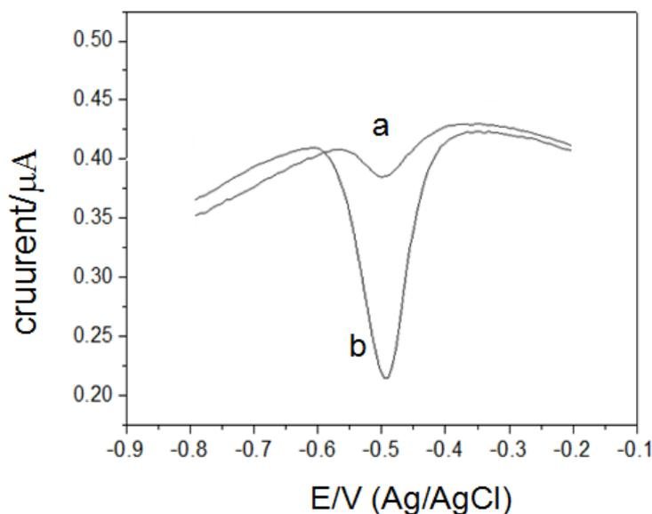
**Figure 3.** DPV response of the biosensor in the prepared solution containing 1 nmol  $\text{L}^{-1}$  DNA-PbS (a) without  $\text{Hg}^{2+}$  (b) in the presence of  $\text{Hg}^{2+}$  ( $c = 1280$  nmol  $\text{L}^{-1}$ ).
