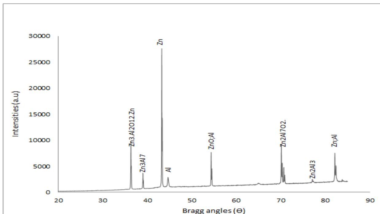
Figure 4. XRD Spectral of Zn-Al<sub>2</sub>O<sub>3</sub>+Tea/Mea in 10 minutes at 0.8 V
