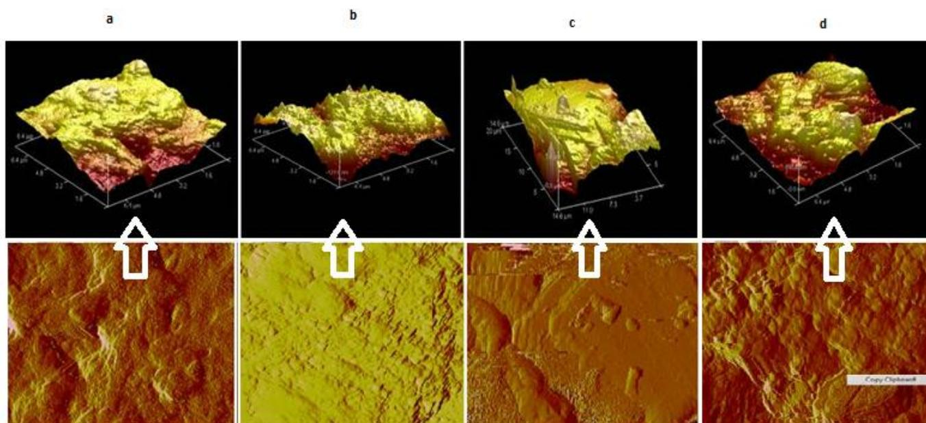
**Figure 3:** AFM micrographs of [a] Zn-Al<sub>2</sub>O<sub>3</sub>+Tea/Mea 10min at 0.5 V [b] Zn-Al<sub>2</sub>O<sub>3</sub>+Tea/Mea 10min at 0.8V [c]Zn-Al<sub>2</sub>O<sub>3</sub>+Tea/Mea 15min at 0.5V [d] Zn-Al<sub>2</sub>O<sub>3</sub>+Tea/Mea 15min at 0.8 V.
