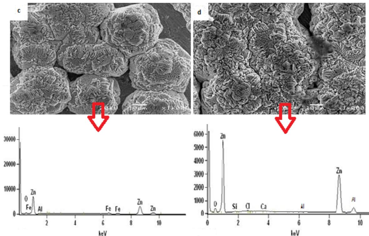
**Figure 2.** SEM/EDS micrographs [c] Zn-Al<sub>2</sub>O<sub>3</sub>+Tea/Mea 15min at 0.5 V [d] Zn-Al<sub>2</sub>O<sub>3</sub>+Tea/Mea 15min at 0.8 V -X1000 magnification
