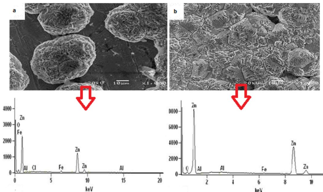
Figure 2. SEM micrographs of [a] Zn-Al<sub>2</sub>O<sub>3</sub>+Tea/Mea 10min at 0.5 V [b] Zn-Al<sub>2</sub>O<sub>3</sub>+Tea/Mea 10min at 0.8 V -X1000 magnification
