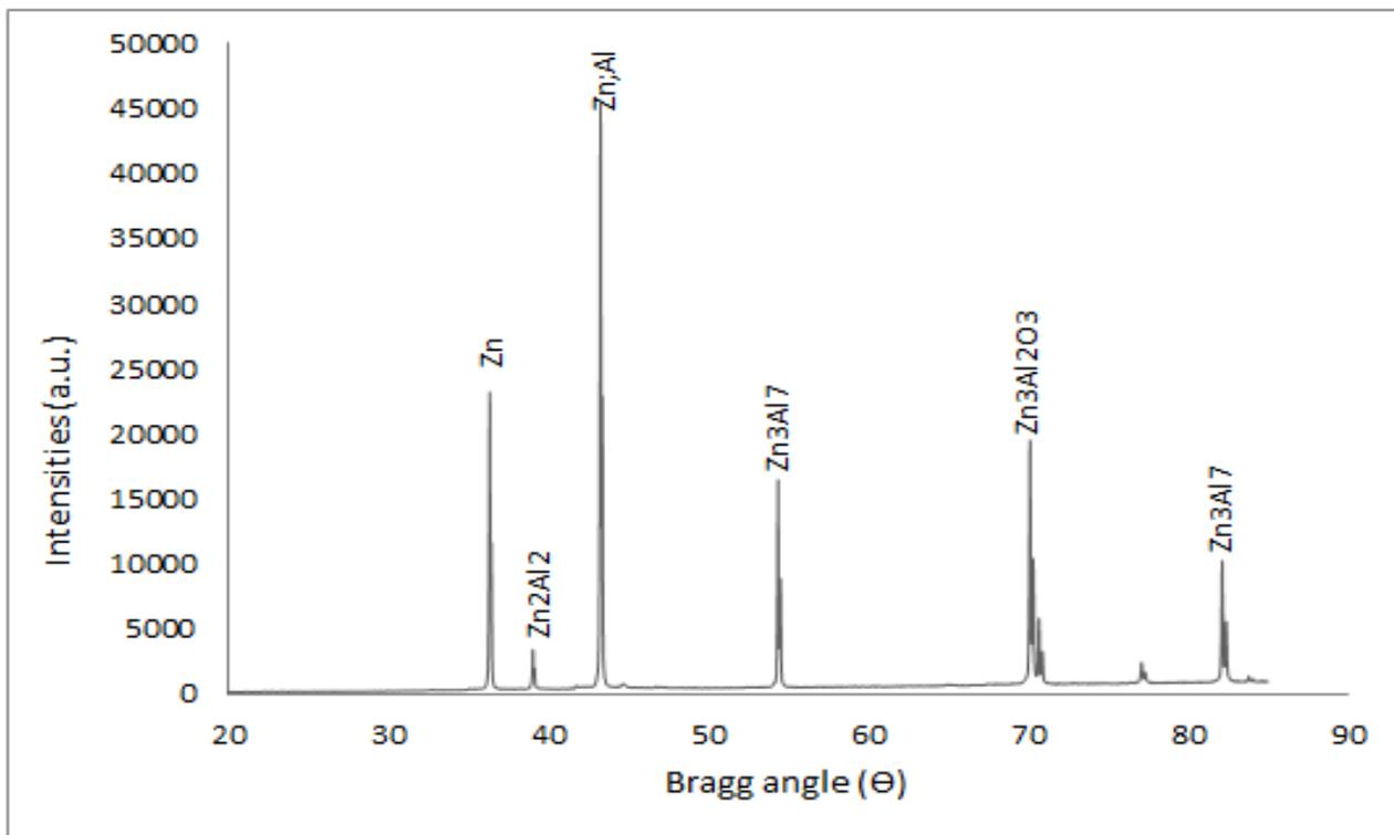
Figure 5. XRD Spectral of Zn-Al<sub>2</sub>O<sub>3</sub>+Tea/Mea in 15 minutes at 0.8 V
