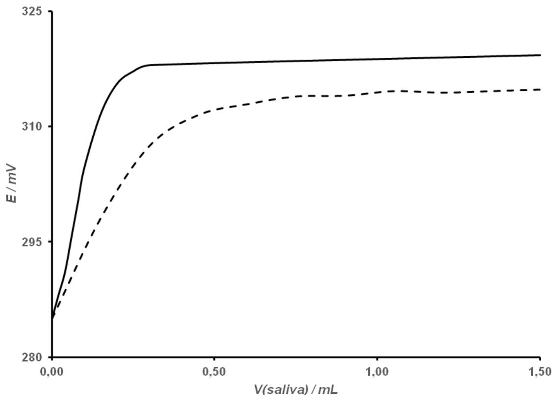
**Figure 2.** The typical responses of a platinum redox sensor in the rower saliva samples before (dashed line) and after (full line) the training.
