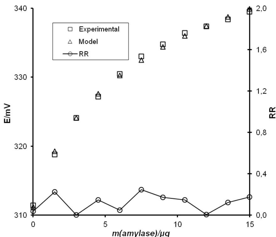
**Figure 1.** Comparison of experimental ( $\square$ ) and modeled ( $\Delta$ ) response characteristics of a platinum redox sensor toward  $\alpha$ -amylase (triiodide concentration  $100 \mu\text{M}$ , iodide concentration  $0.05 \text{ M}$ , starch concentration  $5 \text{ mg/mL}$ ). The values of the squared residuals RR ( $\circ$ ) are presented on the secondary Y-axis.
