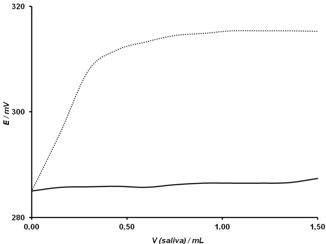
**Figure 4.** The typical responses of a platinum redox sensor in the saliva samples before (dotted line) and after (full line) alcohol consumption.
