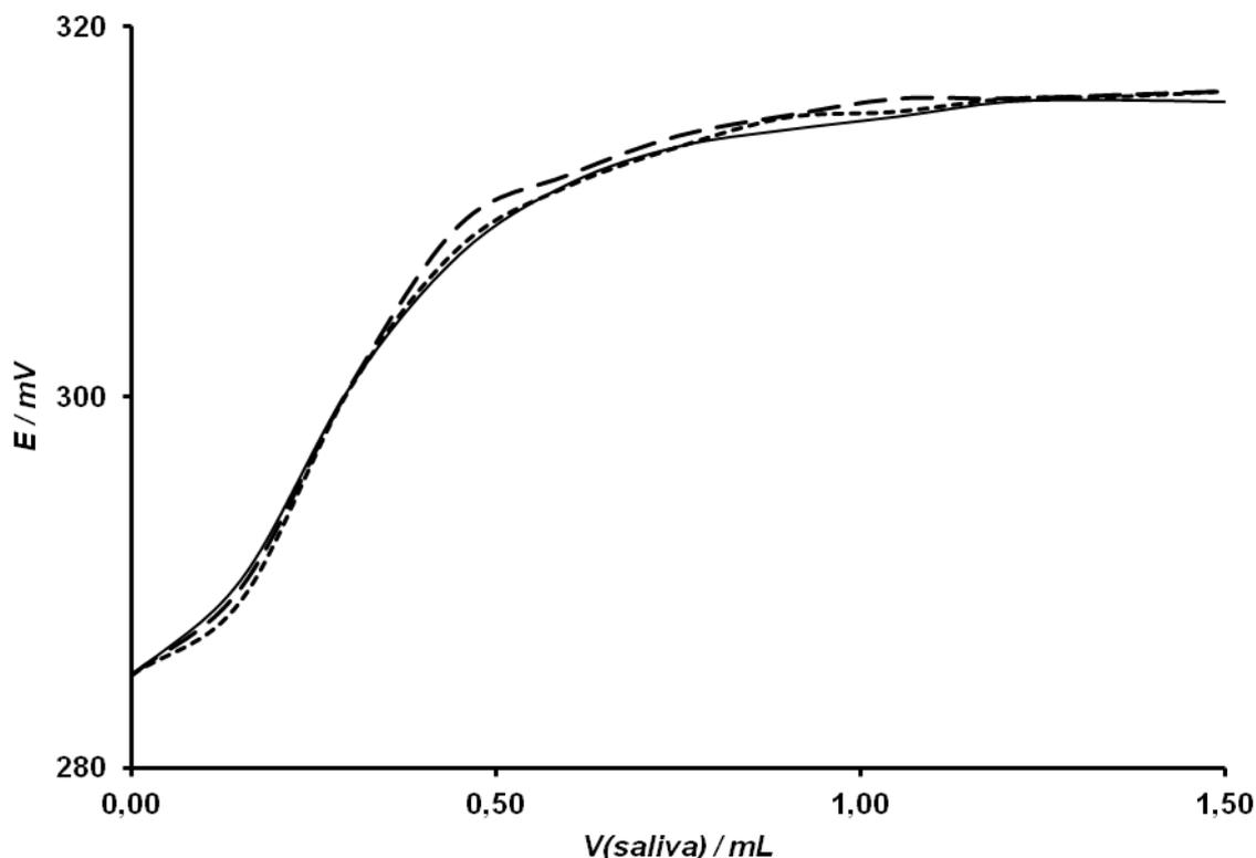
**Figure 3.** The responses of a platinum redox sensor for the 3 series of measurements in the same rowler saliva sample before the training.
