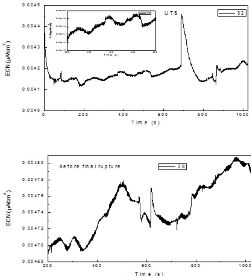
**Figure 3.** Noise in current for S41425 steel strained in the H<sub>2</sub>S-containing 3.5% NaCl solution at 40 <sup>0</sup>C
