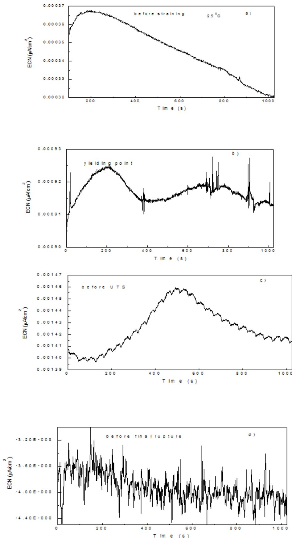
**Figure 2.** Noise in current for S41425 steel in the H<sub>2</sub>S-containing 3.5% NaCl solution at 25 °C
