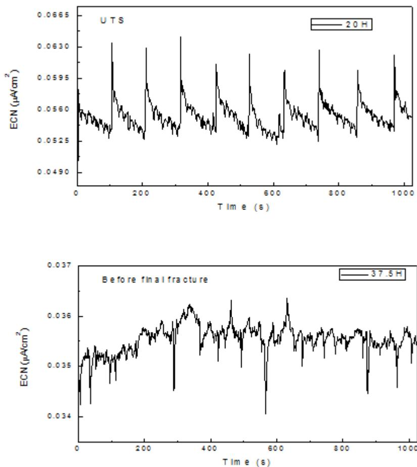
**Figure 6.** Noise in current for S41425 steel strained in the  $\text{H}_2\text{S}$ -containing 3.5% NaCl solution at  $80^{\circ}\text{C}$
