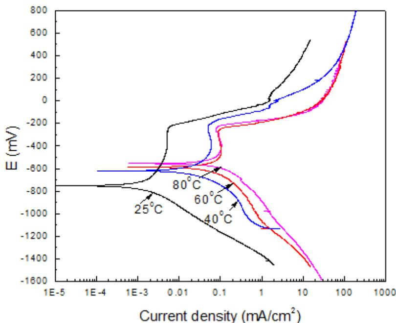
**Figure 1.** Effect of the temperature in the polarization curves for S41425 in a H<sub>2</sub>S-containing 3.5% NaCl solution.
