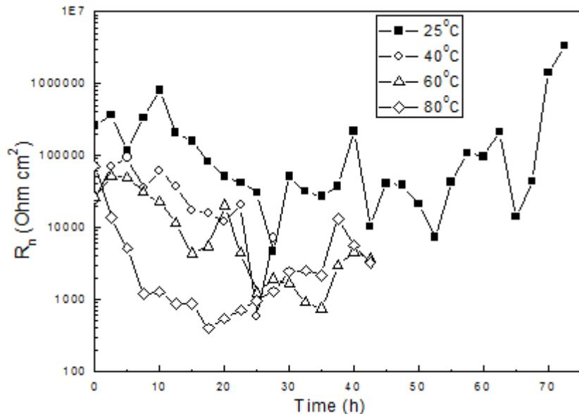
**Figure 10.** Variation of the noise resistance value,  $R_n$ , with time for the different SSRT experiments.
