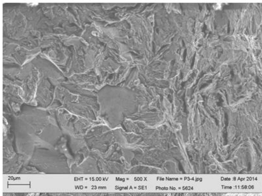
**Figure 5.** SEM micrograph of S41425 steel fractured in the  $\text{H}_2\text{S}$ -containing 3.5% NaCl solution at  $60^{\circ}\text{C}$
