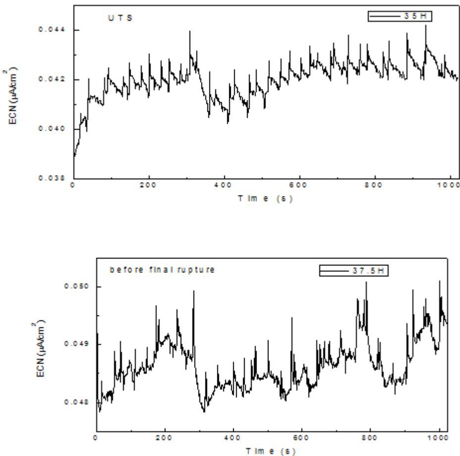
**Figure 4.** Noise in current for S41425 steel in strained in the  $\text{H}_2\text{S}$ -containing 3.5% NaCl solution at 60  $^{\circ}\text{C}$  a) before straining, b) at the yielding point, c) near the UTS and d) before final fracture.
