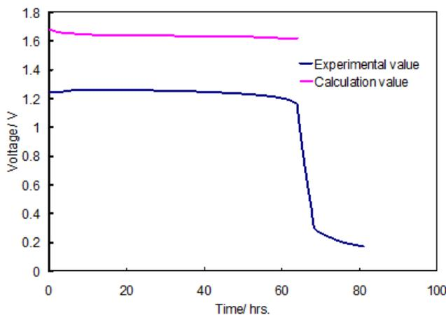
**Figure 7.** Comparison of discharge curves for Mg and Zn mixed button battery
