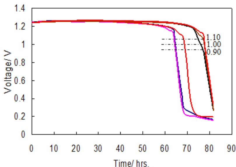
**Figure 6.** Continuous discharge curves of Mg and Zn mixed button batteries
