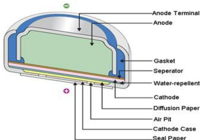
**Figure 2.** Schematic diagram of Mg and Zn mixed button battery
