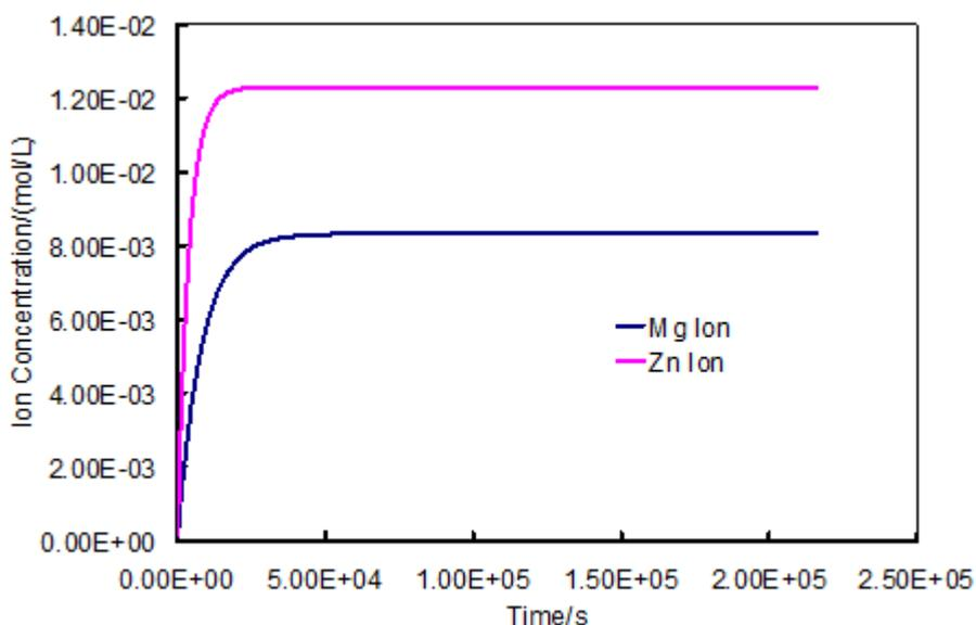
**Figure 3.** Ion concentration simulated curves of Mg and Zn mixed button battery
