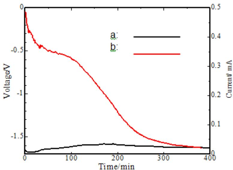
**Figure 5.** Electrochemical properties of Mg air battery (a: Open circuit potential; b: Loop current)
