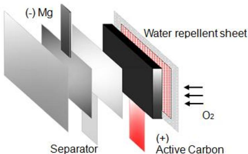
**Figure 1.** Schematic diagram of Mg air battery
