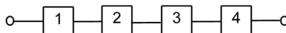
Figure 1. Block diagram of accumulator structural model: (1) accumulator EMF; (2) activation-ohmic element; (3) element, determining discharge polarization and (4) relaxation element
