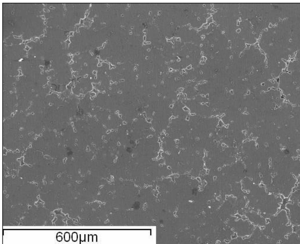
**Figure 2.** Matrix alloy microstructure constituted by Al-Mg solid solution rich in aluminum with dendritic microstructure.
