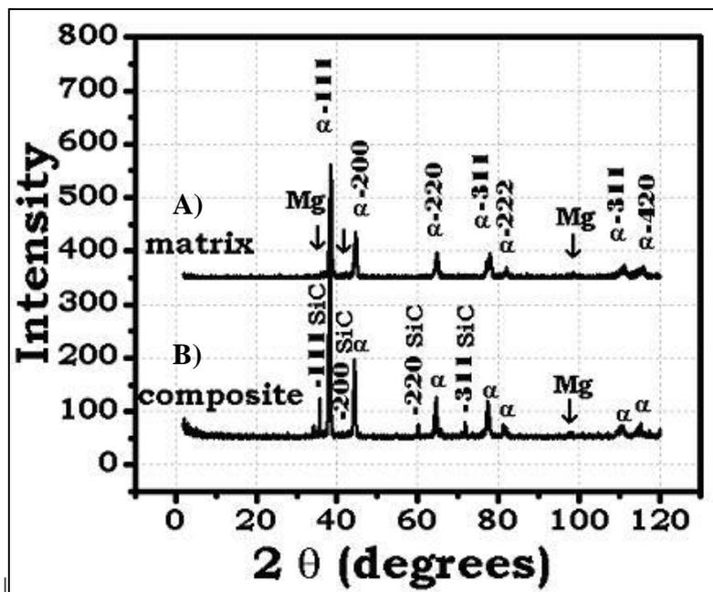
**Figure 1.** X-ray pattern showing the (A)  $\alpha$ -aluminum and magnesium particles on the matrix alloy and (B) SiC particles in the Al-MMC.
