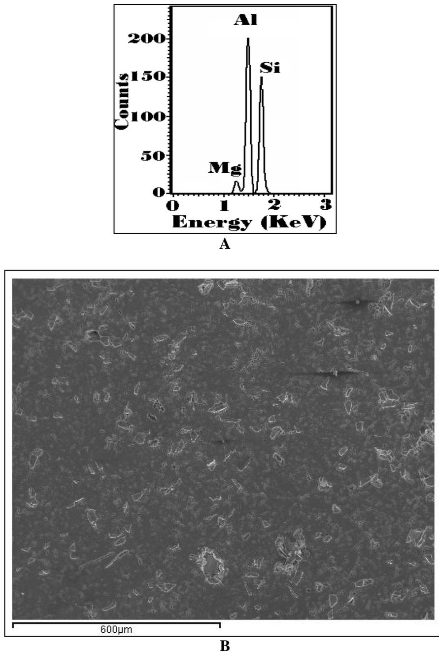
**Figure 3.** (A) Energy dispersive X-ray analyses spectrum from a spot of the solid solution interface with SiC particles. (B) Al-MMC microstructure of Al-Mg solid solution reinforcement with SiCp.
