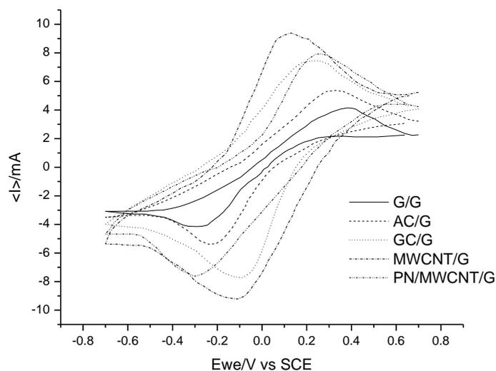
**Figure 4.** CV of modified electrode in 1M NaCl containing 10/10mM  $K_4Fe(CN)_6/K_3Fe(CN)_6$  at pH 7.
