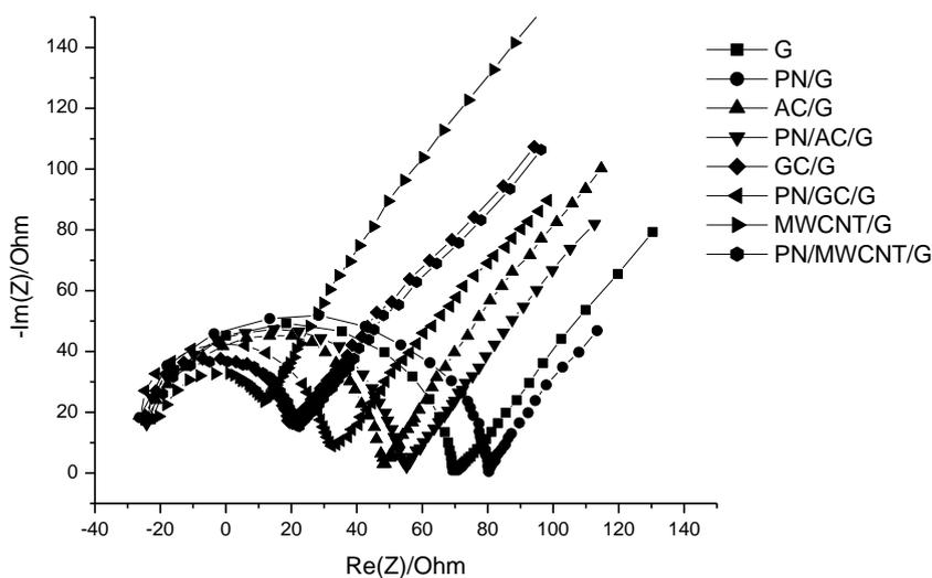
**Figure 2.** Nyquist plot of Carbon based working electrodes in 0.1M NaCl containing 10/10mM  $[\text{Fe}(\text{CN})_6]^{3-}/[\text{Fe}(\text{CN})_6]^{4-}$  ions
