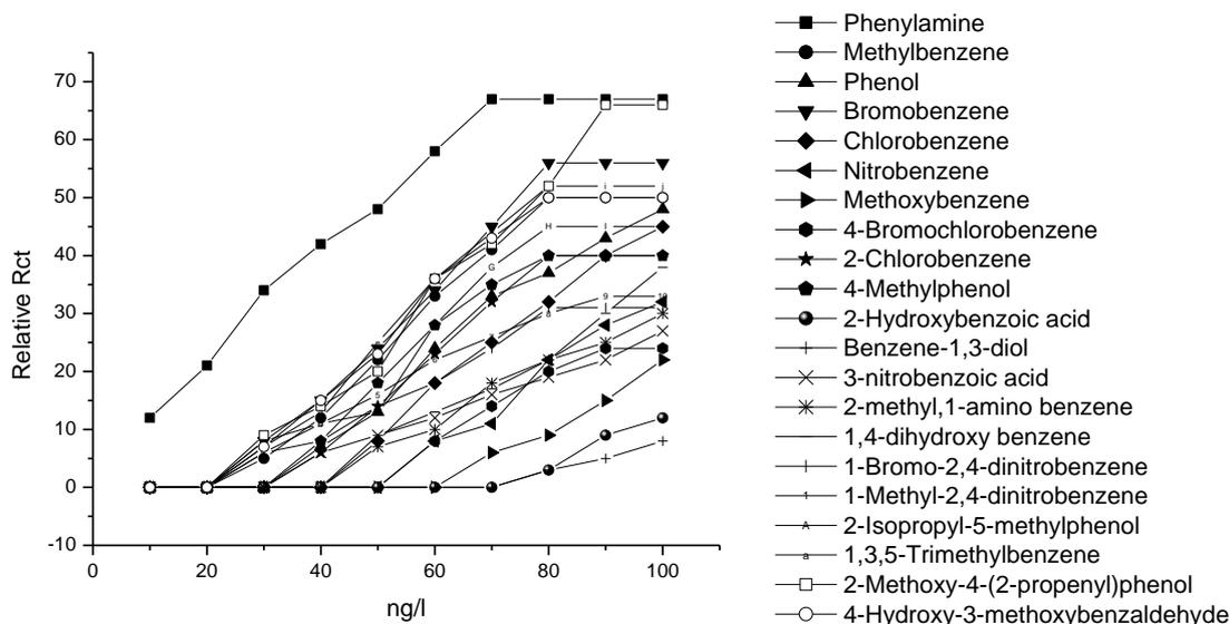
**Figure 5.** Calibration curves for the detection of benzene substituted derivatives by the standardized purine nucleobases immobilized MWCNT modified graphite electrode.
