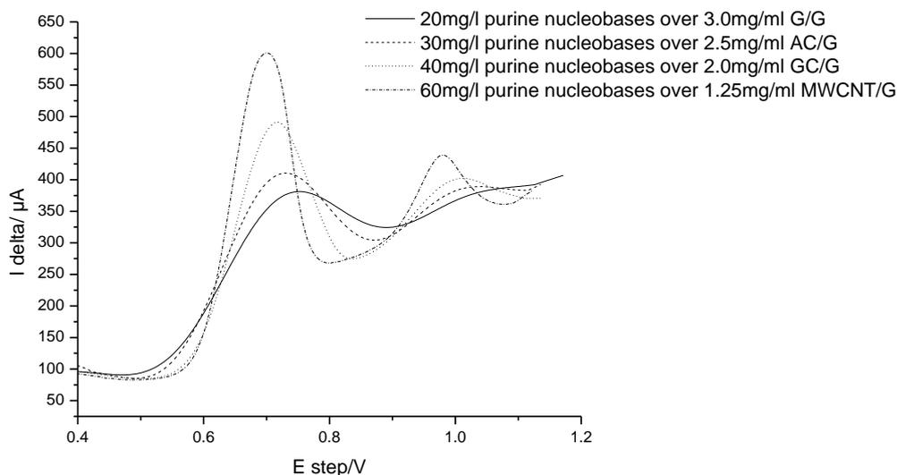
**Figure 1.** DPV response of the optimized carbon based electrode
