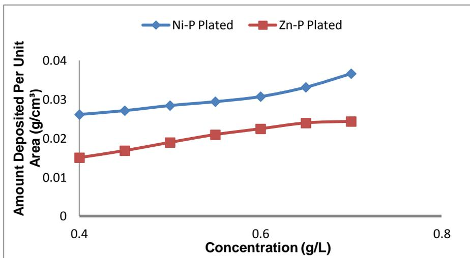
**Figure 2.** Amount deposited per unit area of Ni-P and Zn-P deposited on AISI 1045 steel at varied concentration
