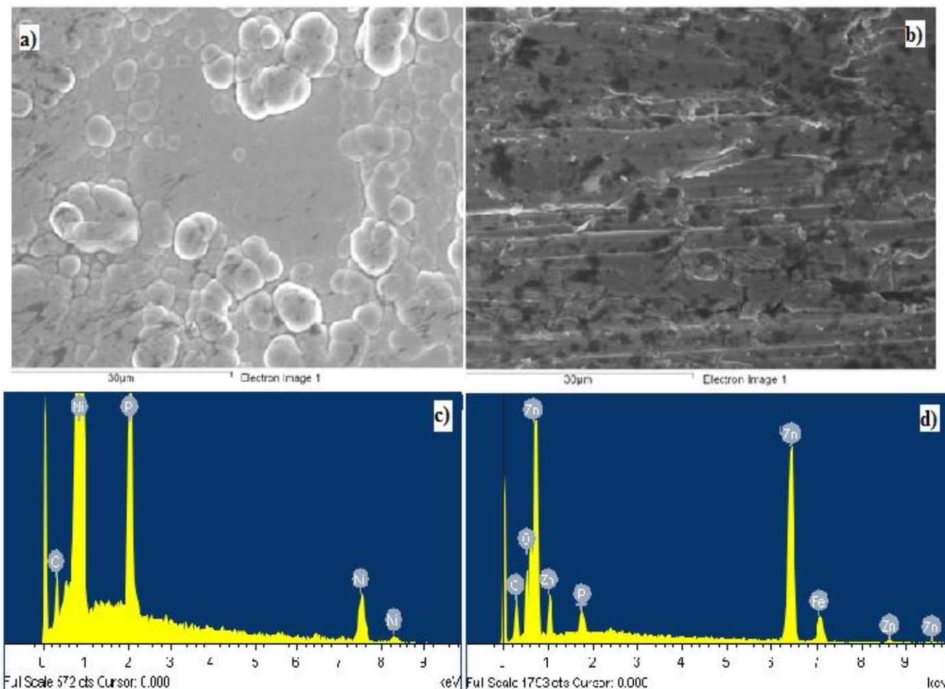
**Figure 8.** a) SEM for Ni-P b) SEM for Zn-P and EDS analysis c) for Ni-P EDS analysis for d) Zn-P at 0.55 g/L concentration, 80 °C temperature and 30 minutes deposition time
