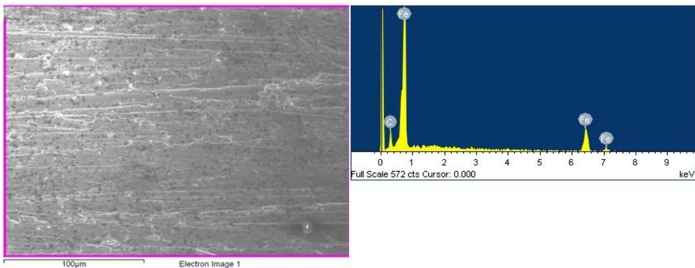
Figure 6. SEM Micrograph and EDS spectra for Unplated AISI 1045 Steel
