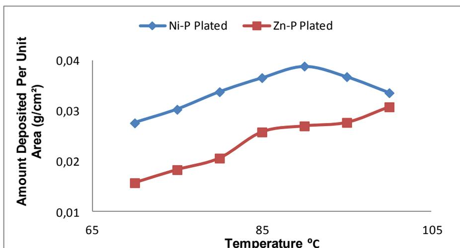
**Figure 1.** Amount deposited per unit area of Ni-P and Zn-P deposited on AISI 1045 steel at varied Temperature
