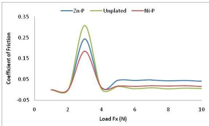
**Figure 5.** Plot of Coefficient of Friction Vs Load Fx (N) for electroless Ni-P and Zn-P deposition on AISI 1045 steel substrate
