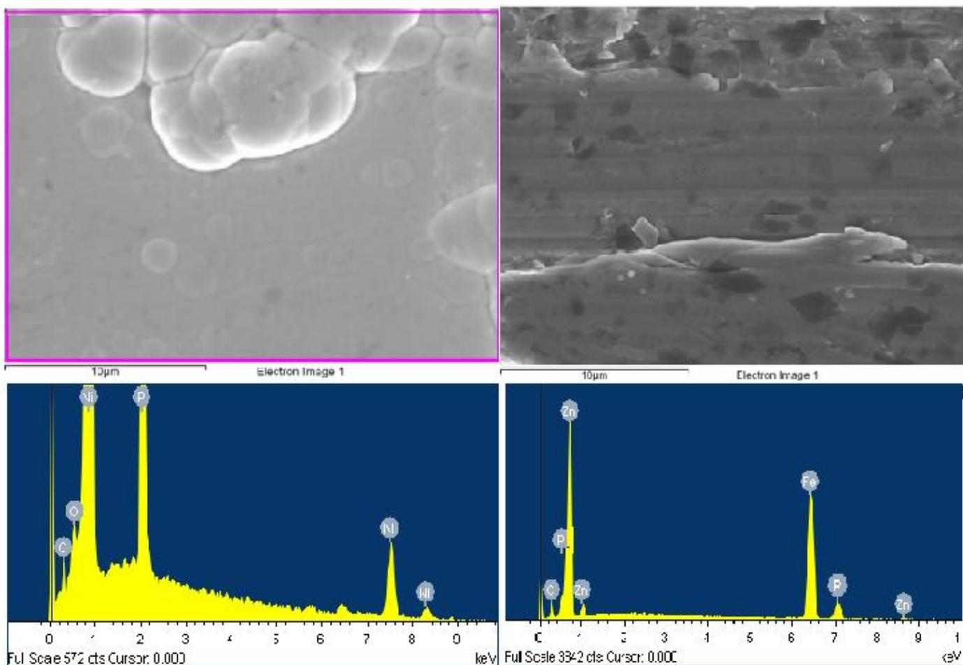
Figure 7. a) SEM for Ni-P b) SEM for Zn-P and EDS analysis c) for Ni-P EDS analysis at 0.55 g/L concentration, 80°C Temperature and 25 minutes
