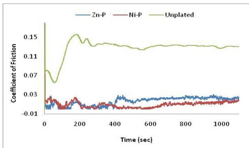
**Figure 4.** Plot of Coefficient of Friction Vs Time (sec) for electroless Ni-P and Zn-P deposition on AISI 1045 steel substrate
