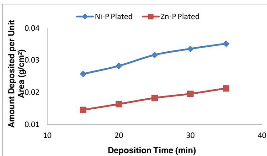
**Figure 3.** Amount deposited per unit area of Ni-P and Zn-P deposited on AISI 1045 steel at varied deposition time
