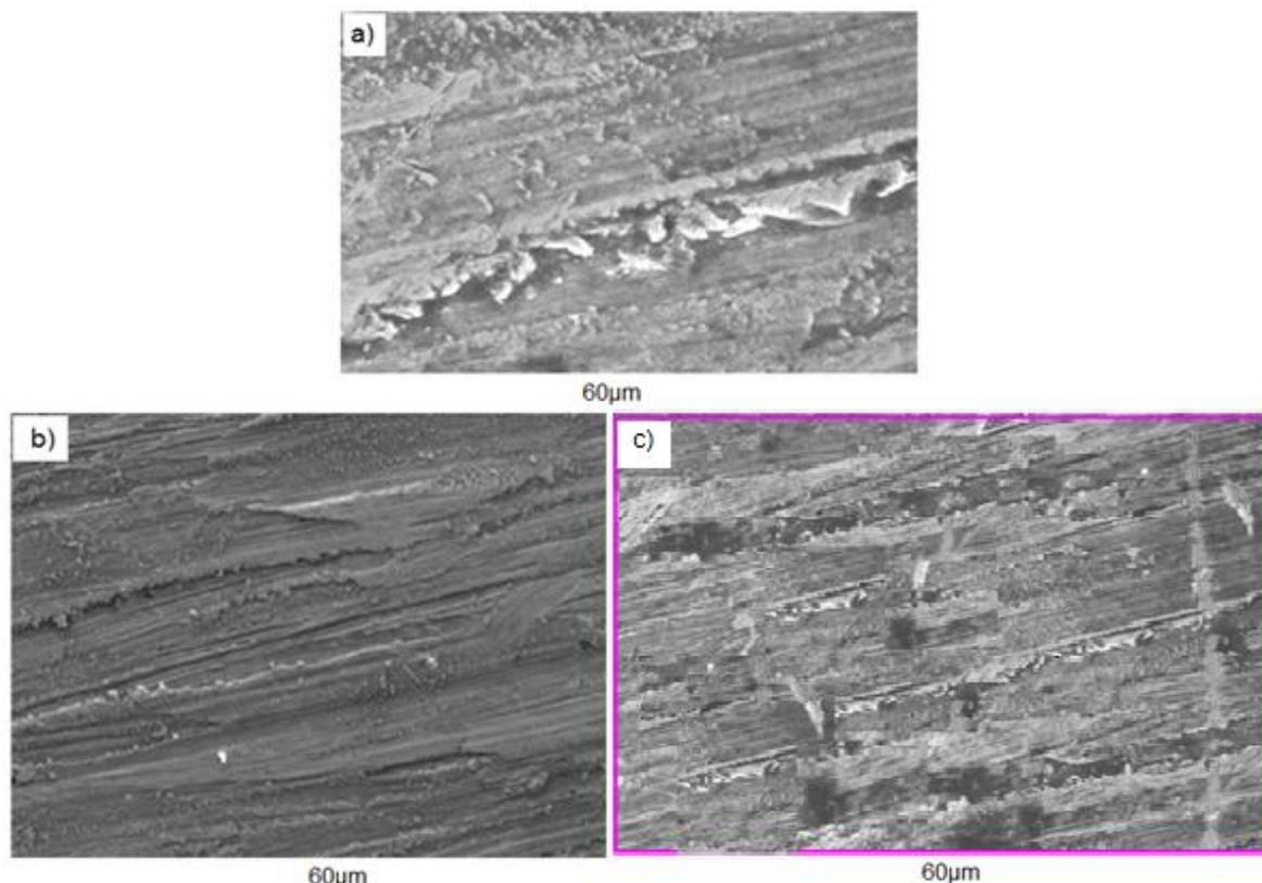
**Figure 9.** SEM of Worn Surfaces for a) Unplated b) Ni-P plated and Zn Plated AISI 1045 Mild Steel
