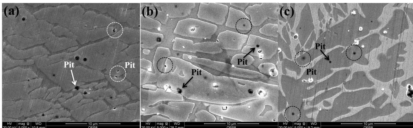
**Figure 5.** SEM morphologies of pits formed each specimens during the potentiodynamic test at 1250mV in 3.5% NaCl:(a) No.1, (b) No.2, (c) No.3
