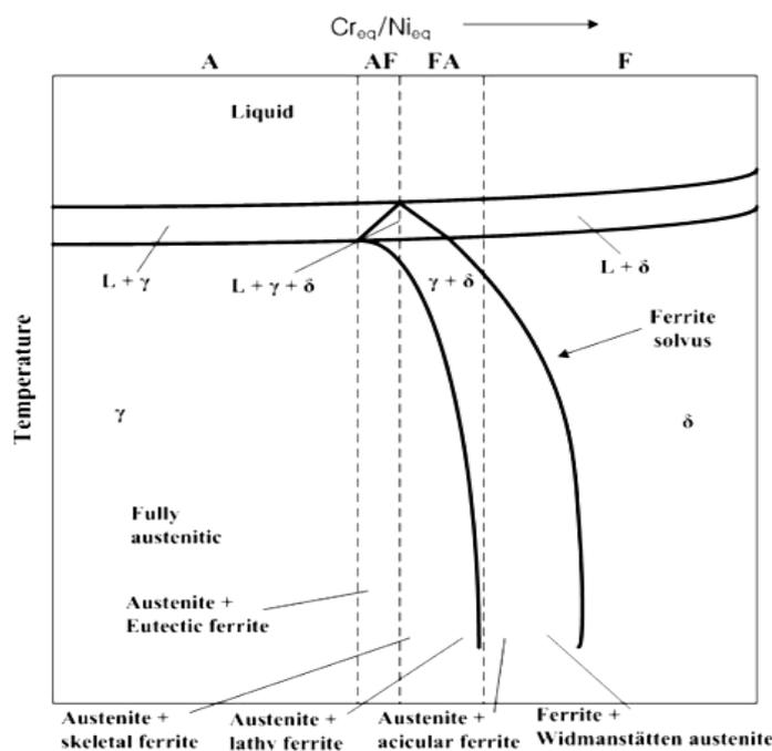
**Figure 3.** Pseudo-binary Fe-Cr-Ni phase diagram
