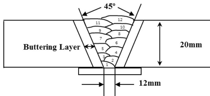
**Figure 1.** Schematic Diagrams of the weldment
