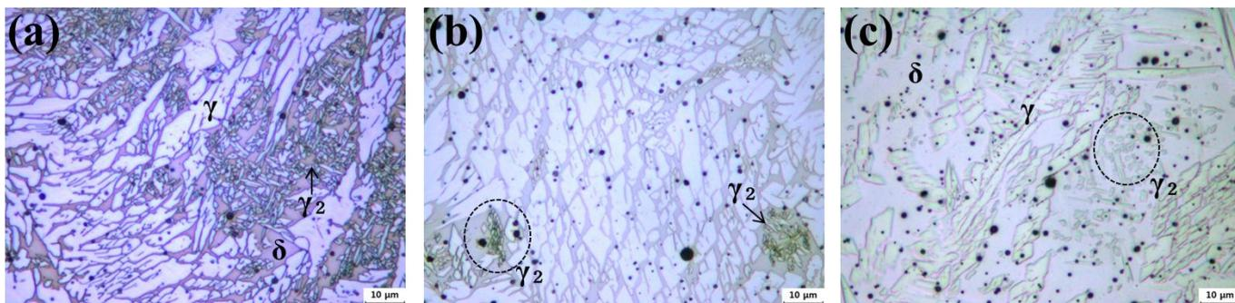
**Figure 2.** Microstructure of Weldments : (a) No.1, (b) No.2, (c) No.3
