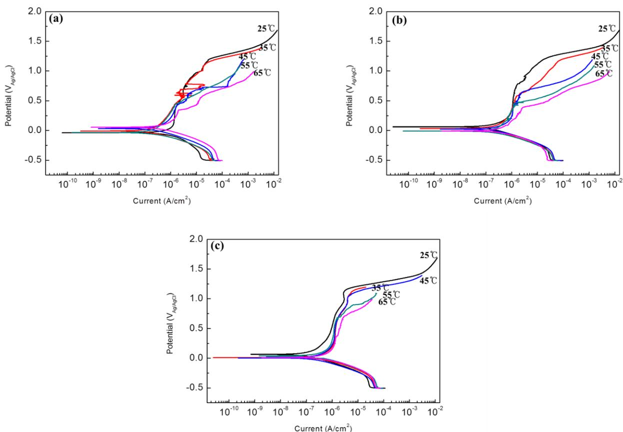
**Figure 8.** Polarization curve of each specimens in 25°C, 35°C, 45°C, 55°C, 65°C, 3.5% NaCl: (a) No.1 (b) No.2 (c) No.3
