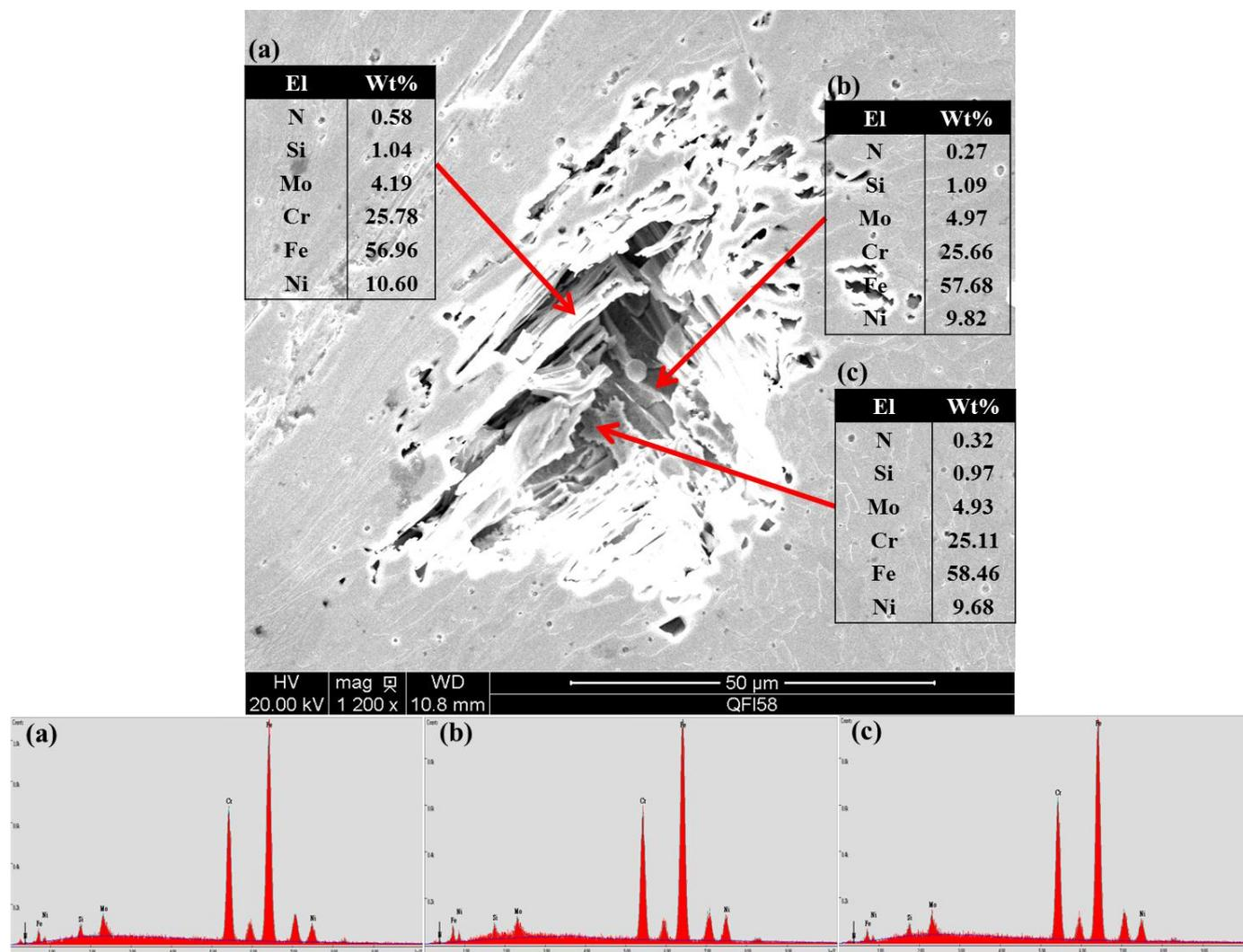
Figure 6. SEM & EDS measurements of  $\delta$ -ferrite formed inside the pit
