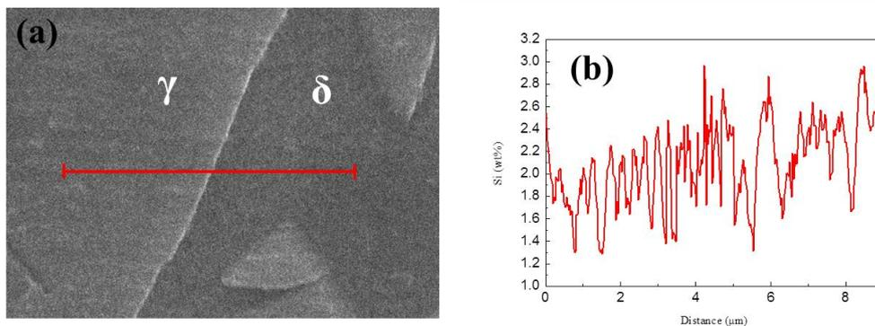
**Figure 7.** Mapping analysis of  $\gamma/\delta$ -ferrite grain boundary
