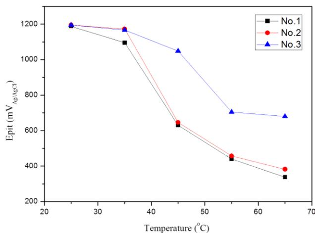
**Figure 9.** Pitting potential (E<sub>pit</sub>) against temperature in each specimens
