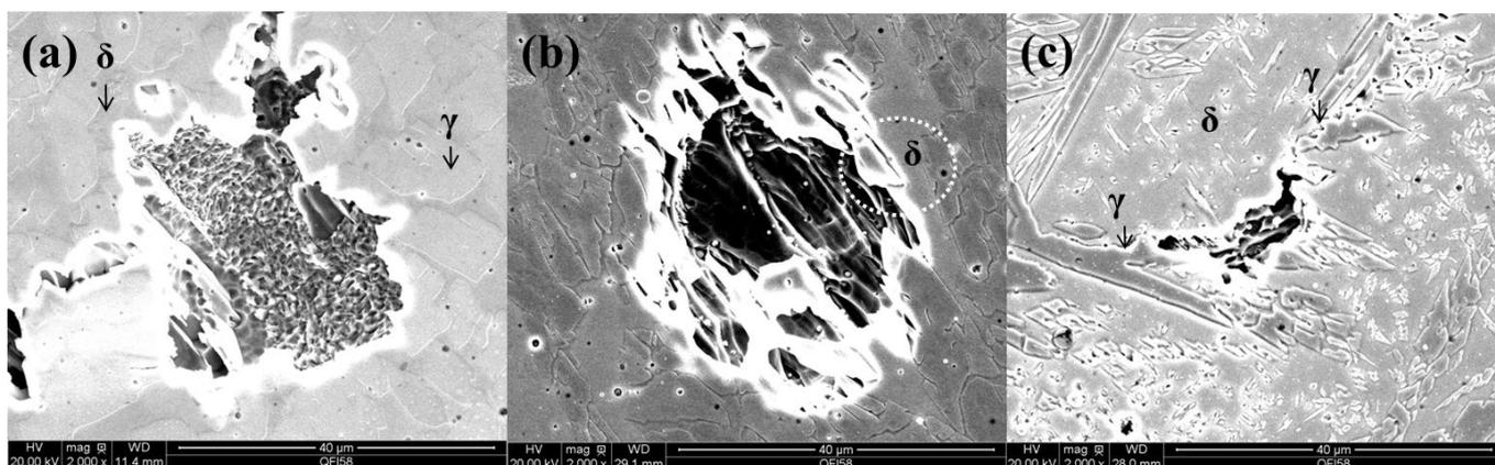
**Figure 4.** SEM morphologies of pits formed each specimens after CPT test in 6% FeCl<sub>3</sub> + 1% HCl solution:(a) No.1, (b) No.2, (c) No.3
