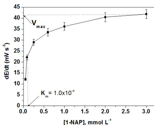
**Figure 5.** Initial reaction rates obtained with 1-NAP membrane sensor with several 1-NAP initial concentrations fitted to the Michaelis-Menten equation
