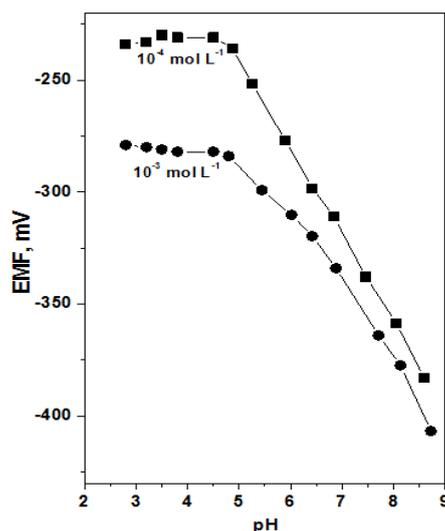
**Figure 4.** Influence of the solution pH on the response of the 1-NAP membrane based sensor
