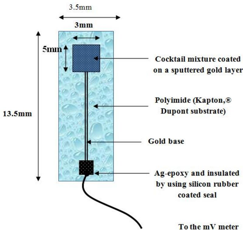
**Figure 1.** Planar-chip sensor
