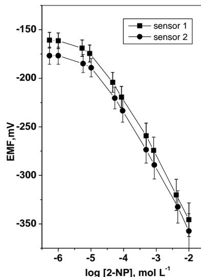
**Figure 3.** Response characteristics of 1-NAP substrate PVC membrane sensor in  $0.05 \text{ mol L}^{-1}$  acetate buffer of pH 4.7.
