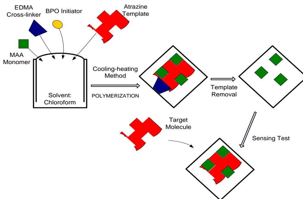
**Figure 1.** The process of preparing an atrazine molecularly imprinted polymer (MIP) and testing its sensing characteristics [23].
