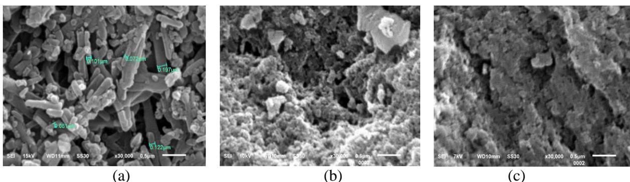
**Figure 2.** SEM images of (a) standard atrazine, (b) polymer before removing the atrazine template, and (c) the atrazine MIP after template removal.
