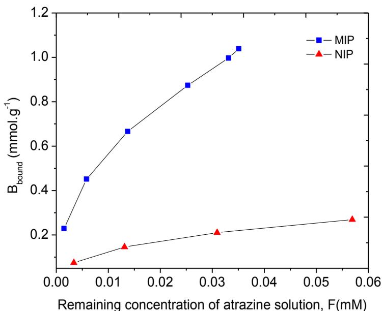
**Figure 8.** The relation between the number of bound atrazine molecules (targets) and the remaining concentration of atrazine solution for MIP and NIP.
