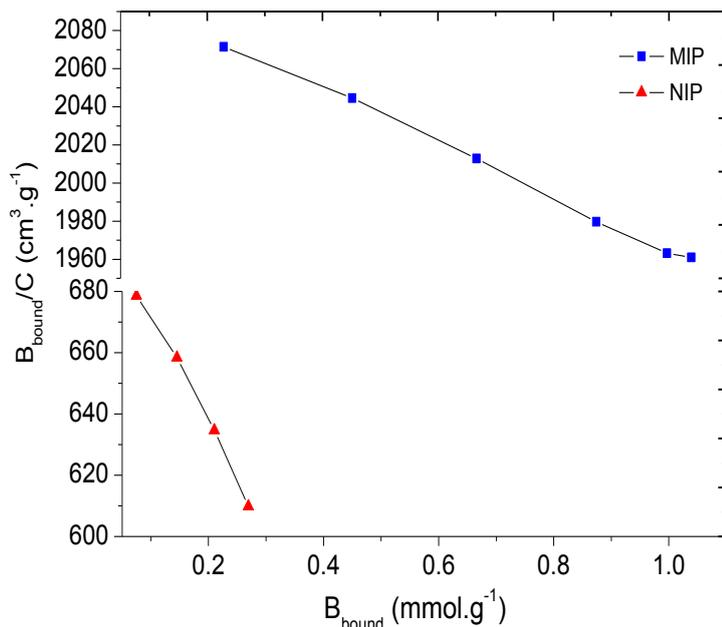
**Figure 7.** Scatchard plots of atrazine MIP and NIP for 1 mL of atrazine solution.
