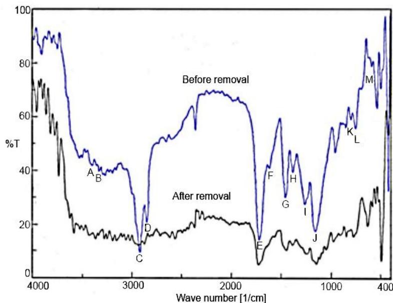
**Figure 4.** FTIR spectra of the polymer before removing the atrazine template and its atrazine MIP obtained after the template removal.
