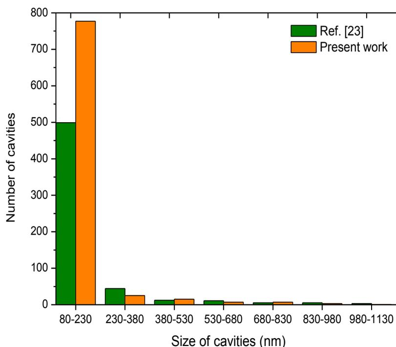
**Figure 3.** Cavity size distributions of atrazine MIP as reported in Ref. [23] due to the single washing process and in the present work that was produced with the repeated washing process.
