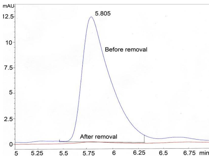
**Figure 5.** HPLC chromatograms of atrazine in the polymer before removing the atrazine template and in its atrazine MIP obtained after the template removal.
