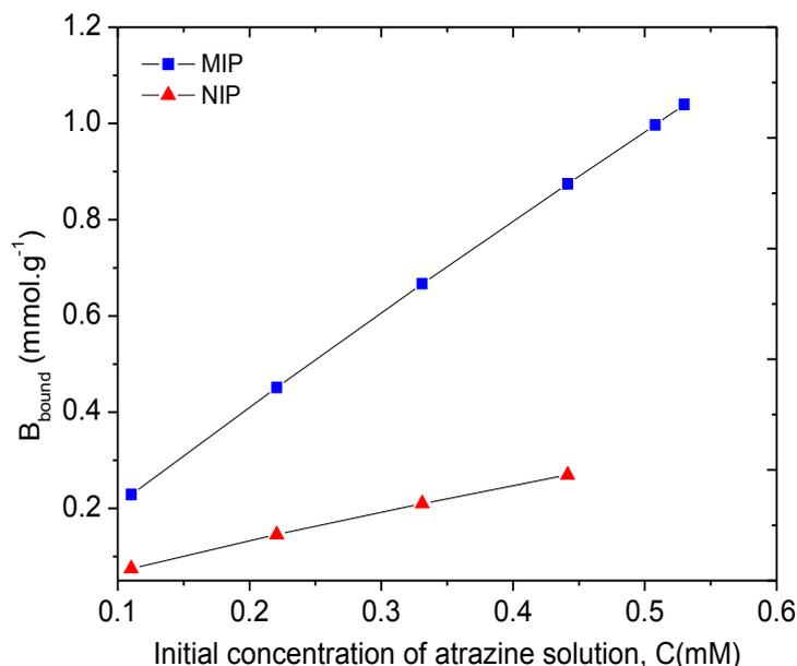
**Figure 6.** The relation between the number of bound atrazine molecules (targets) and initial concentration of atrazine solution for MIP and NIP.
