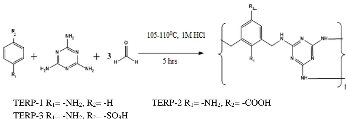
**Scheme 1.** Synthetic scheme of terpolymers
