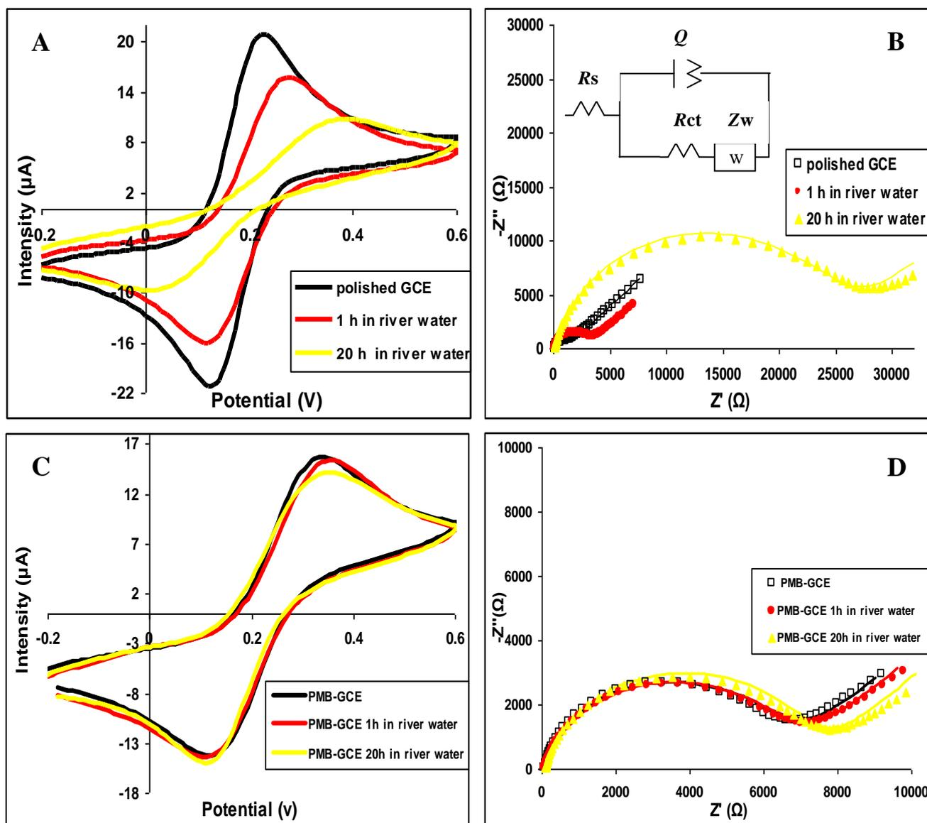
**Figure 4.** The characterization by CV and EIS of a bare-GCE [A, B] and PMB-GCE [C, D] after their immersion in river water during 1 h (red) and 24 h (yellow). For comparison it is presented the initial state (black). Nyquist plots: points are the experimental data and the lines are the curves obtained by fitting using the Randles equivalent circuit.
