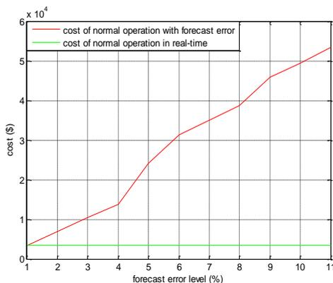
**Figure 8.** Cost of normal operation strategy under forecast error and perfect forecast case
