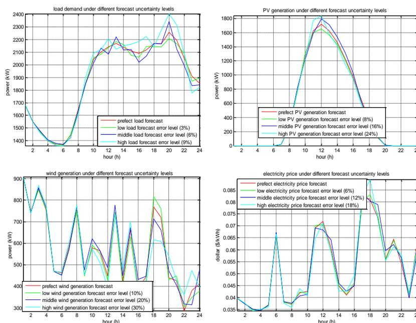
**Figure 6.** Load demand, wind generation, PV generation and electricity price data at different forecast error levels in day-ahead prediction
