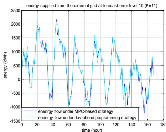
**Figure 10.** Energy supplied by external grid under MPC-based strategy and day-ahead programming strategy when forecast error level is 10 ( $K = 11$ )
