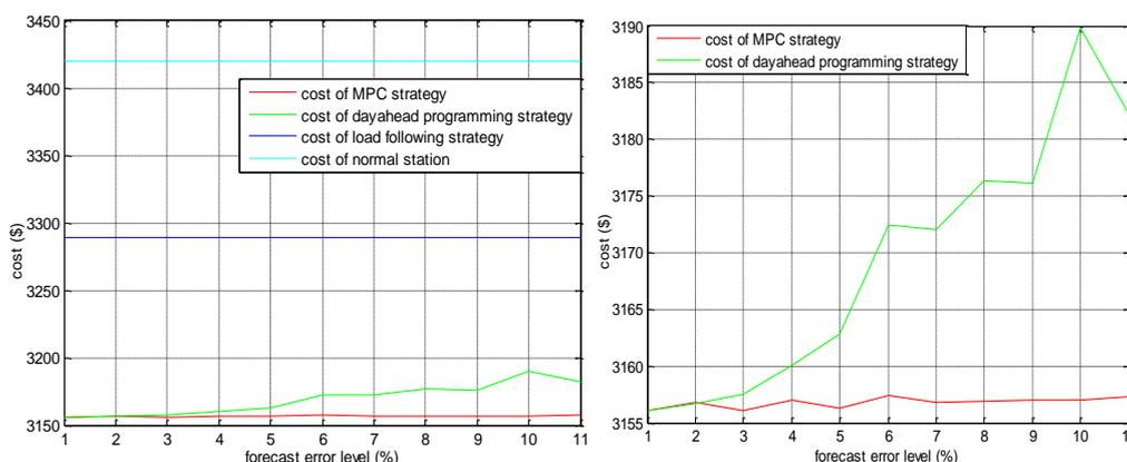
**Figure 7.** Microgrid operation cost of the four strategies under different forecast error levels
