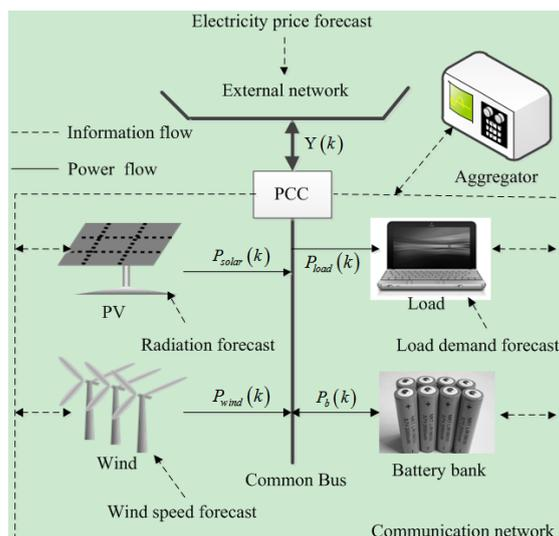
Figure 2. Simplified microgrid architecture
