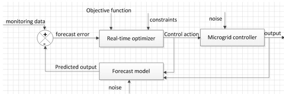
**Figure 3.** Scheme of basic MPC
