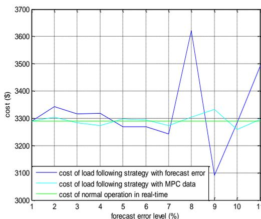
**Figure 9.** Cost of microgrid under load following strategy in three different cases (real-time data, day-ahead forecast data, and forecast data one period ahead)
