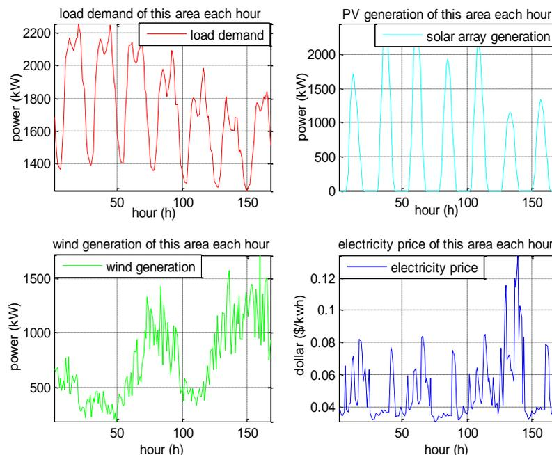
**Figure 4.** Actual data of Load demand, PV generation, wind generations and electricity price
