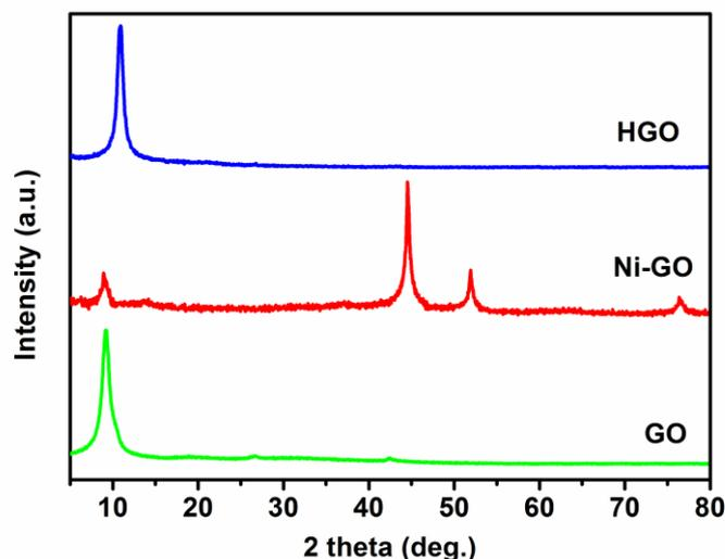
**Figure 1.** XRD pattern of the GO, Ni-GO and HGO.
