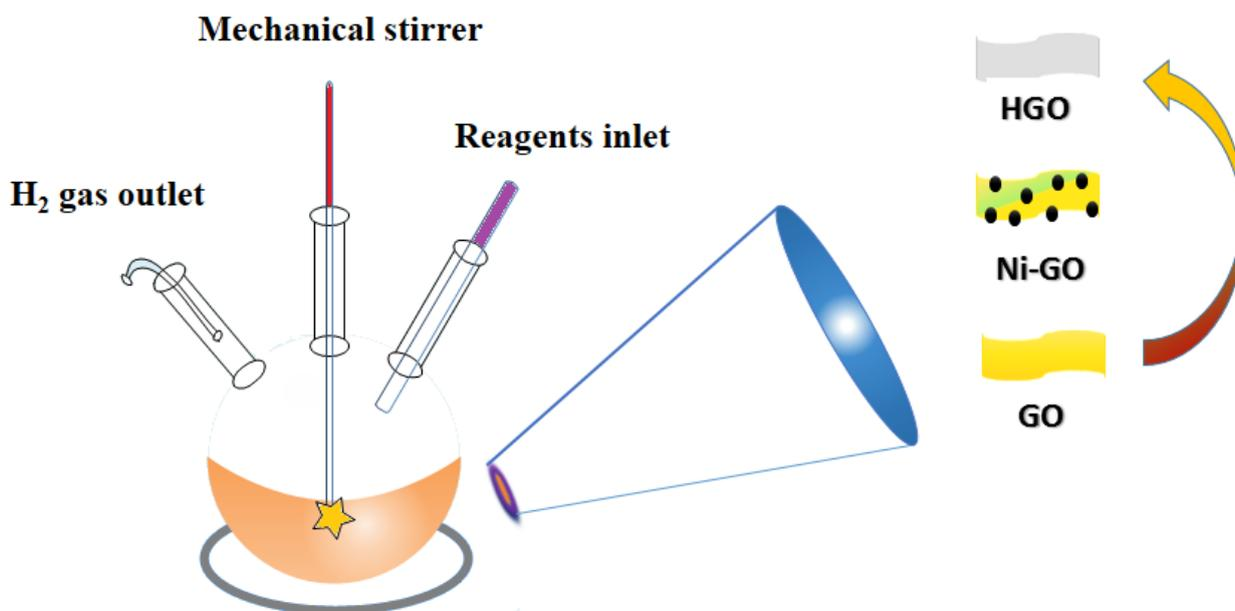
**Scheme 1.** Instrumental setup and representation of HGO synthesis.
