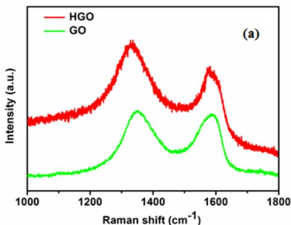
**Figure 4a.** Raman spectra of the GO and HGO.
