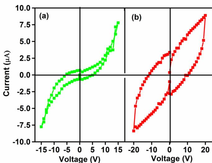
**Figure 7.** Characteristic I vs V curve of HGO in bias range of (a) sweeping voltage (-15 to +15V) and (b) sweeping voltage (-20 to +20V). The voltage is swept in the direction as follows: 0 V → 10 V → 0 V → -10 V → 0 V.
