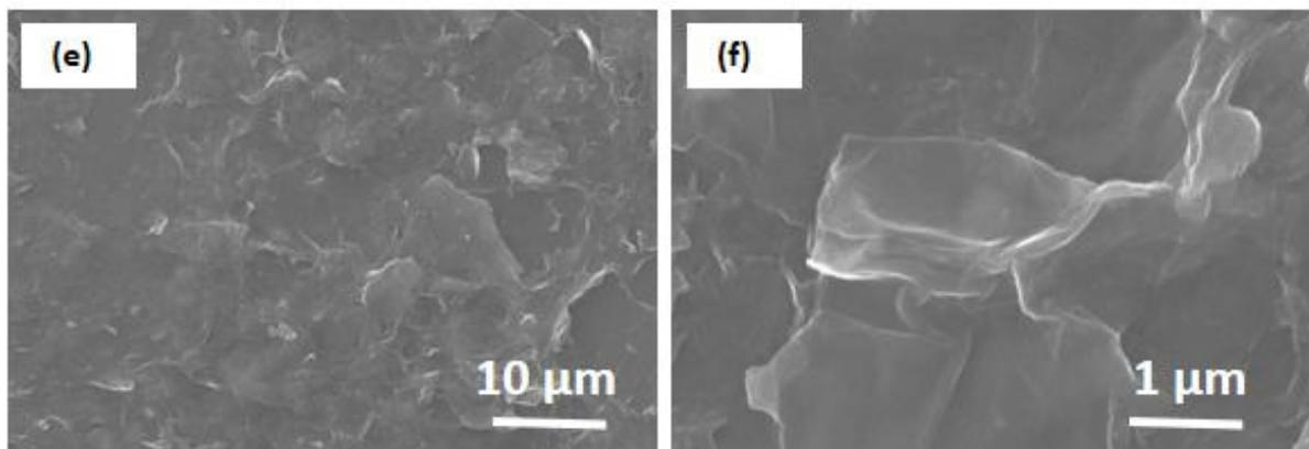
**Figure 5.** (e) and (f) SEM images of final product HGO in lower and higher magnification.
