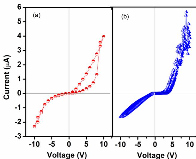
**Figure 8.** Characteristic I vs V curve of annealed sample of HGO in bias range of (-10 to +10V) with two different step sizes (a) with fast scan rate (1V/s step size) (b) with slow scan rate (0.1 V/s step size). The voltage is swept in the direction as follows: 0 V  $\rightarrow$  10 V  $\rightarrow$  0 V  $\rightarrow$  -10 V  $\rightarrow$  0 V.
