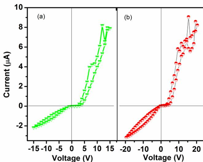
**Figure 9.** Characteristic I vs V curve of annealed sample of HGO in bias range of (a) sweeping voltage (-15 to +15V) and (b) sweeping voltage (-20 to +20V) with scan rate of (1V/s step size). The voltage is swept in the direction as follows: 0 V → 10 V → 0 V → -10 V → 0 V.
