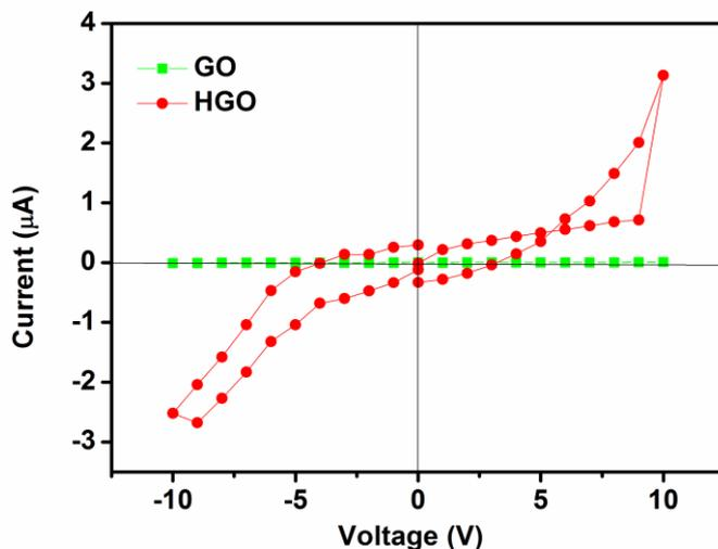
**Figure 6.** Characteristic I vs V curve of GO and HGO in bias range of (-10 to +10V). The voltage is swept in the direction as follows: 0 V → 10 V → 0 V → -10 V → 0 V.
