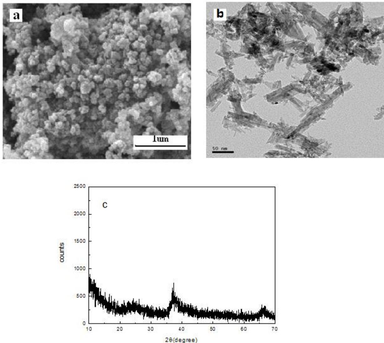
**Figure 1.** SEM image(a), TEM image(b) and XRD pattern(c) of the as-prepared  $\text{MnO}_2$
