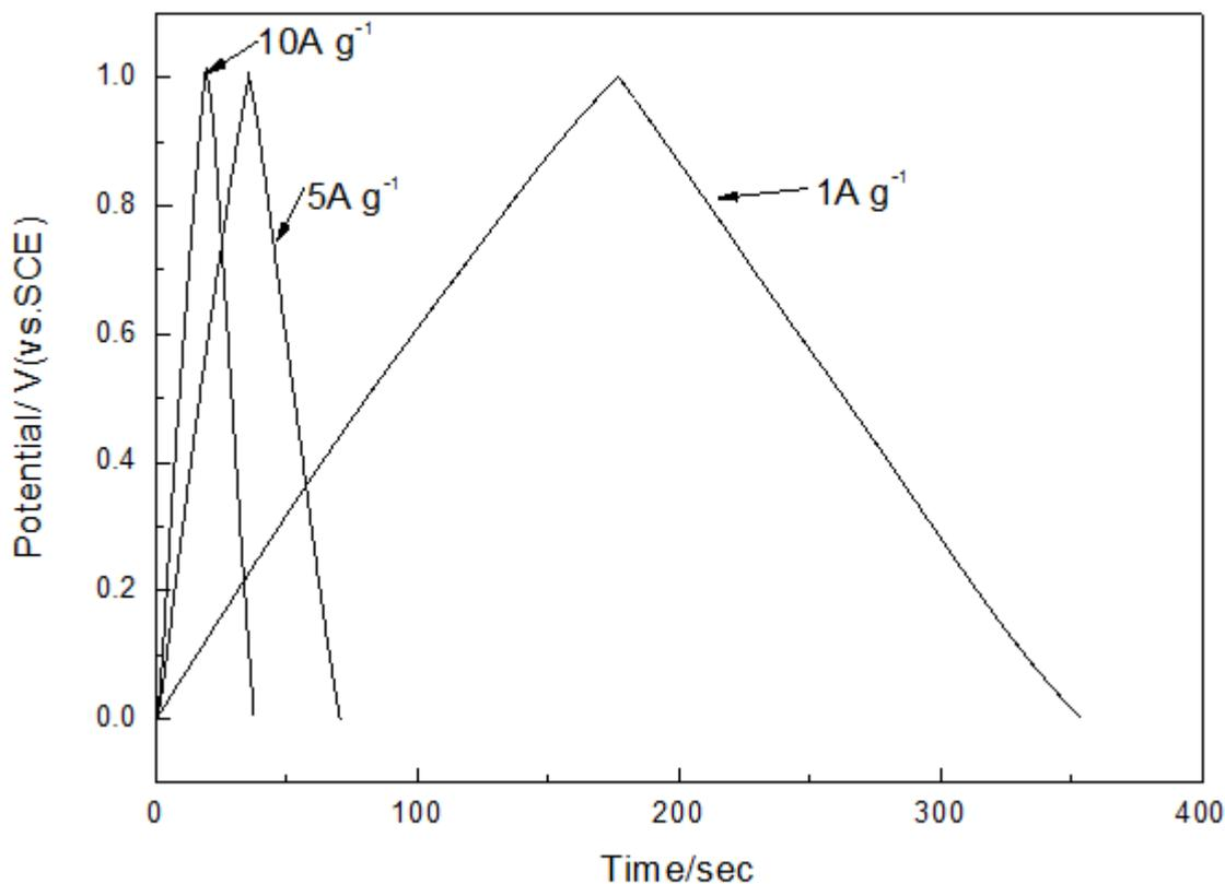
**Figure 8.** Charge/discharge curves of the electrode J5 measured at different current densities in 1M Na<sub>2</sub>SO<sub>4</sub> between 0 and 1.0V vs. SCE.
