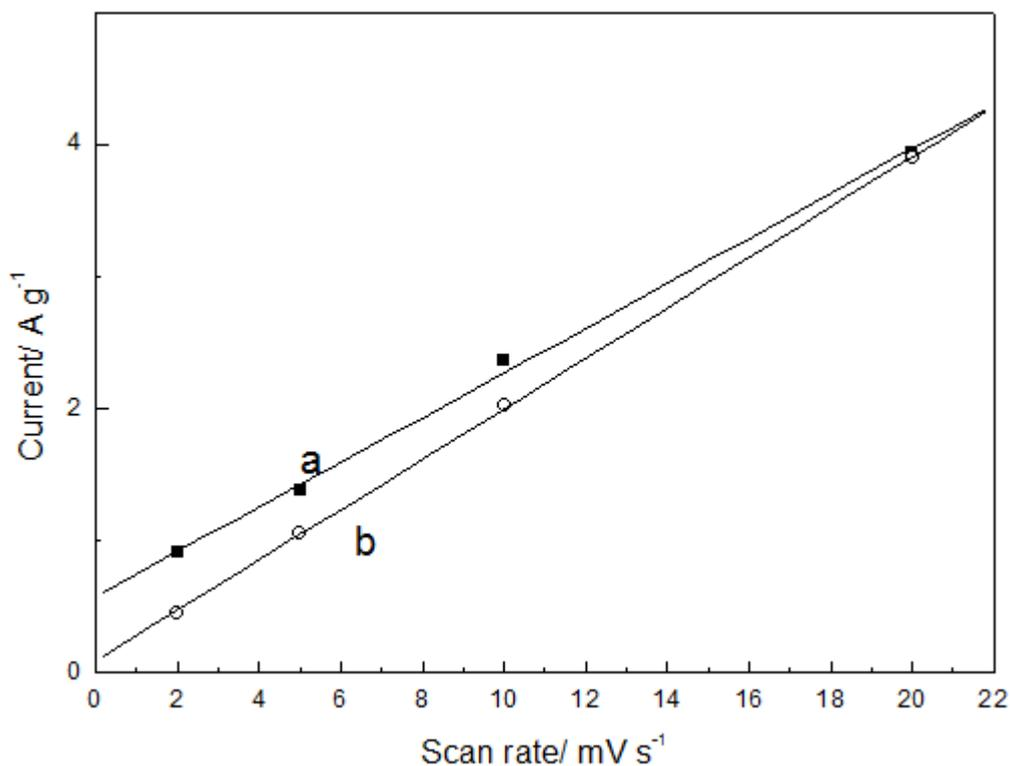
**Figure 4.** Plots of cathodic current change of the electrode J5(a) and J25(b) vs. scan rates. Currents were measured at the middle of the plateau at 0.5V/ Ref.
