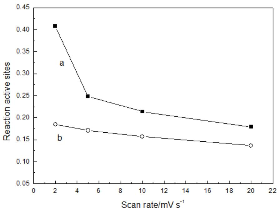
**Figure 6.** Reaction active sites of the as-prepared MnO<sub>2</sub> in the electrode J5(a) and J25 (b) vs. scan rates
