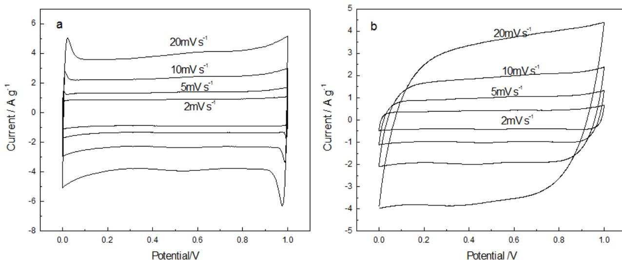
**Figure 3.** Cyclic voltammogram curves of the Electrode J5(a) and J25(b) measured at various scan rates in 1M Na<sub>2</sub>SO<sub>4</sub> solution.
