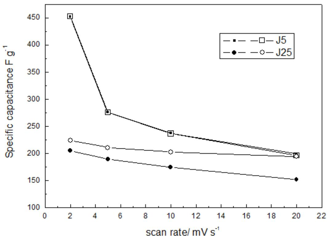
**Figure 5.** Specific capacitance of the electrode J5 and J25 as a function of scan rate. Filled symbols are calculated using equation (1) and open one using equation (2).
