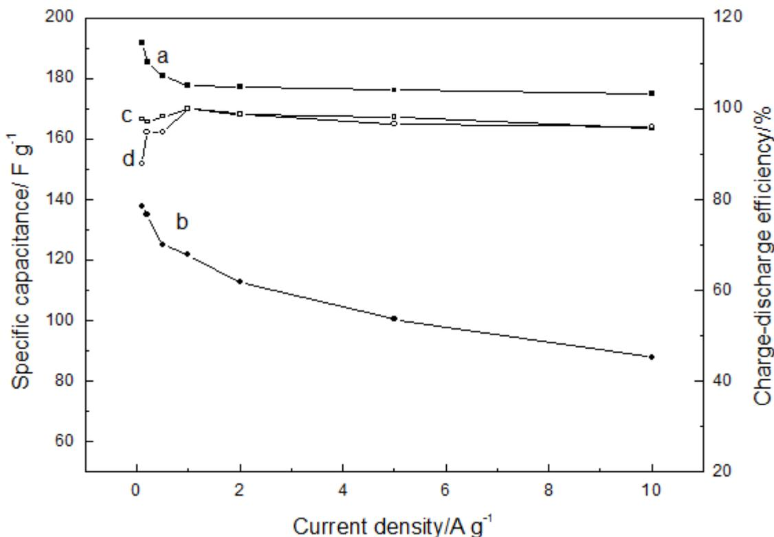
**Figure 9.** Dependence of specific capacitance (a,b) and charge-discharge efficiency(c,d) on current density of charge-discharge cycling of the electrode J5(a,c) and J25(b,d) in 1M  $Na_2SO_4$  between 0 and 1.0 vs. SCE)
