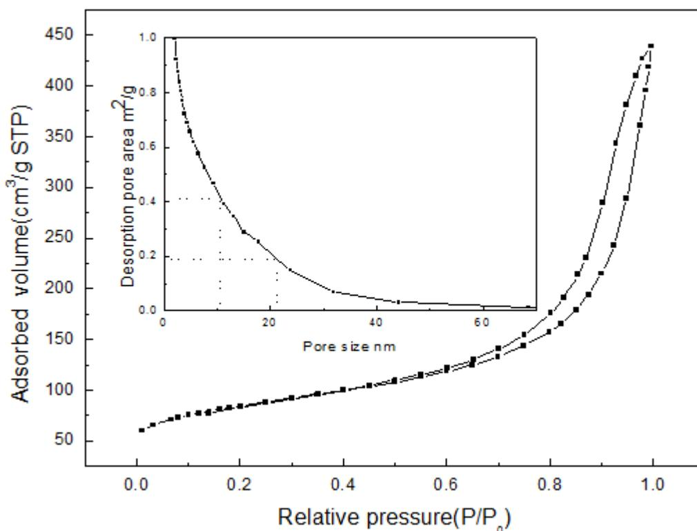
**Figure 2.** Nitrogen adsorption-desorption isotherms of the as-prepared  $\text{MnO}_2$ . The inset shows relative pore area distributions.
