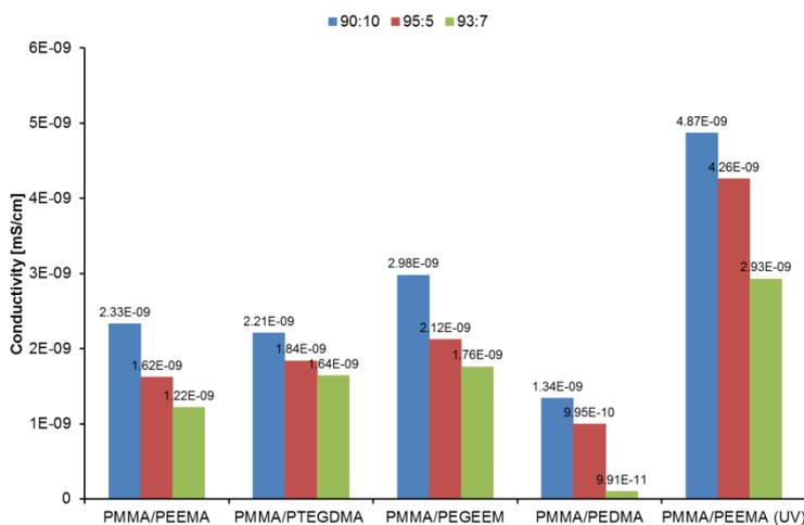
Figure 6. Conductivities of pure polymers
