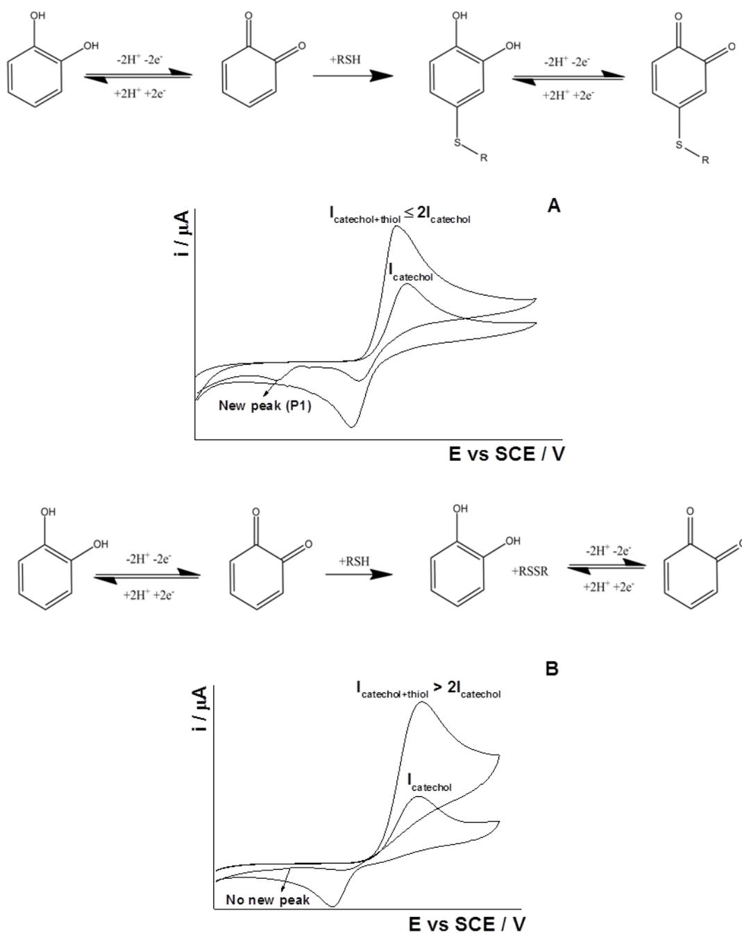
**Figure 1.** Resulting voltammograms of a solution containing catechol ( $I_{\text{catechol}}$ ) and thiol ( $I_{\text{catechol+thiol}}$ ) via: (A) 1,4 –Michael addition and (B) Electrocatalytic reaction.
