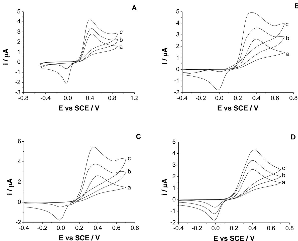
**Figure 3.** Cyclic voltammetric responses for  $100 \mu\text{M}$  catechol in PBS (pH = 7.5) in the absence (a) and presence of glutathione (A), homocysteine (B), cysteine (C) and ascorbic acid (D) using nanocarbon paste electrode. Different concentrations were added (b) 40 and (c)  $100 \mu\text{M}$ .  $v = 100 \text{ mVs}^{-1}$ .
