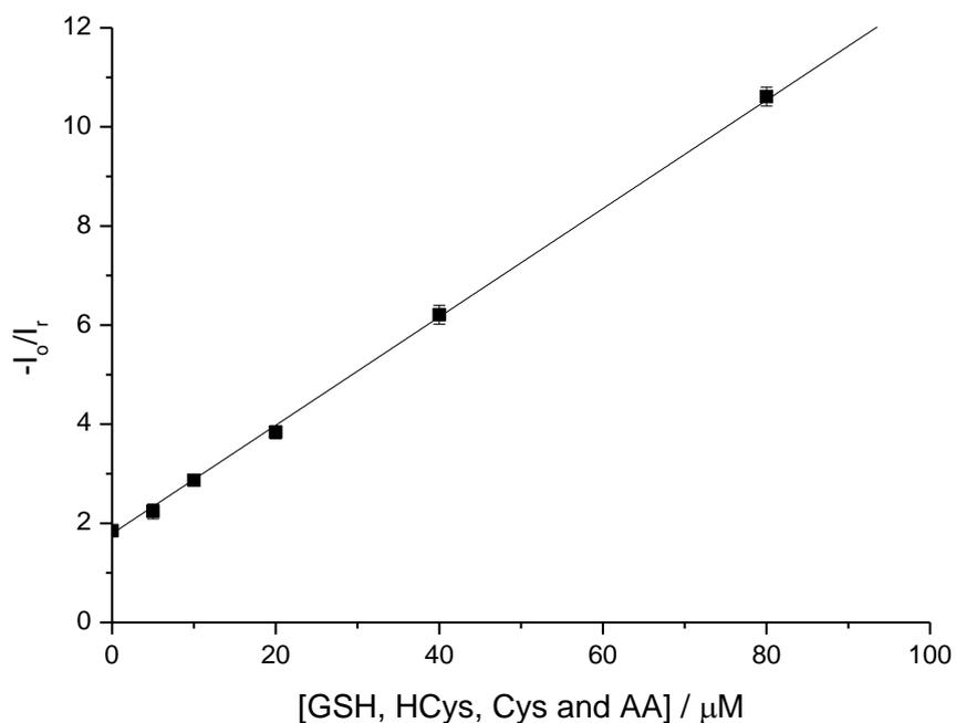
**Figure 9.** Calibration curve for total antioxidants using nanocarbon-catechol paste electrode.
