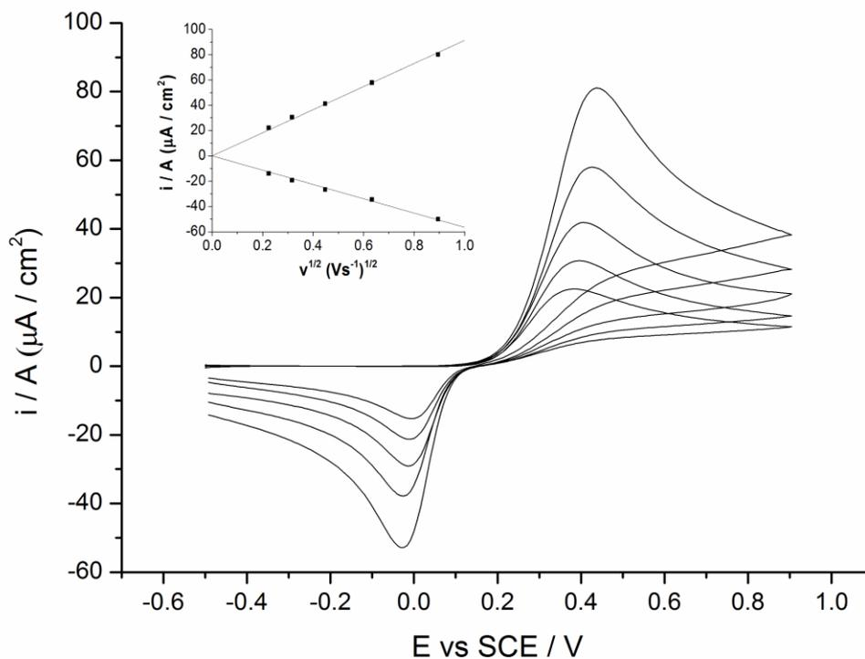
**Figure 2.** Cyclic voltammetric responses for 100 μM catechol in PBS (pH = 7.5) at different scan rate (from 50 to 800 mVs<sup>-1</sup>) at nanocarbon electrode. Inset: plot of peak current against square root of scan rate. The current was normalized by electrode area.  $E^0 = +0.17\text{V}$  and  $D = 7.0 \times 10^{-6} \text{ cm}^2/\text{s}$
