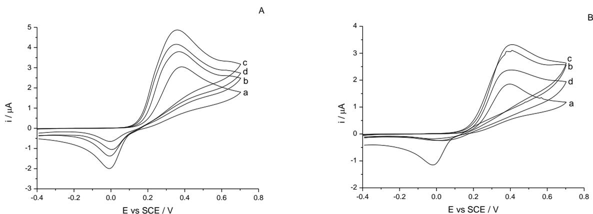
**Figure 8.** Cyclic voltammetric responses in PBS (pH = 7.5) in the absence (a) and presence of 40  $\mu\text{M}$  “mix” (A) and 80  $\mu\text{M}$  “mix” (B) using 0.3% catechol dissolved in nanocarbon paste electrode. Curves b, c and d: “mix” A, C and I, respectively.
