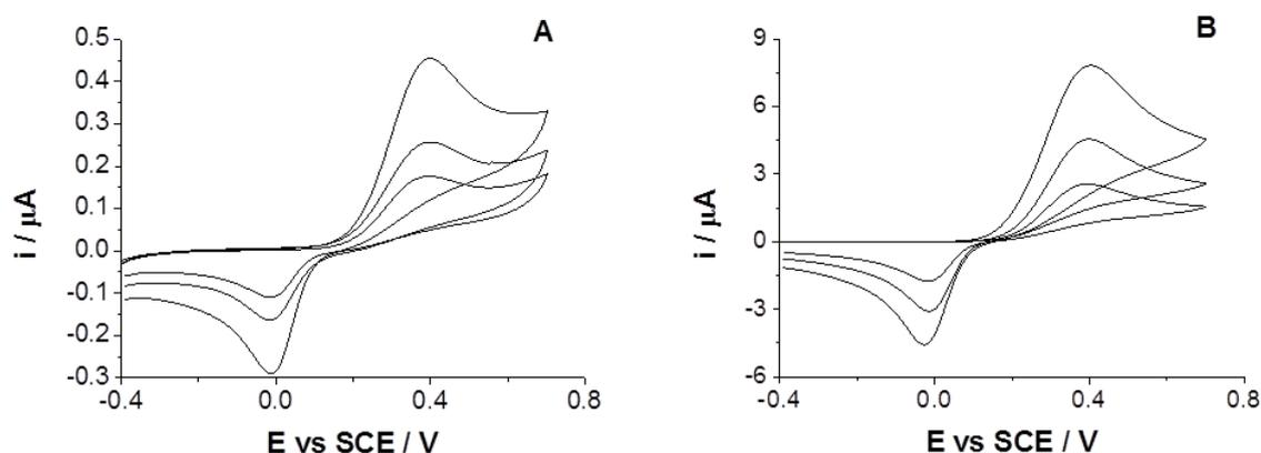
**Figure 6.** Cyclic voltammetric responses for 0.05% (A) and 0.3% (B) catechol dissolved in the nanocarbon paste in PBS (pH = 7.5) at  $100\text{mVs}^{-1}$ . Three scans with the same paste.
