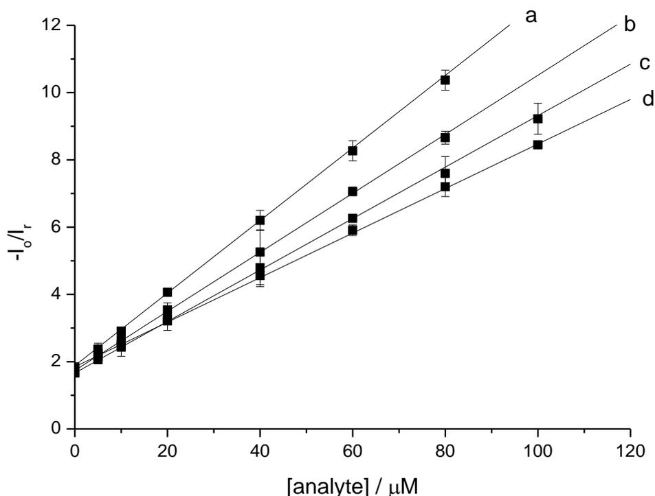
**Figure 7.** Calibration curve for (a) cysteine, (b) homocysteine, (c) glutathione and (d) ascorbic acid using nanocarbon-catechol paste electrode.
