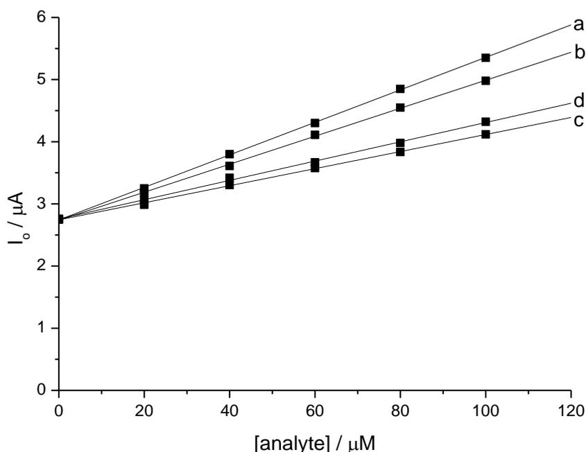
**Figure 4.** Calibration curve for (a) cysteine, (b) homocysteine, (c) glutathione and (d) ascorbic acid using a nanocarbon paste electrode and catechol in solution. [Catechol] =  $100\mu\text{M}$ .
