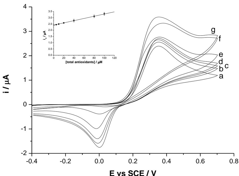
**Figure 5.** Cyclic voltammetric responses for  $100\mu\text{M}$  catechol in PBS ( $\text{pH} = 7.5$ ) in the absence (a) and presence of total antioxidants at different concentrations (b)  $5\mu\text{M}$ , (c)  $10\mu\text{M}$ , (d)  $20\mu\text{M}$ , (e)  $40\mu\text{M}$ , (f)  $80\mu\text{M}$  and (g)  $100\mu\text{M}$  using nanocarbon paste electrode.  $v = 100\text{mVs}^{-1}$ . Inset: analytical curve.
