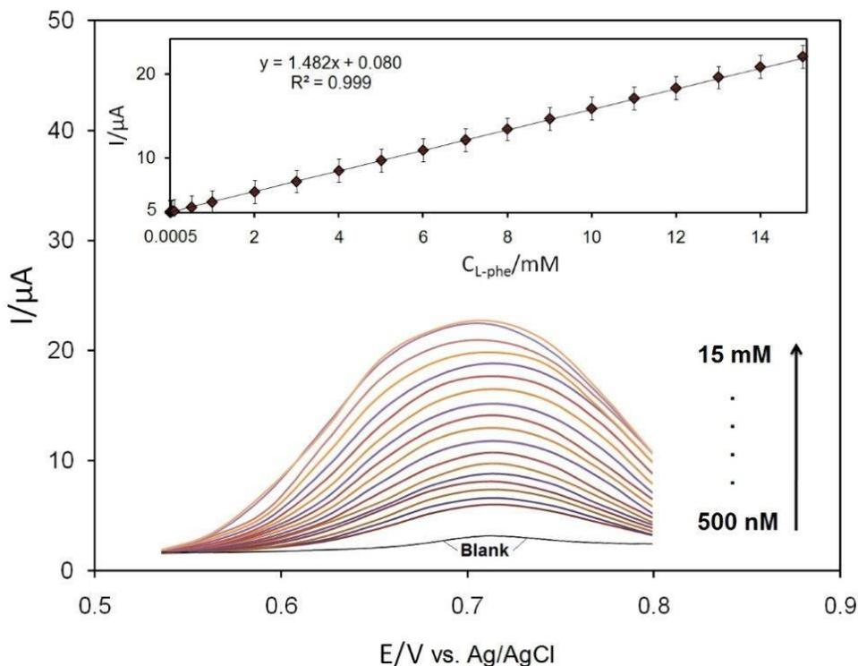
**Figure 4.** Typical DPV plots of the biosensor in Gly/KOH/KCl buffer solution (pH 10.5) containing different concentrations of L-phe (500 nM-15 mM). Inset represents a linear response attributed to L-phe increasing in range of 0.0005 mM to 15 mM. Initial working volume: 12 ml; supporting electrode: 100 mM Gly/KOH/KCl buffer pH 10.5 containing 2.5 mM NAD<sup>+</sup>.
