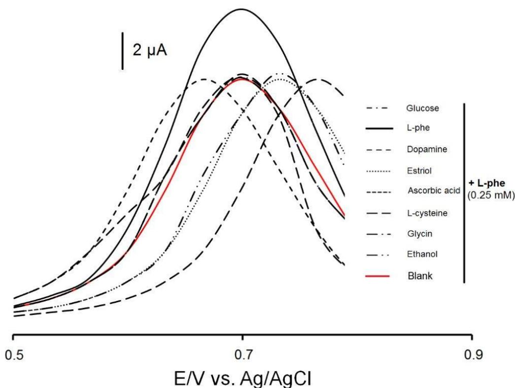
**Figure 5.** Typical DP voltammograms of the enzyme electrode in presence of 1 mM glucose, 1 mM estriol, 1 mM ethanol, 1 mM glycin, 1 mM L-cysteine, 1 mM ascorbic acid and 1 mM dopamine (lower DPV plots), and 1 mM L-phe (upper DPV plot). Initial working volume: 12 ml; supporting electrode: 100 mM Gly/KOH/KCl buffer pH 10.5 containing 2.5 mM  $\text{NAD}^+$  and 0.25 mM L-phe.
