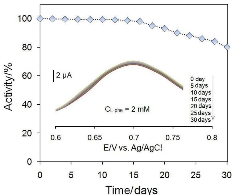
**Figure 6.** Control chart constructed for enzyme-functionalized electrode after 30 days in 2 mM L-phe concentration. Initial working volume: 12 ml; supporting electrode: 100 mM Gly/KOH/KCl buffer pH 10.5 containing 2.5 mM NAD<sup>+</sup>.
