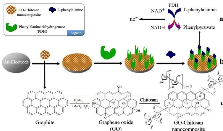
**Figure 1.** Schematic representation: (A) The preparation of the GO-Chitosan-PDH. (B) The fabrication processes of the biosensor. (C) Reaction mechanism of L-phe in presence of PDH.
