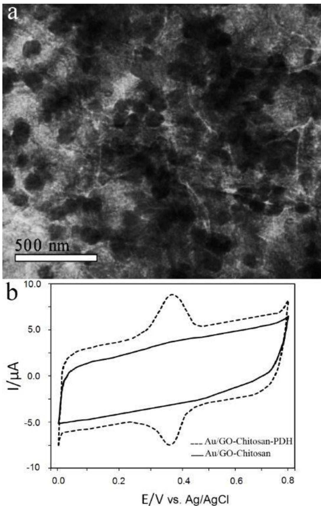
**Figure 2.** (A) TEM image of GO-chitosan composite. (B) Cyclic voltammograms of AuE/chitosan-GO (solid) and AuE/chitosan-GO-PDH (dashed) in 0.1M Gly/KOH/KCl buffer solution (pH 10.5) at scan rate of  $25 \text{ mV}\cdot\text{s}^{-1}$ .
