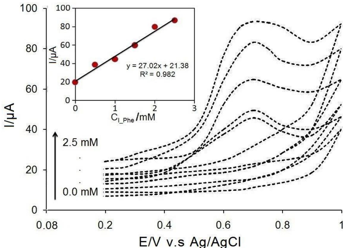
**Figure 3.** Cyclic voltammograms of the enzyme electrode at scan rate of 25 mV/s containing 2.5 mM  $\text{NAD}^+$ , without L-phe, 0.5, 1, 2, 2.5 mM, of L-phe, respectively. Inset represents a linear response related to L-phe increasing in range of 0.5 to 2.5mM.
