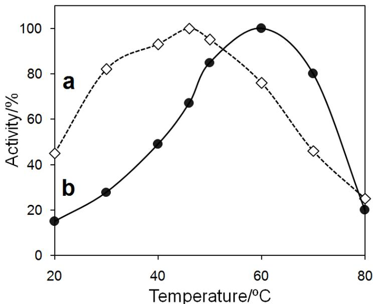
**Figure 3.** Effect of temperature on the catalytic activity of the suspended PDH (a) and the amperometric response of the enzyme electrode (b) toward 2.5mM L-phe. Applied potential: 1.0 V; stirring rate: 200 rpm; initial working volume: 12ml; supporting electrode: 100mM Gly/KOH/KCl buffer pH 10.5 containing 2.5mM NAD<sup>+</sup>.
