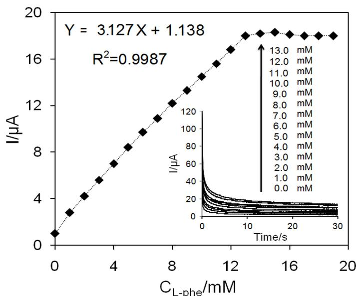
**Figure 7.** Chronoamperograms of the enzyme electrode at the constant voltage of 200mV. Inset: currents rises as L-phe concentration increases by 0-10mM of L-phe, respectively. Initial working volume: 12ml; supporting electrode: 100mM Gly/KOH/KCl buffer pH 10.5 containing 2.5mM  $\text{NAD}^+$ .
