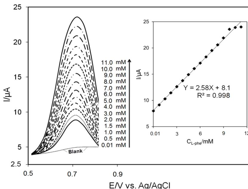
**Figure 8.** DP voltammograms of the biosensor in Gly/KOH/KCl buffer solution (pH 10.5) containing different concentrations of L-phe (0.01-11mM). Inset represents a linear response attributed to L-phe increasing in range of 0.01 to 11mM. Initial working volume: 12ml; supporting electrode: 100mM Gly/KOH/KCl buffer pH 10.5 containing 2.5mM  $NAD^+$ .
