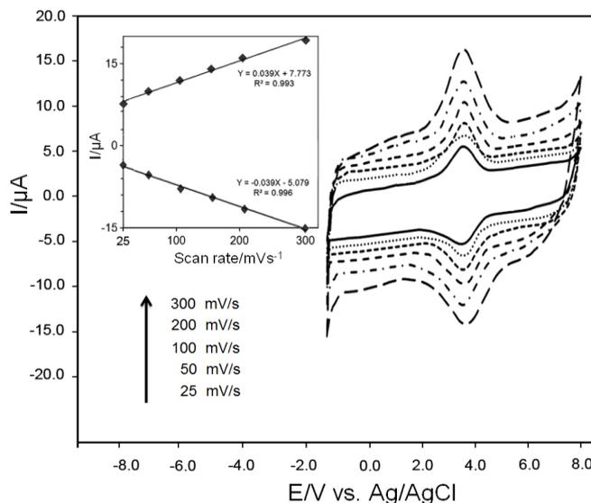
**Figure 5.** Cyclic voltammograms at various scan rates from 25, 50, 100, 200, to 300mVs<sup>-1</sup>, respectively. Inset: plot of peak currents vs. scan rates. Initial working volume: 12ml; supporting electrode: 100mM Gly/KOH/KCl buffer pH 10.5containing 2.5mM NAD<sup>+</sup>.
