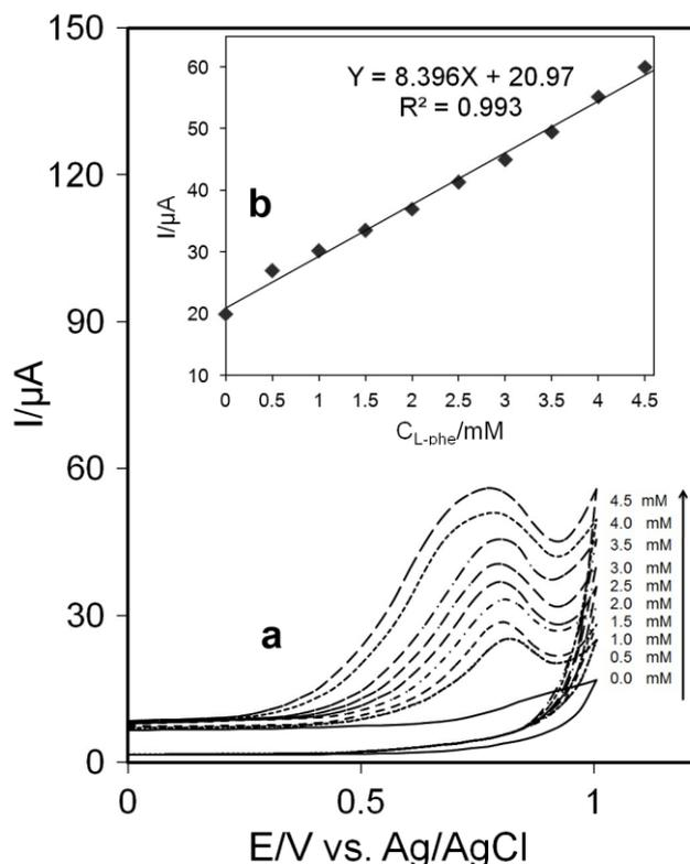
**Figure 6.** (a) Cyclic voltammograms of the enzyme electrode at scan rate of 25 mV/s containing 2.5 mM NAD<sup>+</sup>, blank (solid), and 0.5, 1, 1.5, 2, 2.5, 3, 3.5, 4, 4.5mM, of L-phe, respectively (dashed), (b) plot of peak currents vs. different concentration of L-phe (0-4.5mM). Initial working volume: 12ml; supporting electrode: 100mM Gly/KOH/KCl buffer pH 10.5containing 2.5mM NAD<sup>+</sup>.
