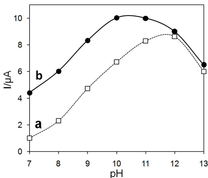
**Figure 2.** Effect of pH on catalytic activity (amperometric response) of the suspended enzyme (a) and the enzyme electrode (b). Applied potential: 1.0V; temperature: 23 °C; initial working volume: 12ml; supporting electrode: 100mM Gly/KOH/KCl buffer pH 10.5 containing 2.5mM NAD<sup>+</sup>.
