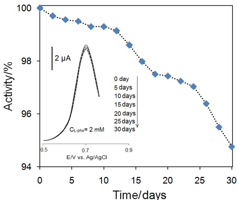
**Figure 10.** DPV responses to the enzyme electrode after 0 to 30 days kept in a cold room at 2 mM concentration of L-phe. Inset: DP voltammograms of peak currents vs. voltage. Initial working volume: 12ml; supporting electrode: 100mM Gly/KOH/KCl buffer pH 10.5 containing 2.5mM  $\text{NAD}^+$ .
