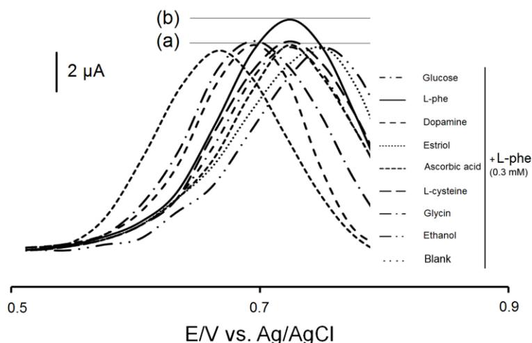
**Figure 9.** DP voltammograms recorded for the solutions of 1 mM glucose, 1 mM estriol, 1 mM ethanol, 1 mM glycin, 1 mM L-cysteine, 1 mM ascorbic acid and 1 mM dopamine (a), and 0.5 mM L-phe (b). Initial working volume: 12ml; supporting electrode: 100mM Gly/KOH/KCl buffer pH 10.5 containing 2.5mM  $\text{NAD}^+$  and 0.3mM L-phe.
