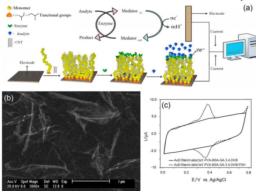
**Figure 1.** (a) Scheme depicting the functional principles of the L-phe biosensor,(b) SEM image of PDH–nanocomposite, and (c) cyclic voltammograms of AuE/starch-MWCNT-PVA-CMC-BSA-GA-3,4-DHB (solid) and AuE/starch-MWCNT-PVA-CMC-BSA-GA-3,4-DHB-PDH (dashed) in 0.1M Gly/KOH/KCl buffer solution (pH 10.4) at scan rate of 25mVs<sup>-1</sup>.
