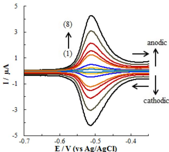
**Figure 4.** CVs of 0.05 mM ZFN solution between -0.2 and -0.7 V with different scan rates in BR of pH 5.5, (scan rates in  $Vs^{-1}$ : (1) 0.05, (2) 0.075, (3) 0.10, (4) 0.25, (5) 0.35, (6) 0.50, (7) 0.70, (8) 1.00)
