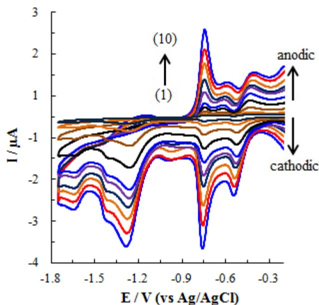
**Figure 2.** CVs of 0.5 mM ZFN solution with different scan rates in BR of pH 5.5 (scan rates in  $\text{Vs}^{-1}$ : (1) 0.03, (2) 0.05, (3) 0.10, (4) 0.18, (5) 0.25, (6) 0.35, (7) 0.50, (8) 0.65, (9) 0.80, (10) 1.00)
