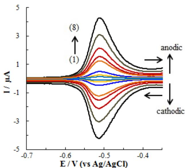
**Figure 4.** CVs of 0.05 mM ZFN solution between -0.2 and -0.7 V with different scan rates in BR of pH 5.5, (scan rates in  $\text{Vs}^{-1}$ ): (1) 0.05, (2) 0.075, (3) 0.10, (4) 0.25, (5) 0.35, (6) 0.50, (7) 0.70, (8) 1.00
