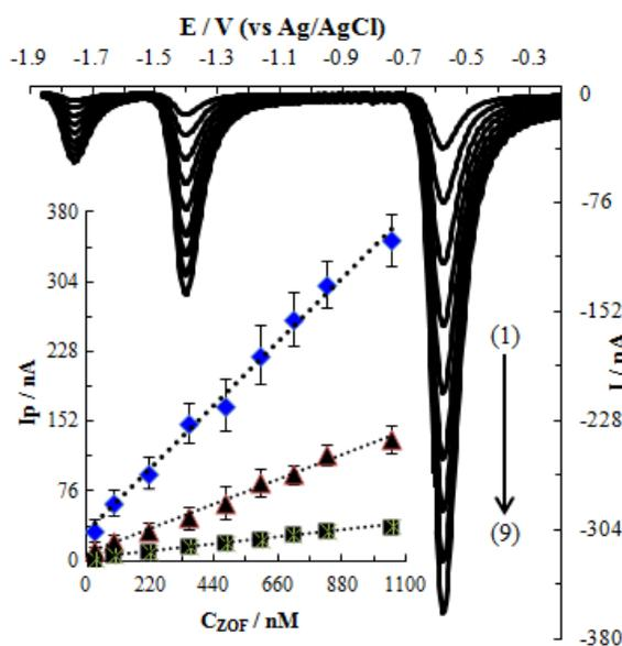
**Figure 7.** SWCAdSVs for calibration studies of ZFN at optimum conditions and calibration curves for PcI, PcII and PcIII, (concentrations: (1) 0.03, (2) 0.09, (3) 0.22, (4) 0.35, (5) 0.48, (6) 0.60, (7) 0.71, (8) 0.83, (9) 1.05  $\mu\text{M}$ )
