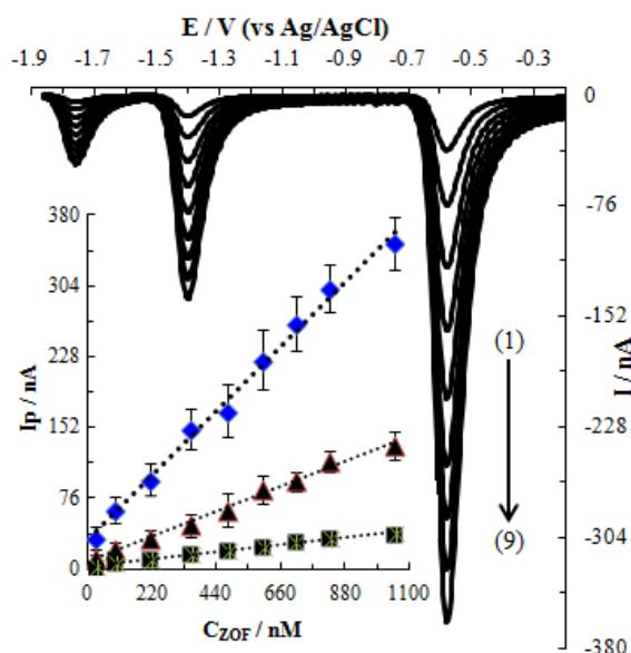
**Figure 7.** SWCAdSVs for calibration studies of ZFN at optimum conditions and calibration curves for Pcl, PclI and PclII, (concentrations: (1) 0.03, (2) 0.09, (3) 0.22, (4) 0.35, (5) 0.48, (6) 0.60, (7) 0.71, (8) 0.83, (9) 1.05  $\mu\text{M}$ )
