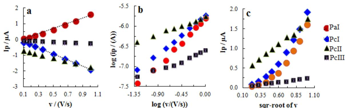
**Figure 3.** (a) Peak current vs. scan rate (b) logarithm of peak current vs. logarithm of scan rate (c) peak current vs. square-root of scan rate
