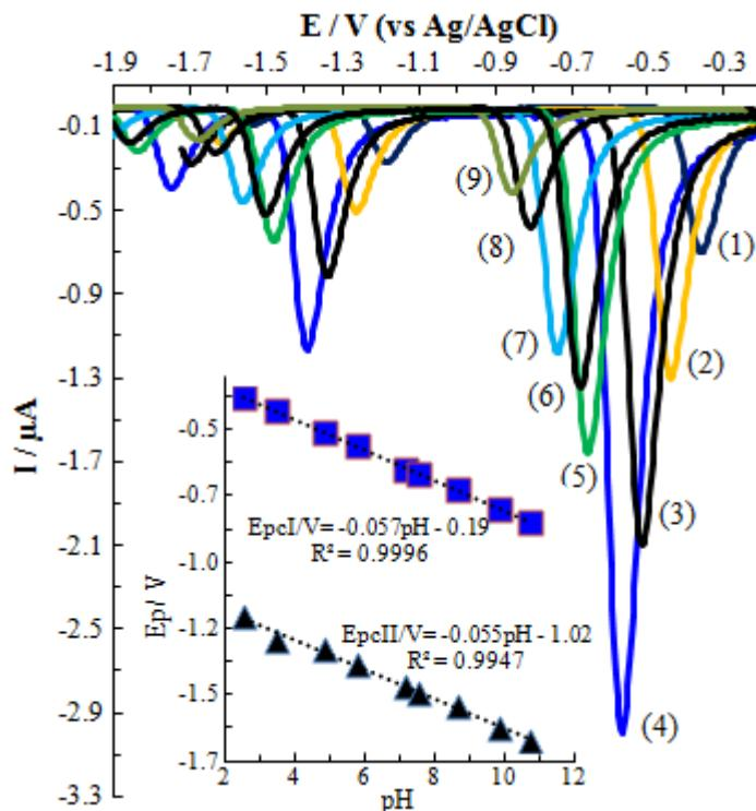
**Figure 5.** SWVs of 10.0  $\mu$ M ZFN solution for different pHs (pH values: (1) 2.5, (2) 3.5, (3) 4.8, (4) 5.5, (5) 7.1, (6) 7.6, (7) 8.6, (8) 9.7, (9) 10.8, inset: peak potential vs. pH)
