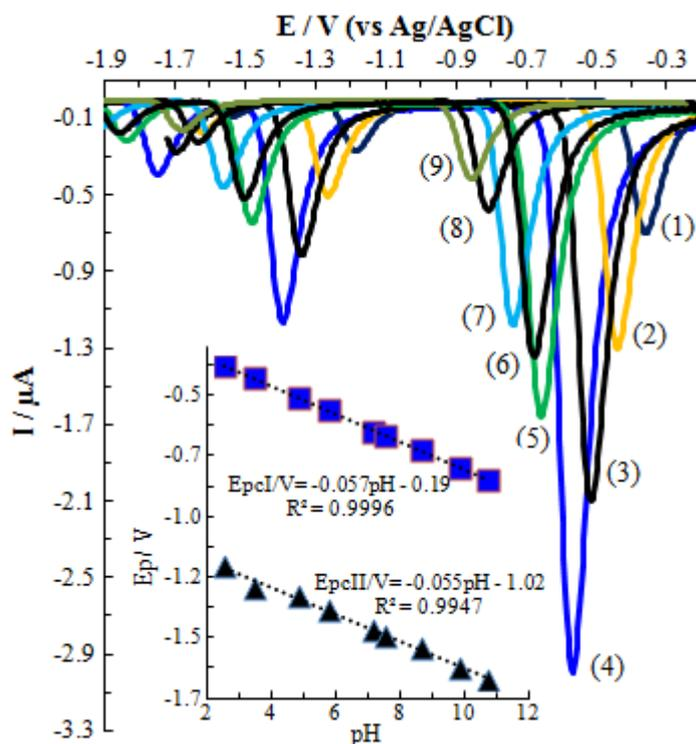
**Figure 5.** SWVs of 10.0 μM ZFN solution for different pHs (pH values: (1) 2.5, (2) 3.5, (3) 4.8, (4) 5.5, (5) 7.1, (6) 7.6, (7) 8.6, (8) 9.7, (9) 10.8, inset: peak potential vs. pH)
