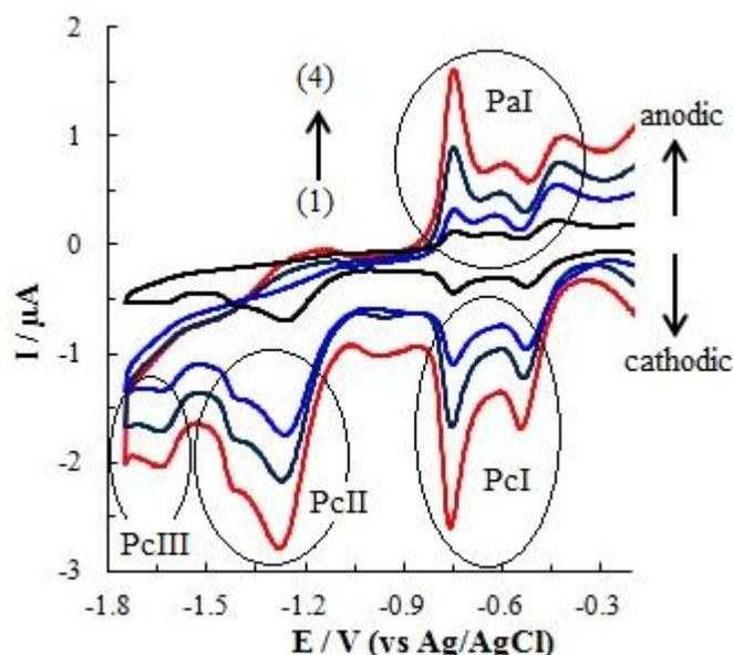
**Figure 1.** CVs of ZFN solutions with different concentrations (1) 0.5, (2) 1.0, (3) 1.5, (4) 2.0 mM in BR of pH 5.5, Scan rate: 0.100 Vs<sup>-1</sup>
