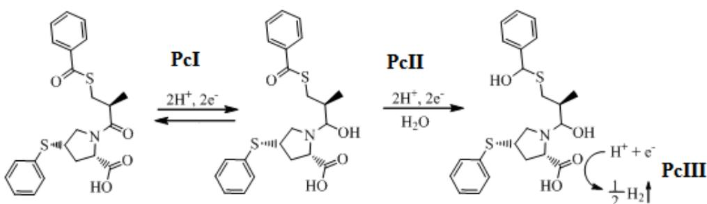
**Scheme 2.** Proposed reduction mechanisms for PcI, PcII and PcIII
