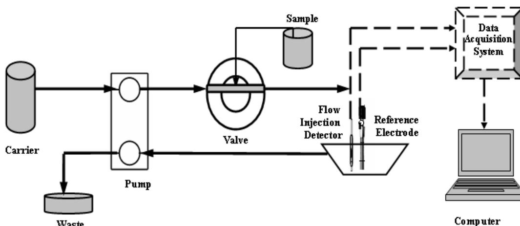
**Figure 2.** Manifold for the FIA set up used for the determination of CFZN.
