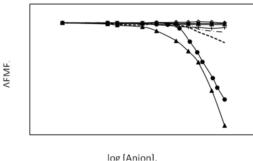
**Figure 8.** Potentiometric responses of CFZN sensitive electrodes using TDMAC based membrane electrodes, measured in 50 mM acetate buffer pH 5.5, towards various anions, additives and some cephalosporins: (●)  $CFZN^-$ , (---) Cefadroxil, (⋄) Cefoperazone, (....)  $Cl^-$ , (Δ)  $SO_4^{2-}$ , (▲)  $NO_3^-$ , (○)  $CH_3COO^-$ , (\*) Cefradine, (—|—) Cefaclor, (-.-.-) Ceftazidime, (...◆...) glucose, (□) fructose and (—) maltose.
