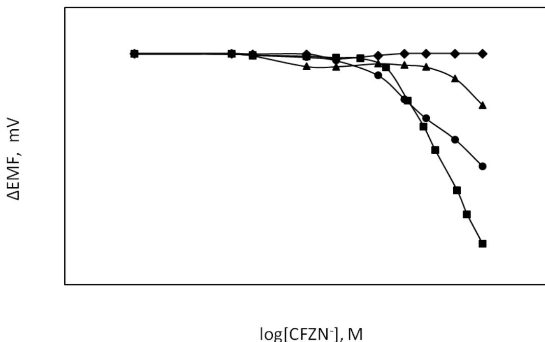
**Figure 3.** Potentiometric response of various PVC membrane electrodes towards CFZN measured in 50 mM acetate buffer, pH 5.5. The ion-exchangers tested were (■) TDMAC, (●) TDMAB, (◆) BTBAB and (▲) EBTPPB.
