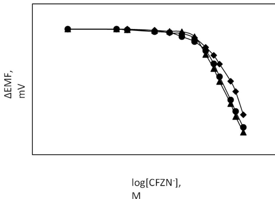
**Figure 5.** Potentiometric response of TDMAC based membrane electrodes formulated with different solvents mediators; (▲) *o*-NPOE, (●) DOS and (◆) FPNPE.
