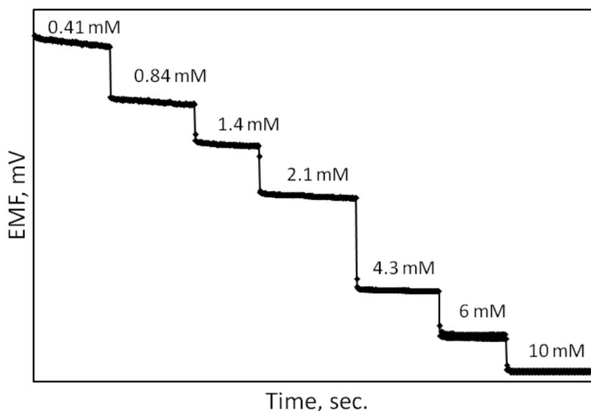
**Figure 7.** Response time of TDMAC based membrane sensor towards CFZN measured in acetate buffer pH 5.5.
