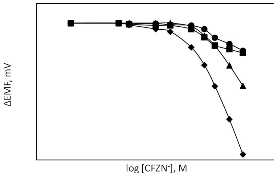
**Figure 4.** Potentiometric response of various PVC membrane electrodes towards CFZN measured in 50 mM acetate buffer, pH 5.5. The ionophores tested were (■)Pd TPP-Cl<sub>2</sub>, (●)Sn TPP-Cl<sub>2</sub>, (▲)Cu OEP and (◆)Zn OEP.
