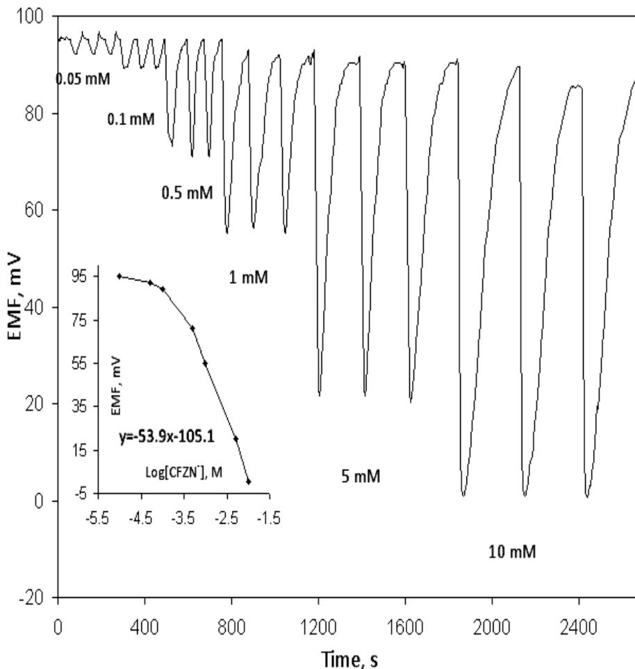
**Figure 9.** Typical (FIA) peaks produced by injection of standard CFZN through 150 µl valve loop into a stream of 50 mM acetate buffer pH 5.5 using the TDMAC based membrane sensor. The inset shows a FI response curve.
