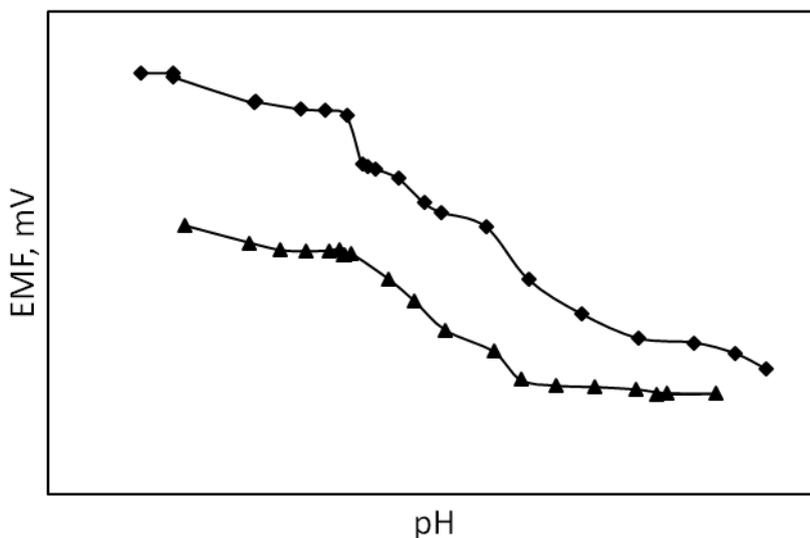
**Figure 6.** Influence of pH on the potentiometric response of TDMAC based membrane sensor in presence of: (▲) 10 mM and (◆) 1 mM CFZN.
