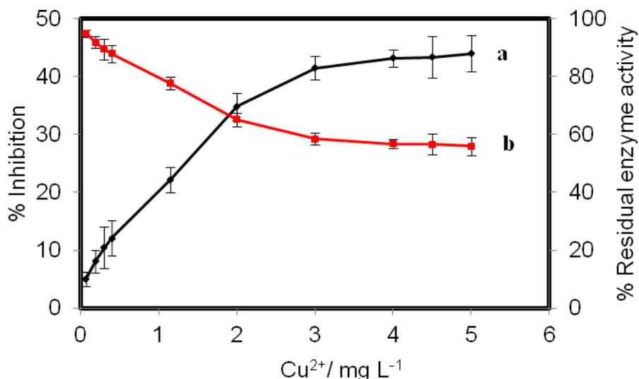
**Figure 8.** Dose-dependent enzyme inhibition (a) and residual enzyme activity (b) of  $\text{Cu}^{2+}$  towards HRP-catalyzed  $\text{H}_2\text{O}_2$ , Error bar =  $\pm$  S.D. and  $n = 3$ .
