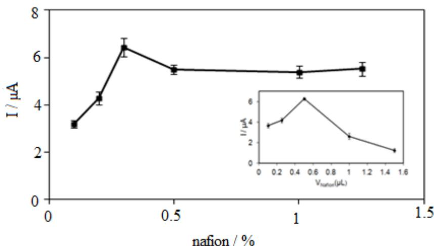
**Figure 4.** Influence of nafion concentrations on the electrocatalytic response current obtained by HRP/MT-MWCNT biosensor in the presence of 0.1 mM  $\text{H}_2\text{O}_2$  in 0.1 M PBS (pH 7.0). Error bar =  $\pm$  S.D. and  $n = 3$ .
