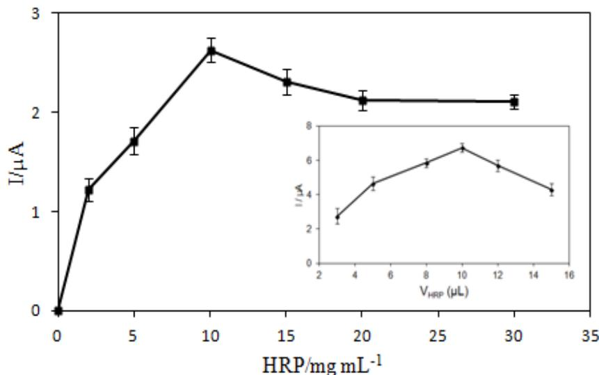
**Figure 3.** The effect of amount of HRP on the response current of HRP/MT-MWCNT biosensor in 0.1 M PBS (pH 7.0), Scan rate:  $50 \text{ mV s}^{-1}$ . *Inset:* Current responses of volume HRP injected on the MT-MWCNT/GCE. Error bar =  $\pm$  S.D. and  $n = 3$ .
