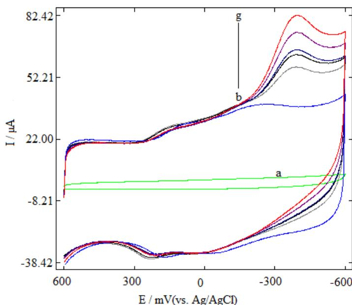
**Figure 1.** (A) Cyclic voltammograms of GCE (a), HRP biosensor in 0.1 M PBS, pH 7.0 and 0.1 M KCl (b) without substrate, (c–g) with 0.01–0.5 mM substrate.
