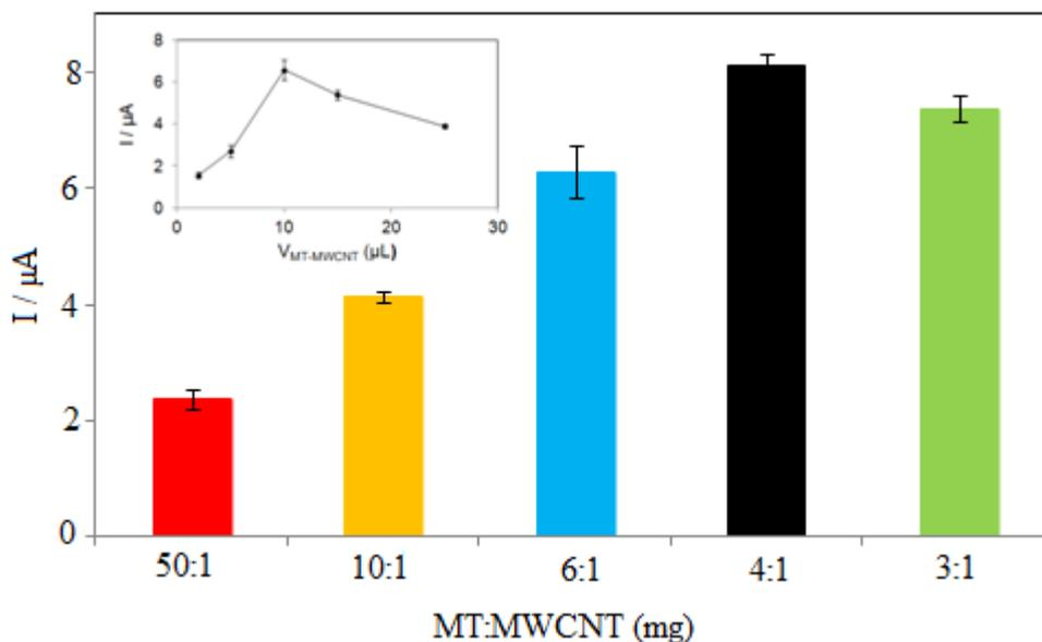
**Figure 2.** Current responses of the HRP/MT-MWCNT biosensor loading variable amount of MT: MWCNT amount to 0.1 mM  $\text{H}_2\text{O}_2$  in 0.10 M PBS (pH 7.0). *Inset:* Current responses of volume MT-MWCNT injected on the GCE. Error bar =  $\pm$  S.D. and  $n = 3$ .
