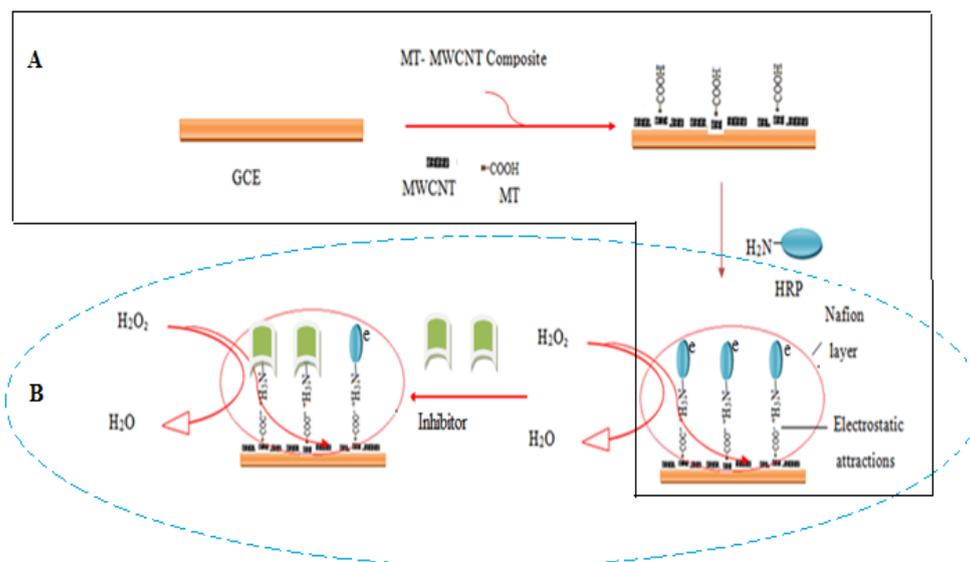
**Scheme 1.** Fabrication process (A) Inhibition process (B)
