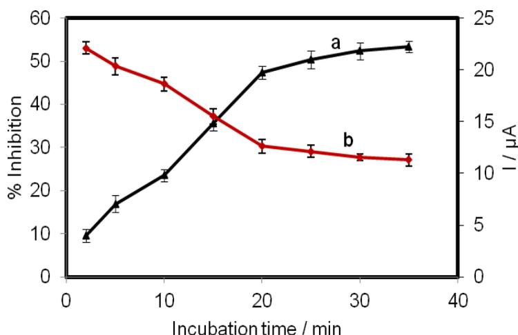
**Figure 7.** The effect of incubation time on the biosensor response (a) and enzyme activity decay (b) in 0.5 mg L<sup>-1</sup> Cu<sup>2+</sup> 0.1 M PBS (pH 7.0) and 0.1 mM H<sub>2</sub>O<sub>2</sub>, Error bar = ± S.D. and  $n = 3$ .
