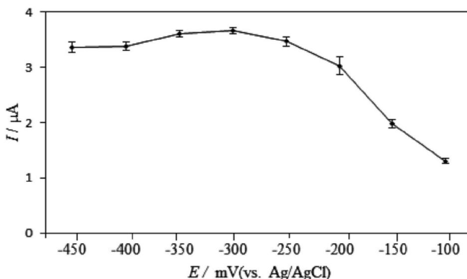
**Figure 6.** Effects of the applied potential on the performance of HRP/MT-MWCNT biosensor in the presence of same concentration of  $\text{H}_2\text{O}_2$  in 0.1 M PBS. Error bar =  $\pm$  S.D. and  $n = 3$ .
