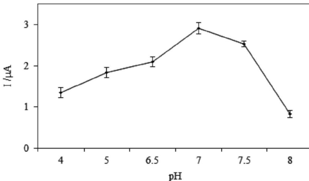
**Figure 5.** Effects of solution pH on the performance of HRP/MT-MWCNT biosensor in the presence of same concentration of  $\text{H}_2\text{O}_2$  in 0.1 M PBS. Error bar =  $\pm$  S.D. and  $n = 3$ .
