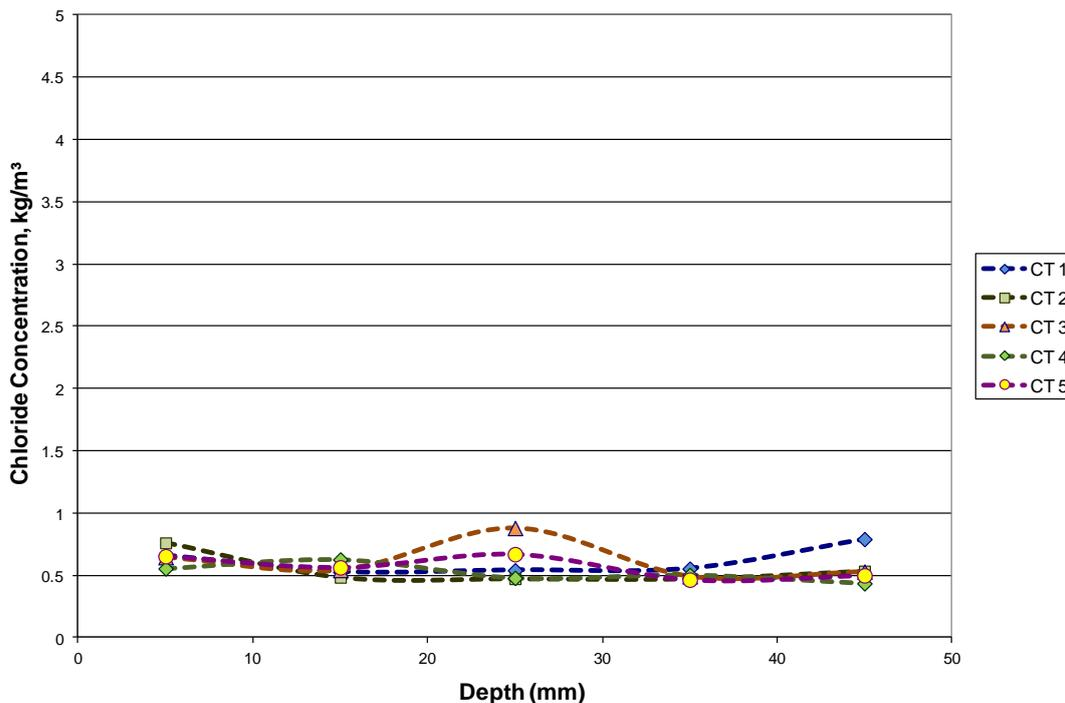
Figure 7. Chloride concentration from Chetumal (CT) houses, kg/m<sup>3</sup> of concrete.
