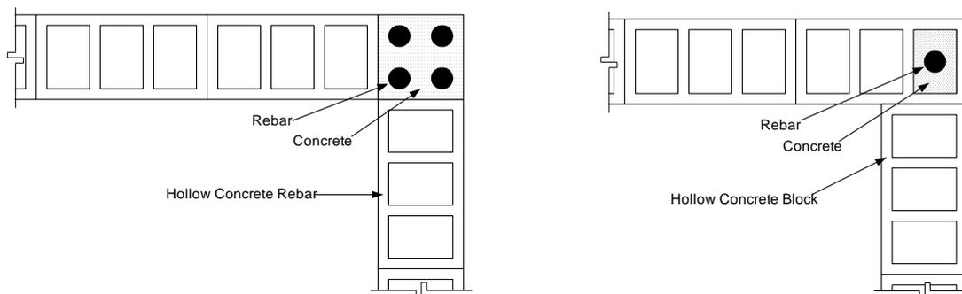
**Figure 2.** Wall corner detail (plant view).
