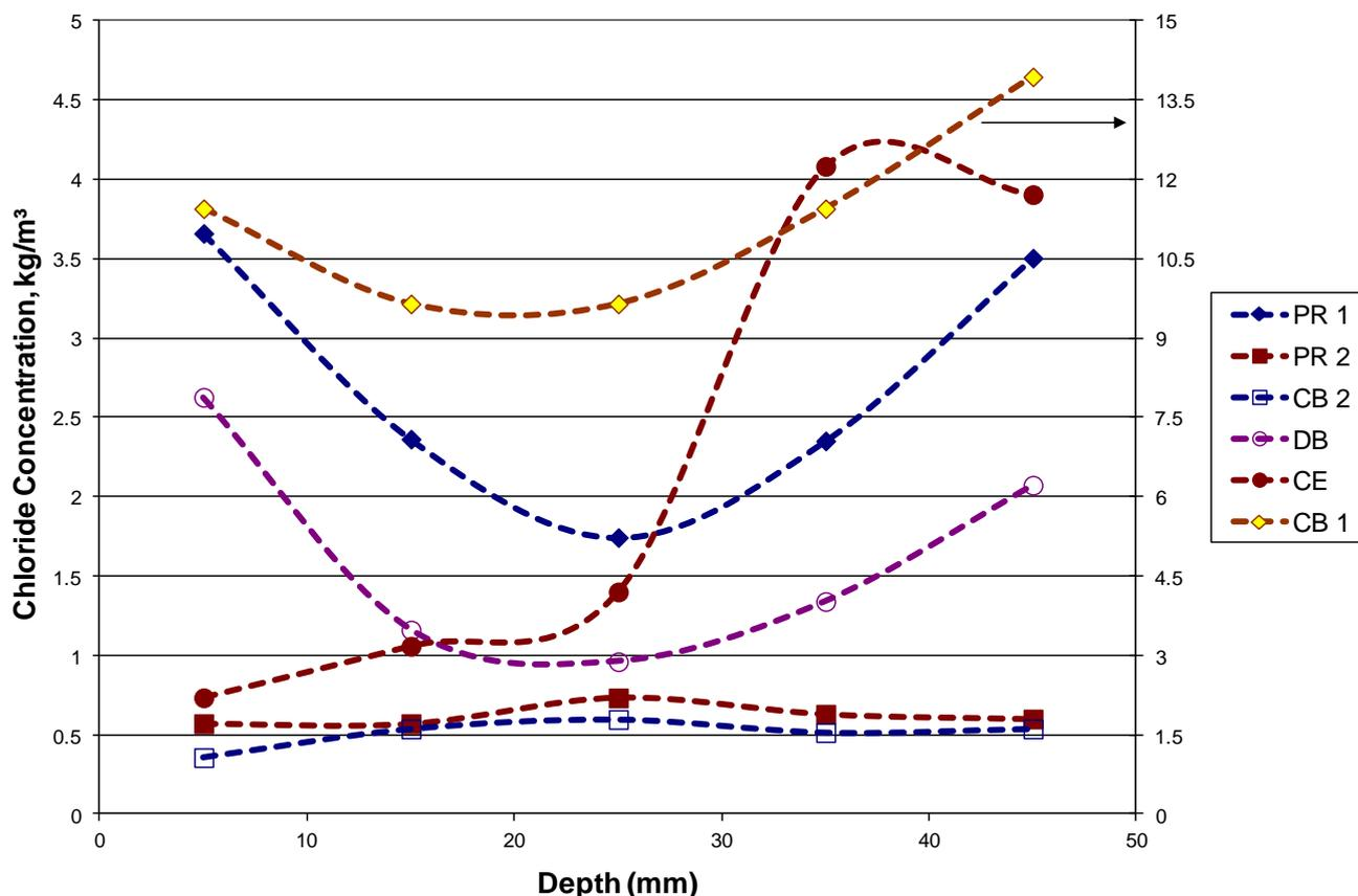
**Figure 5.** Chloride concentration from Celestun (CE), Progreso (PR), Chabihau (CB) and Dzilam-Bravo (DB) houses, in kg/m<sup>3</sup> of concrete.
