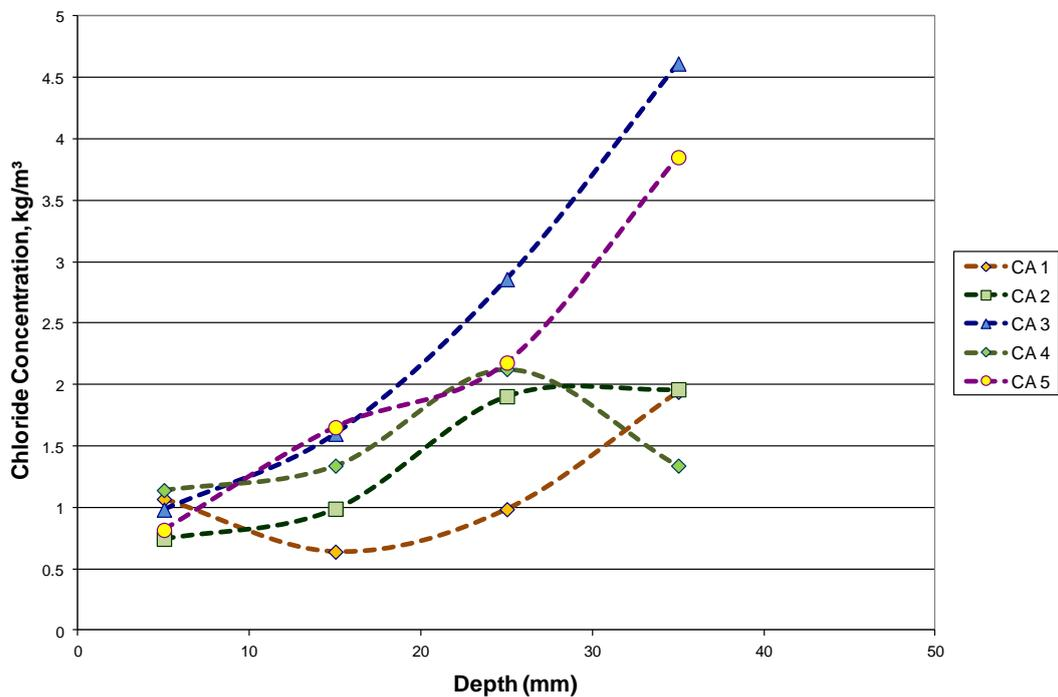
Figure 6. Chloride concentration from Cancun (CA) houses, kg/m<sup>3</sup> of concrete.
