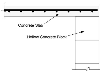
**Figure 1.** Reinforced concrete slab.
