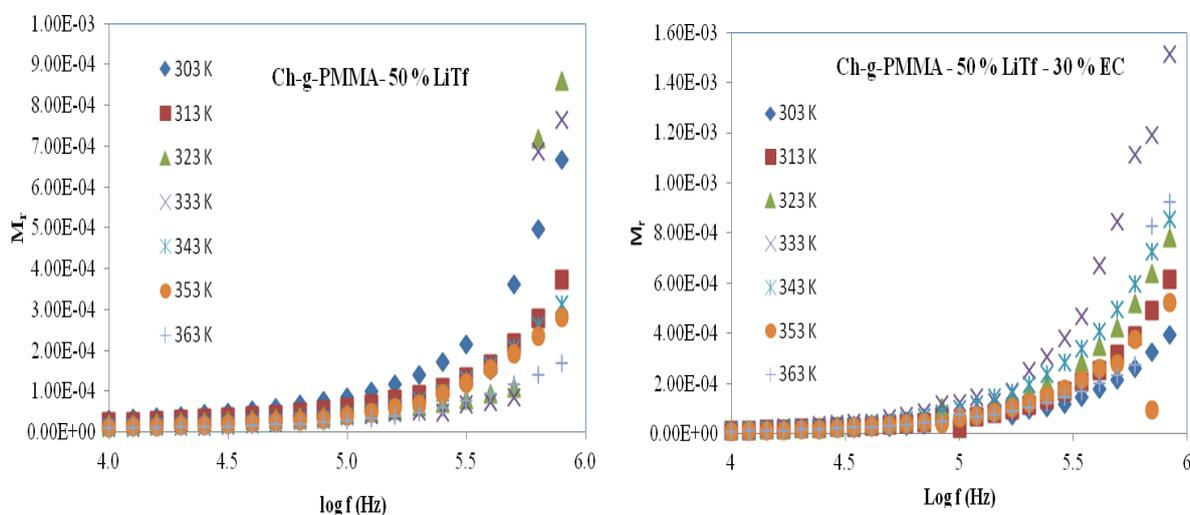
**Figure 7.** Variation of real part of the electric constant ( $M_r$ ) as a function of frequency at various temperature for the unplastized (Ch-g-PMMA-50 % LiTf) and plastized (Ch-g-PMMA-50 % LiTf -30 % EC) samples with highest conductivity.
