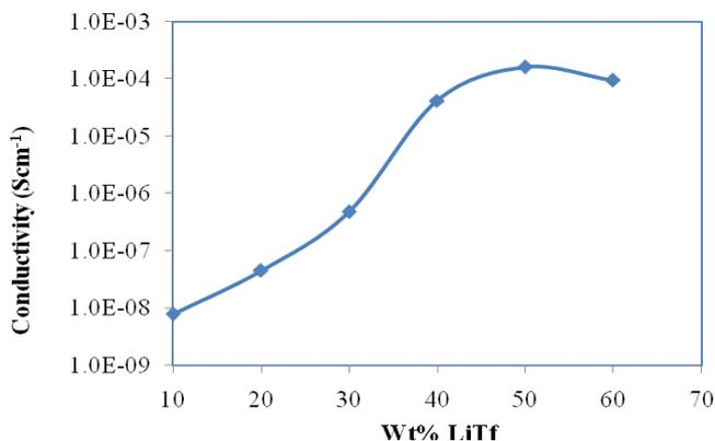
**Figure 2.** The dependence of ionic conductivity of salted system at room temperature (30 °C).
