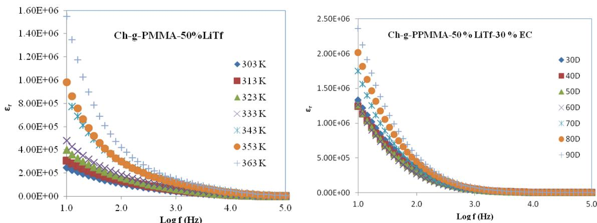
**Figure 5.** Variation of real part of the electric constant ( $\epsilon_r$ ) as a function of frequency at various temperature for the unplasticized (Ch-g-PMMA-50 % LiTf) and plasticized (Ch-g-PMMA-50 % LiTf -30 % EC) samples with highest conductivity.
