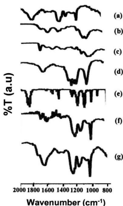
**Figure 1.** FTIR spectrum of (a) pure PMMA, (b) pure Chitosan (c) Chitosan-g-PMMA (d) pure LiTf (e) pure EC (f) Chitosan-g-PMMA -50 wt% LiTf (g) Chitosan-g-PMMA-50 wt% LiTf – 30 % EC
