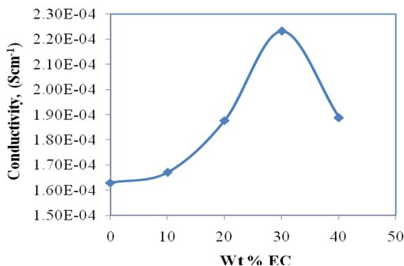
**Figure 3.** The dependence of ionic conductivity of plasticized system at room temperature (30 °C).
