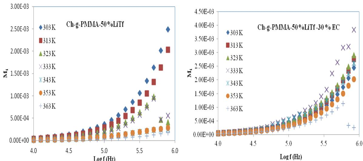
**Figure 8.** Variation of imagine part of the electric constant ( $M_i$ ) as a function of frequency at various temperature for the unplasticized (Ch-g-PMMA-50% LiTf) and plasticized (Ch-g-PMMA-50 % LiTf -30 % EC) samples with highest conductivity.
