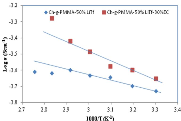
**Figure 4.** The relationship between  $\log \sigma$  and  $1000/T$  for the highest conductivity unplasticized (Ch-g-PMMA-50 % LiTf) and plasticized (Ch-g-PMMA-50 % LiTf -30 % EC) samples
