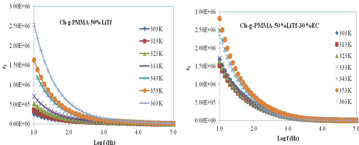
**Figure 6.** Variation of imagine part of the electric constant ( $\epsilon_i$ ) as a function of frequency at various temperature for the unplastized (Ch-g-PMMA-50 % LiTf) and plastized (Ch-g-PMMA-50 % LiTf -30 % EC) samples with highest conductivity.
