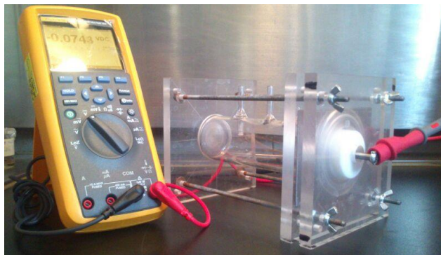
Figure 7. Cell designed to check the repeatability of the model B sensor.
