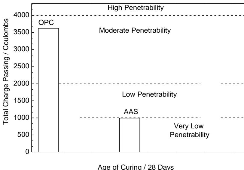
**Figure 4.** Values of permeability to chlorides in AAS concrete
