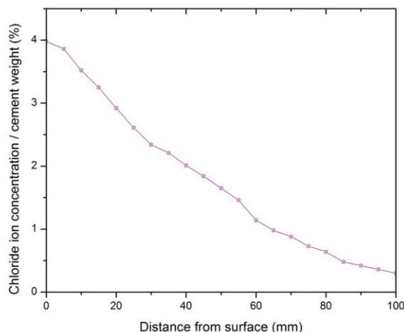
Figure 2. Chloride penetration profile (estimated mathematical model to 28 days)
