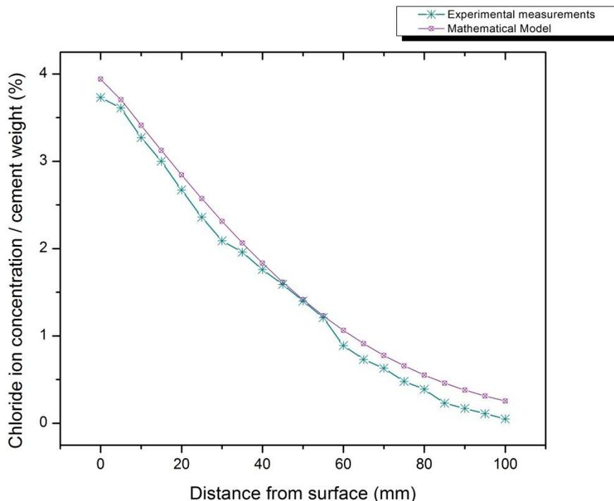
**Figure 3.** Comparison of chloride penetration profile obtained experimentally and theoretically by mathematical model in specimens tested at 28 days
