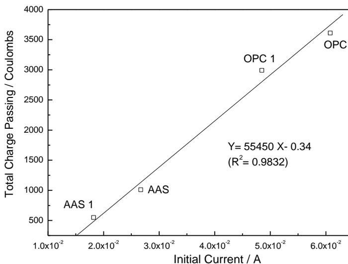
Figure 5. Relationship between the total charge applied and the initial current.
