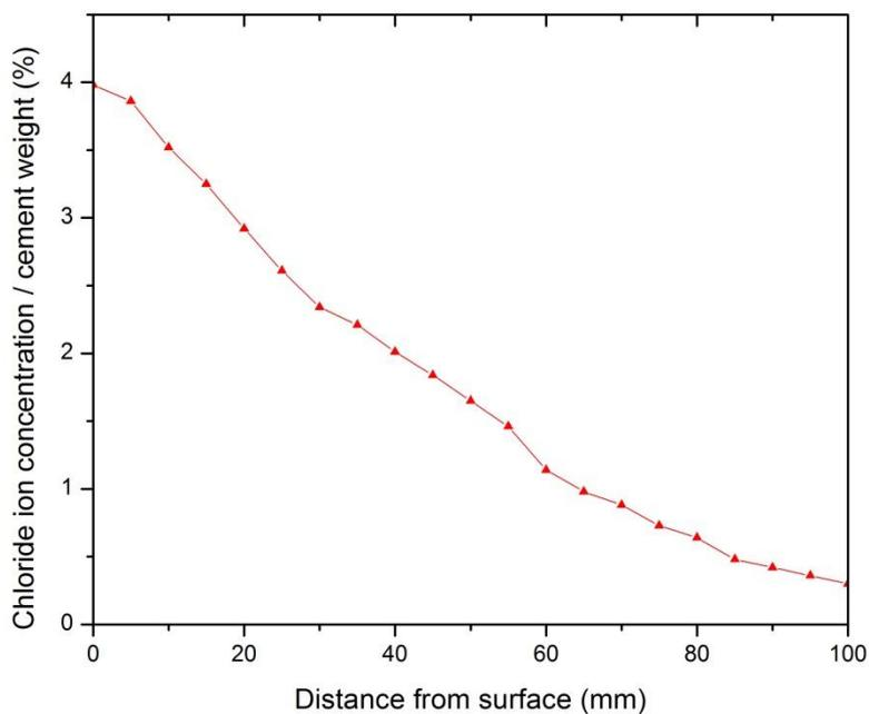
**Figure 1.** Chloride penetration profile (samples taken at 28 days)
