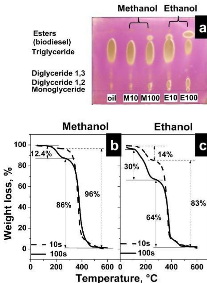
**Figure 4.** Thin layer chromatography a) and thermogravimetric analysis (b and c) showing the composition of the reaction mixture in region I and II using methanol or ethanol during the transesterification reaction of soybean oil. Samples were taken 10 and 100 seconds after adding alkoxide (agitation rate 600 rpm)
