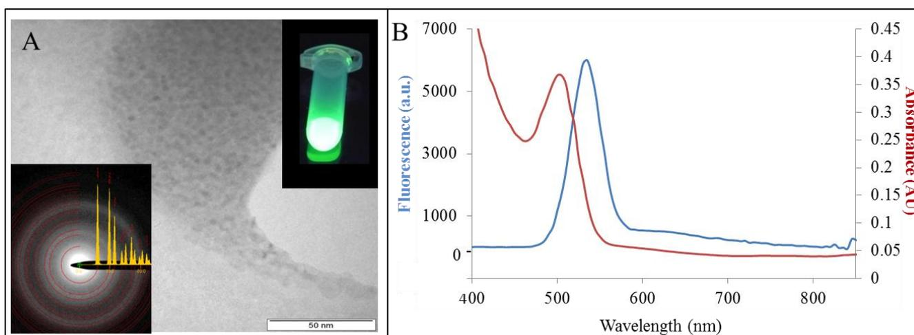
**Figure 1.** (A) TEM micrograph of the sample showing fine morphologies of QDs with the typical particles size below 10 nm; in inset: QDs solution under UV light illumination. (B) Absorption and emission spectra of CdTe QDs.
