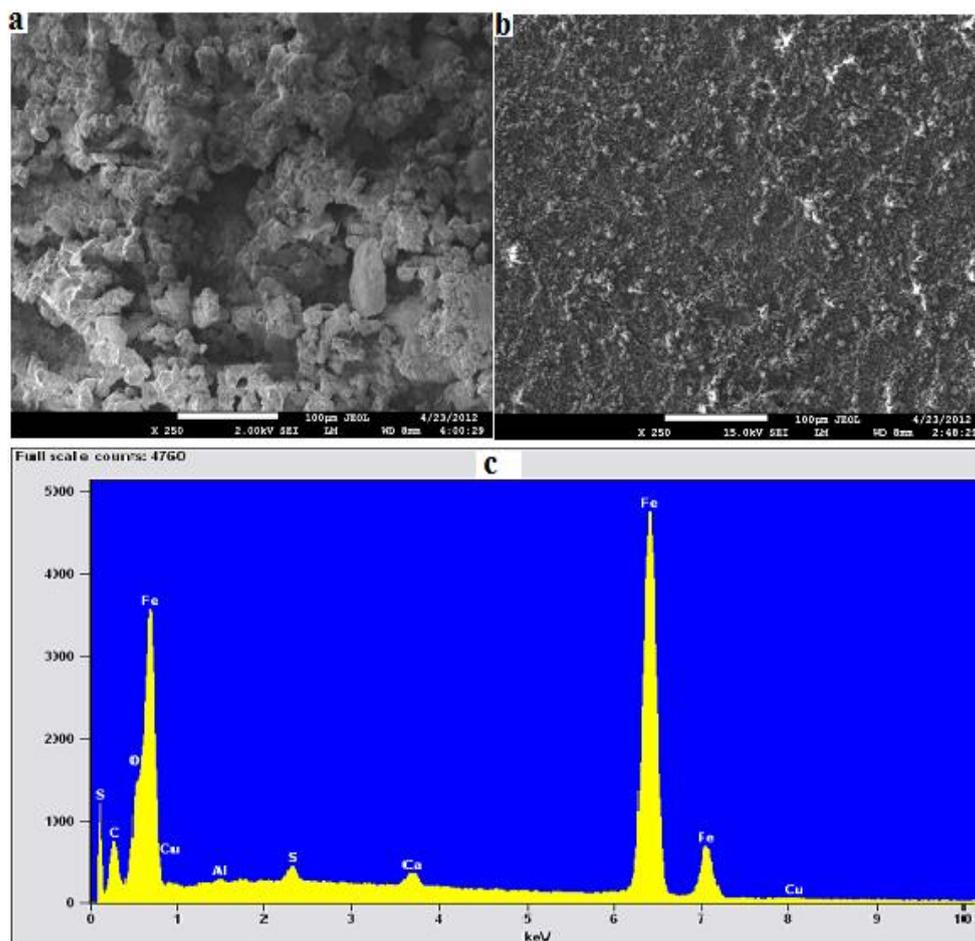
**Figure 4.** SEM micrographs of a) as-corroded uninhibited b) as-corroded inhibited in 50%v/v *Arachis hypogaea* -2M HCl solution after 36 h of immersion time c) EDS spectral for (b)
