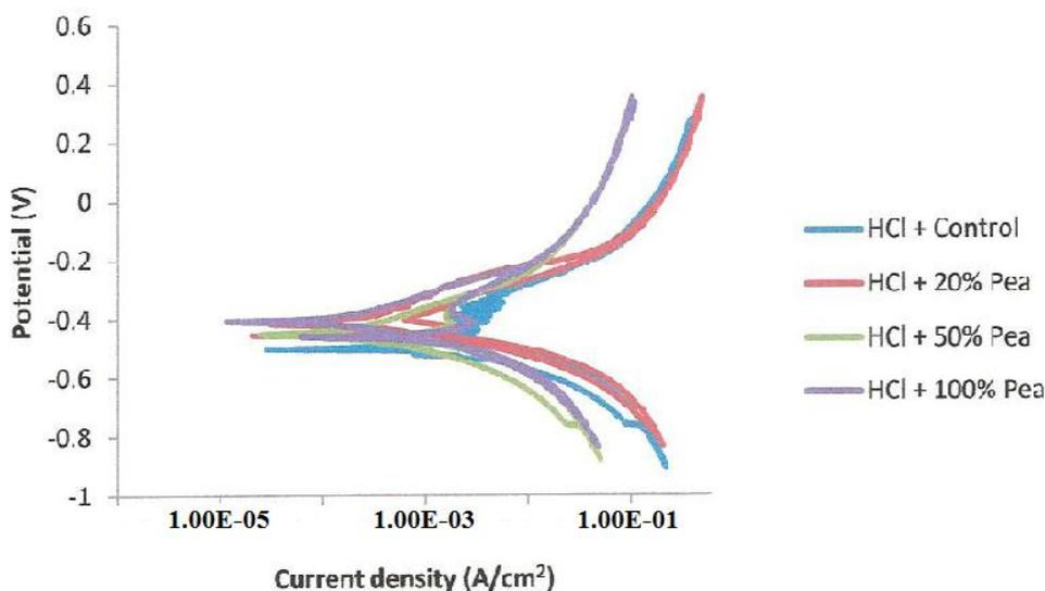
**Figure 3.** Linear polarization curves for mild steel in 2M HCl solution-*Arachis hypogaea* environment
