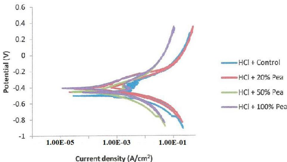
**Figure 3.** Linear polarization curves for mild steel in 2M HCl solution-*Arachis hypogaeae* environment
