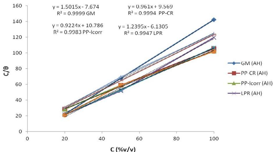
**Figure 6.** Langmuir isotherm for the adsorption of *Arachis hypogaea* compounds on the mild steel surface in 2M HCl solution at 25°C obtained by gravimetric and potentiodynamic polarization methods
