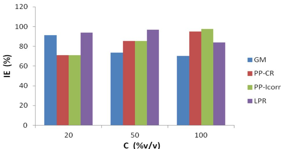
**Figure 5.** Comparative chart of inhibitor efficiency (IE) for mild steel-2M HCl solution/*Arachis hypogaea* concentration obtained by different techniques
