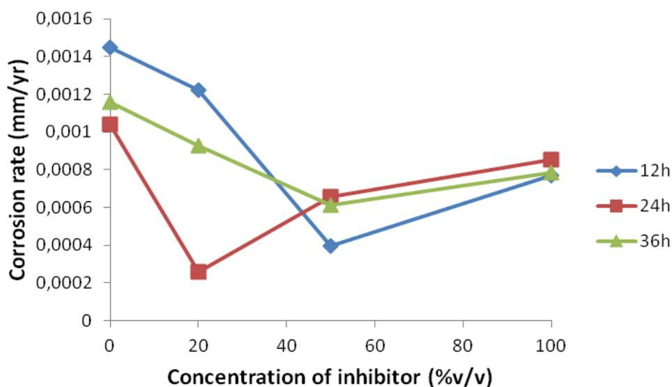
**Figure 2.** Variation of corrosion rate with concentration of inhibitor for mild steel in 2M HCl without and with varying concentration of *Arachis hypogaeae* at 25°C
