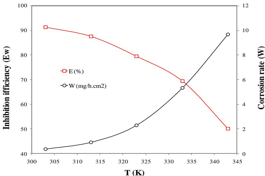
**Figure 2.** Variation of corrosion rate (W and inhibition efficiency ( $E_w$ ) of corrosion of mild steel in 1 M HCl with different temperatures in the presence of *S. inaequidens* essential oil
