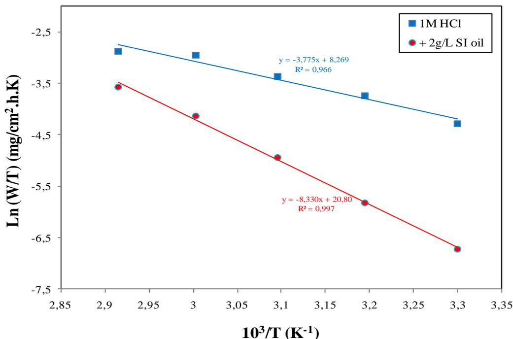
**Figure 4.** Transition-state plots for mild steel corrosion rates (W) in 1 M HCl in absence and in presence of 2 g/L of *S. inaequidens* essential oil.
