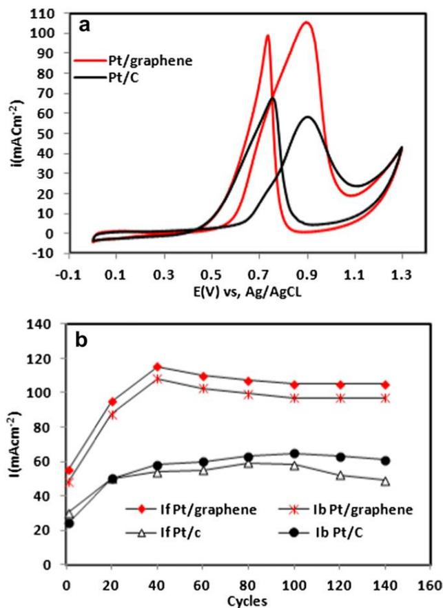
**Figure 3.** (a) Cyclic voltammograms of Pt/carbon and Pt/graphene composite electrodes in 1 M methanol recorded at a scan rate of 50 mVs<sup>-1</sup>. (b) Electrode cyclic stability for methanol oxidation (Reproduced with permission from ref. [57]).
