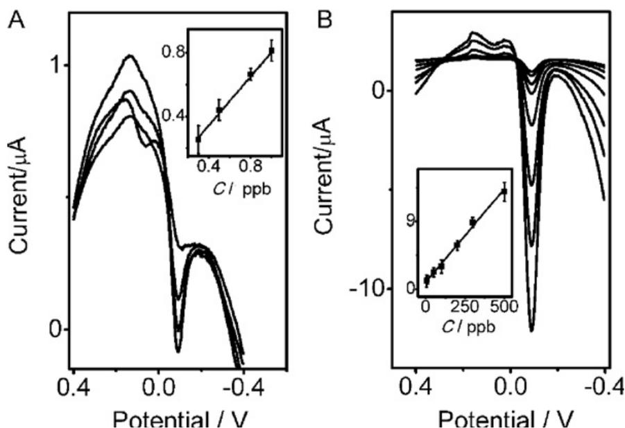
**Figure 7.** (A) DPV curves of the  $\beta$ -CD-graphene/GCE after the solid phase extraction of mp with various concentrations of 0.3, 0.5, 0.8 and 1.0 ppb. (B) The DPV curves of graphene composite after the solid phase extraction of mp with different concentrations of 1, 5, 10, 50, 100, 200, 300 and 500 ppb in 0.1 M PBS (Reproduced with permission from ref. [87]).
