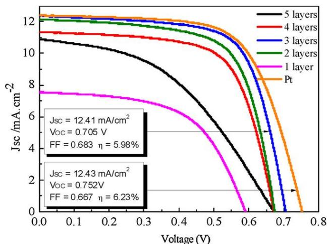
**Figure 4.** J-V curves of DSSCs with Pt counter electrode and MoS<sub>2</sub>/graphene counter electrode in different thickness (Reproduced with permission from ref. [98]).
