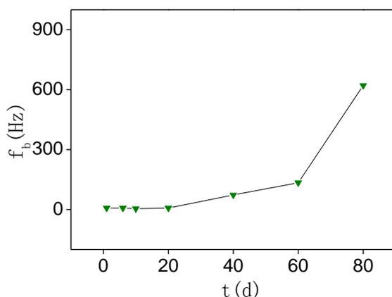
**Figure 6.** Evolution of breakpoint frequency with immersion time of the coatings
