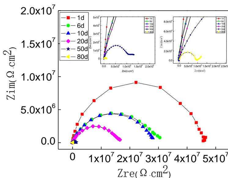
Figure 2. Nyquist spectra of PPE coating in period of immersion in 3.5% NaCl solution
