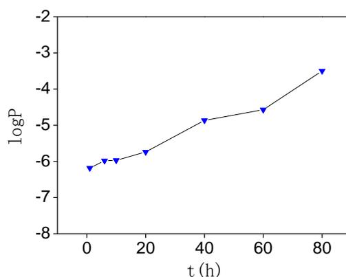
**Figure 5.** Porosity at different time of exposure to 3.5% solution
