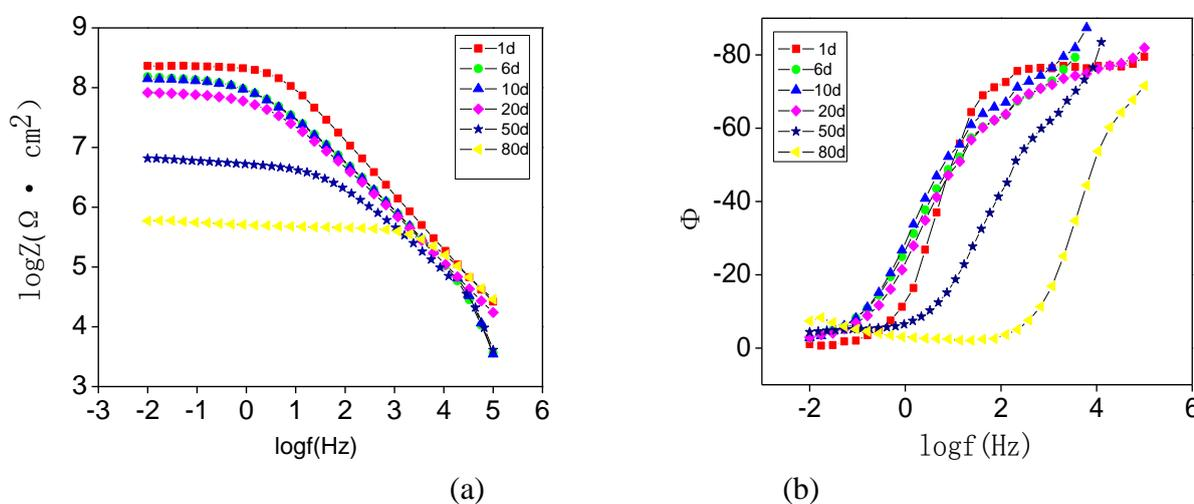
**Figure 1.** Bode spectra of PPE coating in period of immersion in 3.5% NaCl solution
