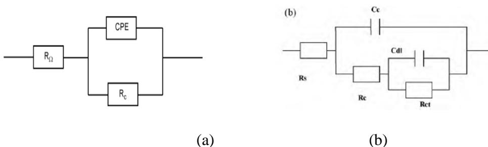
Figure 3. Equivalent circuits for the PPE coating in 3.5% NaCl solution at different stages
