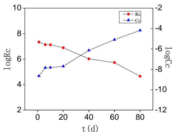
**Figure 4.** Time dependence of  $R_c$  and  $C_c$  of the coating
