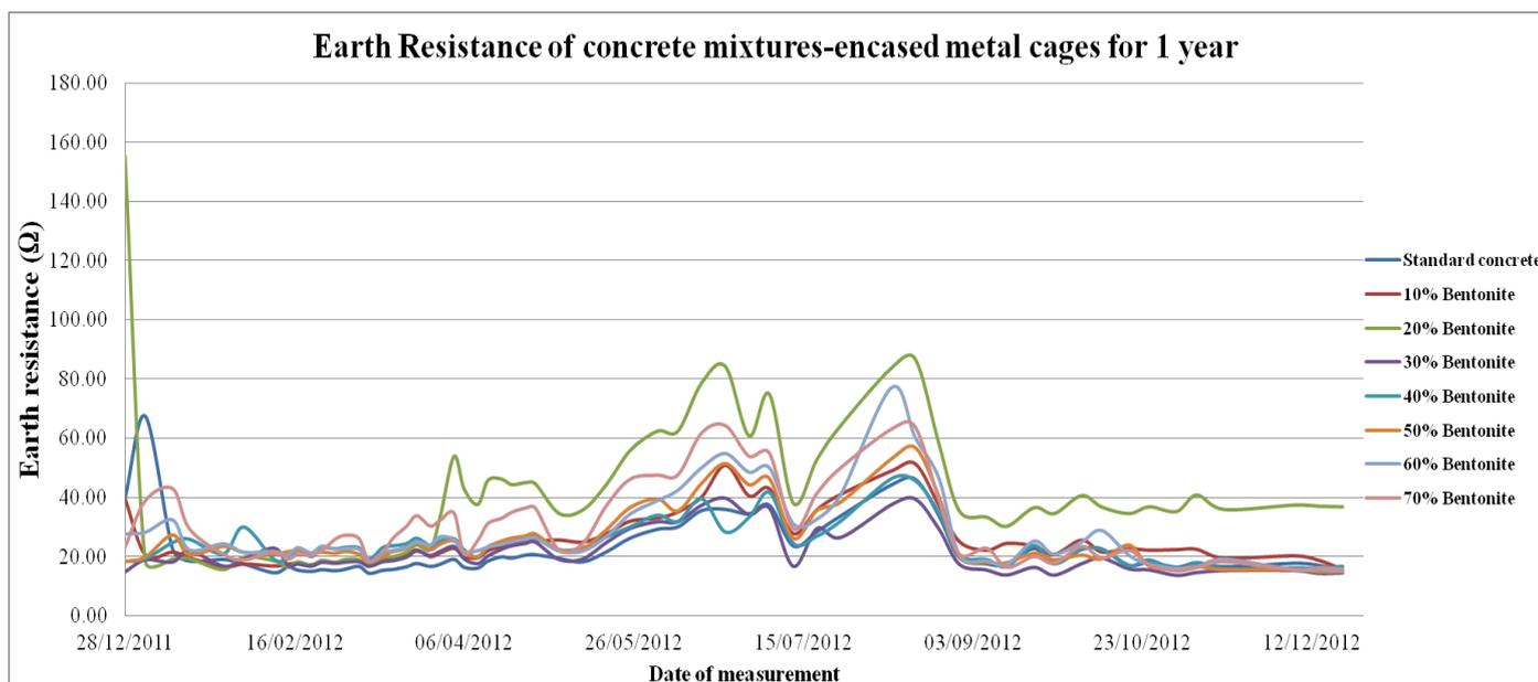
**Figure 4.** Grounding resistance of bentonite-mixed concrete encased metal cages for 12 months
