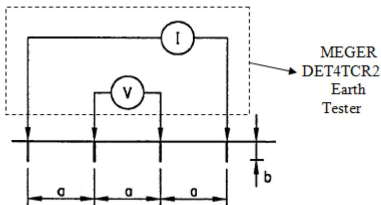
**Figure 3.** Soil resistivity measurement setup
