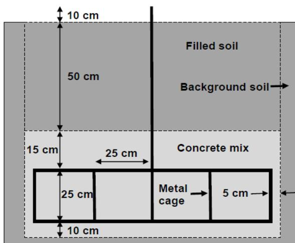
Figure 1. Setup for each pit [20]
