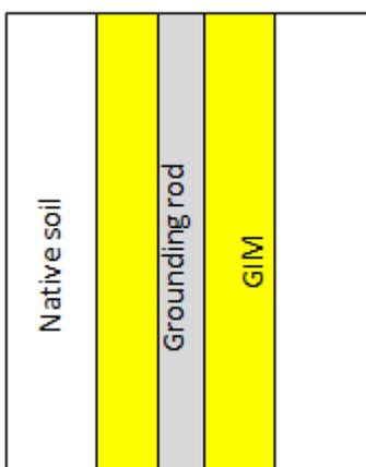
**Figure 9.** Augured-hole method for GIM-based grounding system [8]
