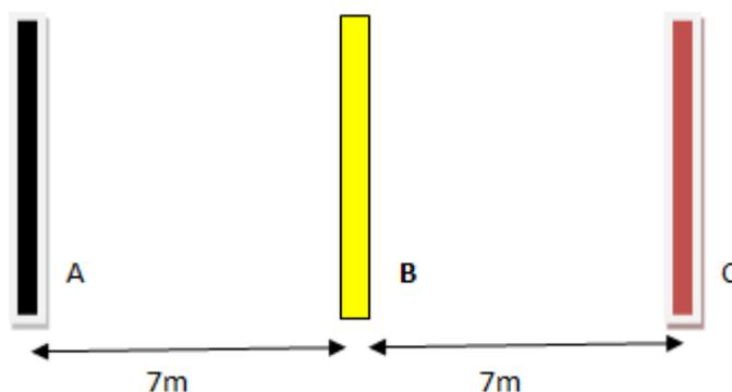
Figure 2. Grounding resistance measurement setup
