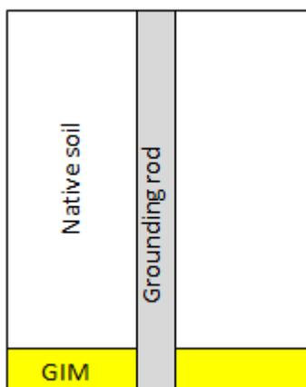
**Figure 10.** Pit method for GIM-based grounding system [8]
