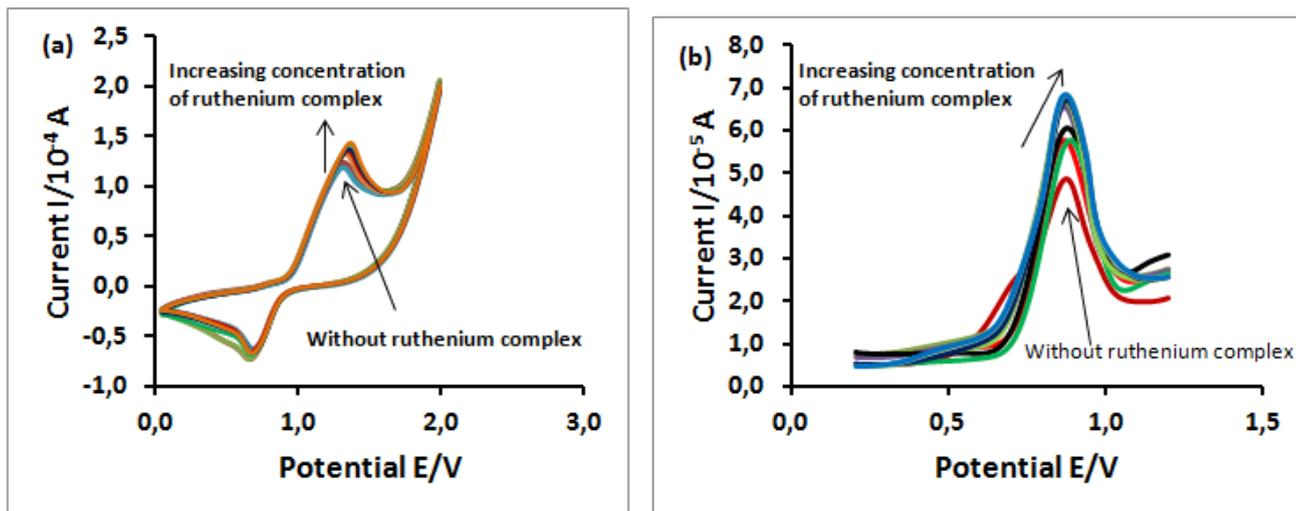
**Figure 1.** (a) CV and (b) DPV of ruthenium complex  $[Ru (phen)_2(qtpy)]^{2+}$  using AuE in TE buffer
