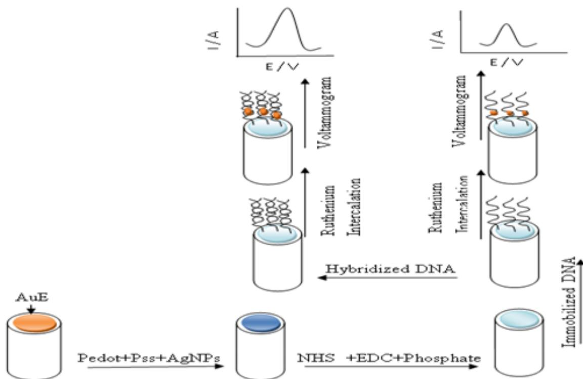
**Scheme 1.** Schematic representation of electrochemical detection of DNA immobilization and hybridization
