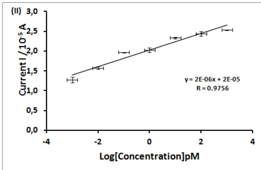
**Figure 4.** (I) Differential pulse voltammograms (DPV) on effect of target DNA concentration of (a) without target DNA, (b)  $1 \times 10^{-15}$  M, (c)  $1 \times 10^{-14}$  M, (d)  $1 \times 10^{-13}$  M, (e)  $1 \times 10^{-12}$  M, (f)  $1 \times 10^{-11}$  M, (g)  $1 \times 10^{-10}$  M, (h)  $1 \times 10^{-9}$  M (II) log(concentration) of target DNA against peak current
