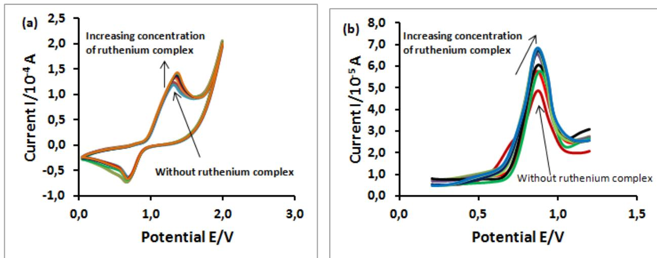
**Figure 1.** (a) CV and (b) DPV of ruthenium complex  $[\text{Ru}(\text{phen})_2(\text{qtpy})]^{2+}$  using AuE in TE buffer
