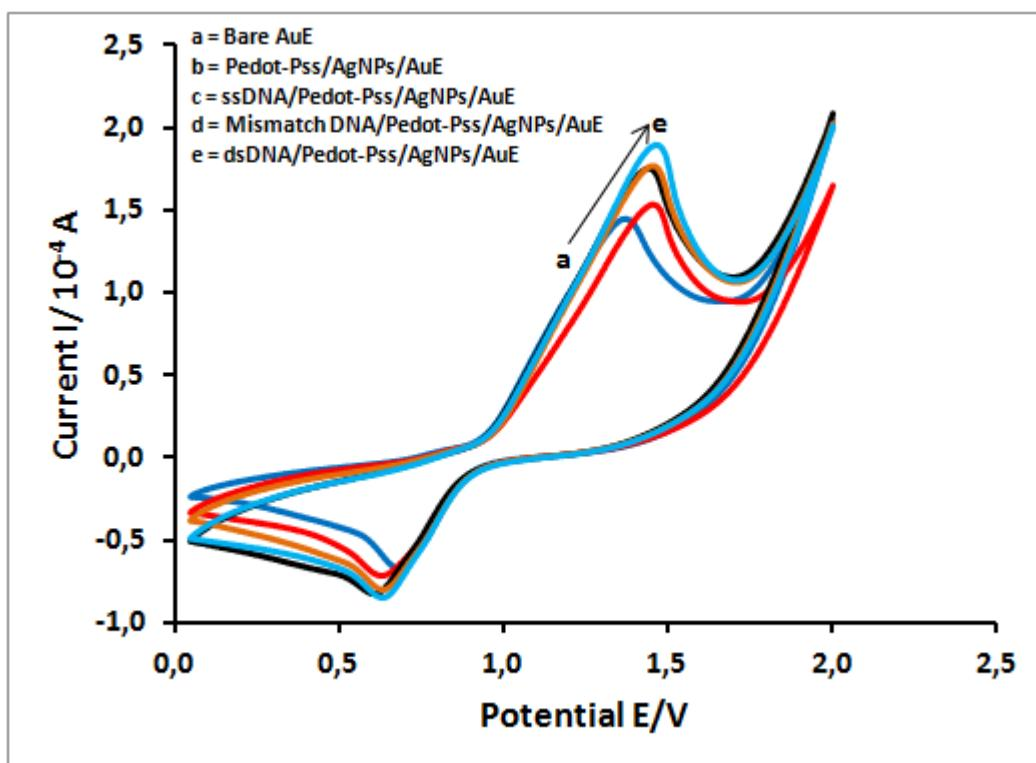
**Figure 3.** CV of (a) Bare AuE, (b) PEDOT-PSS/AgNPs/AuE, (c) ssDNA/PEDOT-PSS/AgNPs/AuE, (d) mismatchDNA/PEDOT-PSS/AgNPs/AuE, (e) dsDNA/PEDOT-PSS/AgNPs/AuE
