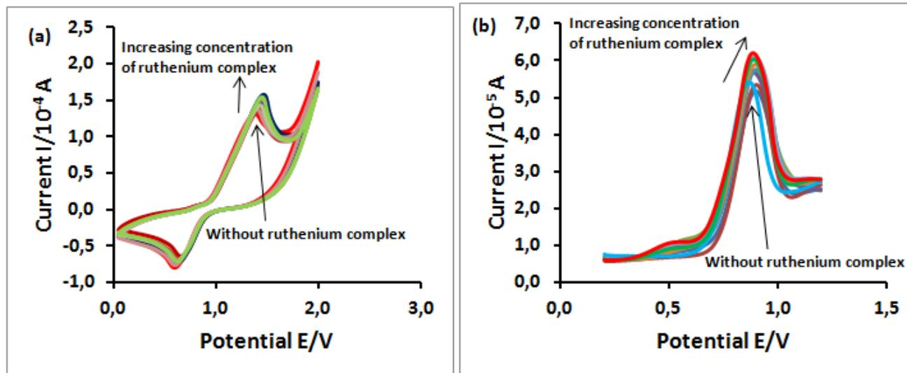
**Figure 2.** (a) CV and (b) DPV of Modified (PEDOT-PSS/AgNPs/AuE) electrode in ruthenium complex  $[Ru (phen)_2(qtpy)]^{2+}$  solution (in TE buffer).
