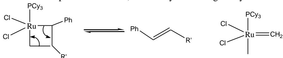
**Scheme 2.** Olefin metathesis reaction mechanism
