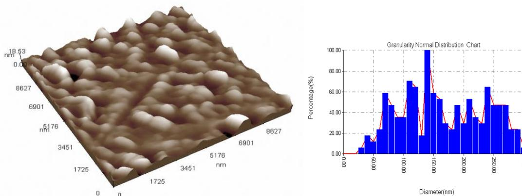
**Figure 6.** AFM image and granularity normal distribution chart of silicon film on amalgamated copper electrode under potentiostatic operation at -3.3V (vs.Pt.quasi-R.E) average particle size=161.05 nm
