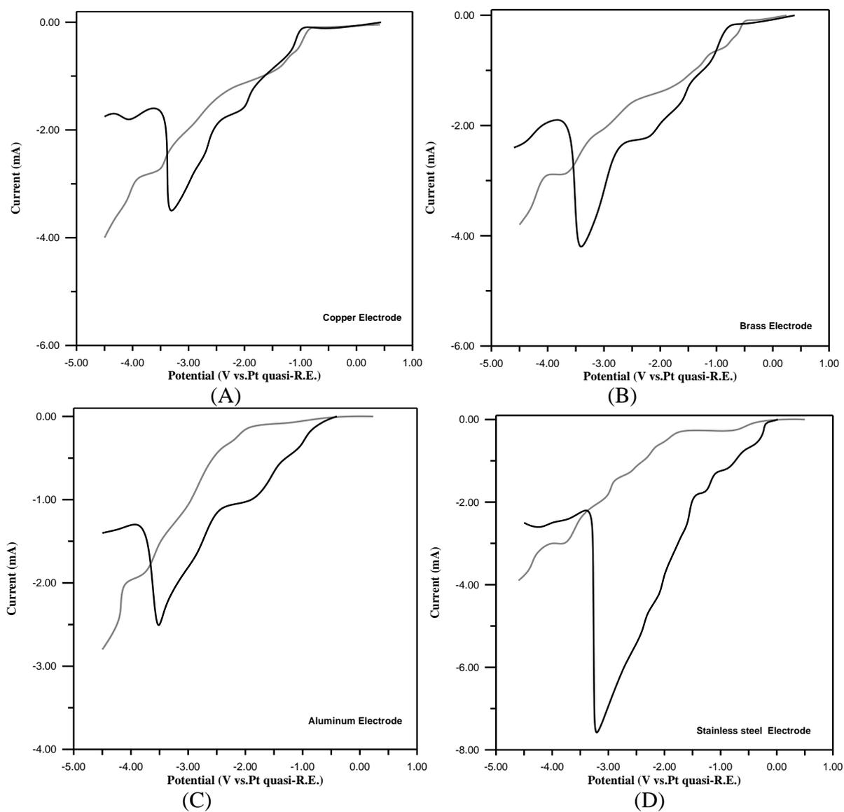
**Figure 2.** Linear sweep voltammograms of 0.6M phenyltrichlorosilane –0.07M TBACl–acetone electrolyte (black curve) and in 0.07M TBACl–acetone electrolyte (gray curve). Scan :10mV/s (in both case):A)Copper, B)Brass, C)Aluminum, D)Stainless steel(316)
