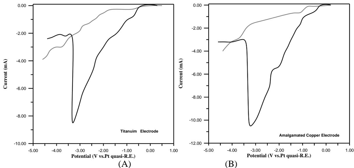
**Figure 3.** Linear sweep voltammograms of 0.6M phenyltrichlorosilane in 0.07M TBACl-acetone electrolyte (black curve) and in 0.07M TBACl-acetone electrolyte (gray curve). Scan rate :10mV/s (in both case): A) Titanium , B) Amalgamated copper electrode
