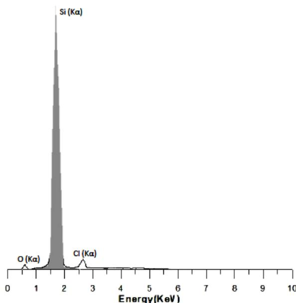
**Figure 5.** EDX spectrum for the sample electrodeposited at  $-3.3\text{V}$  (vs.Pt.quasi-R.E) for ( 4 hr.)potentiostatic operation on titanium cathode
