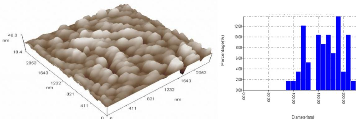
**Figure 7.** AFM image and granularity normal distribution chart of silicon film on titanium electrode at -3.3V (vs.Pt.quasi-R.E), average particle size=164.74 nm.
