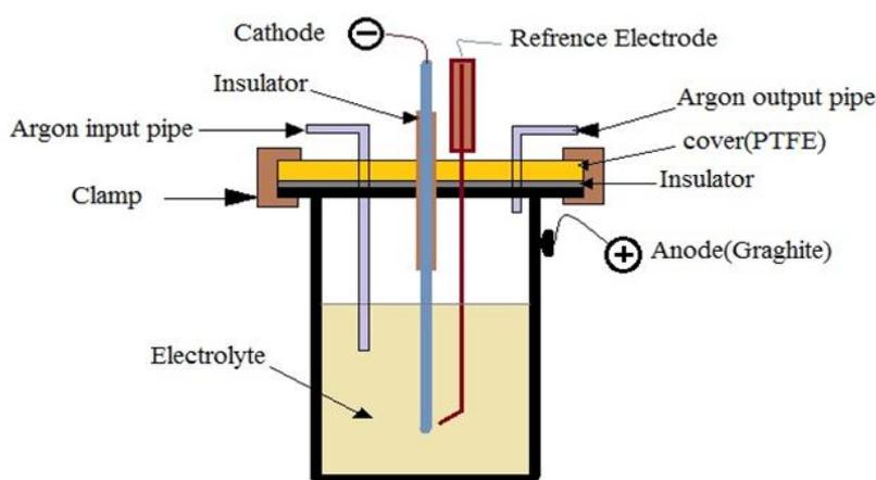
**Figure 1.** The electrolytic cell
