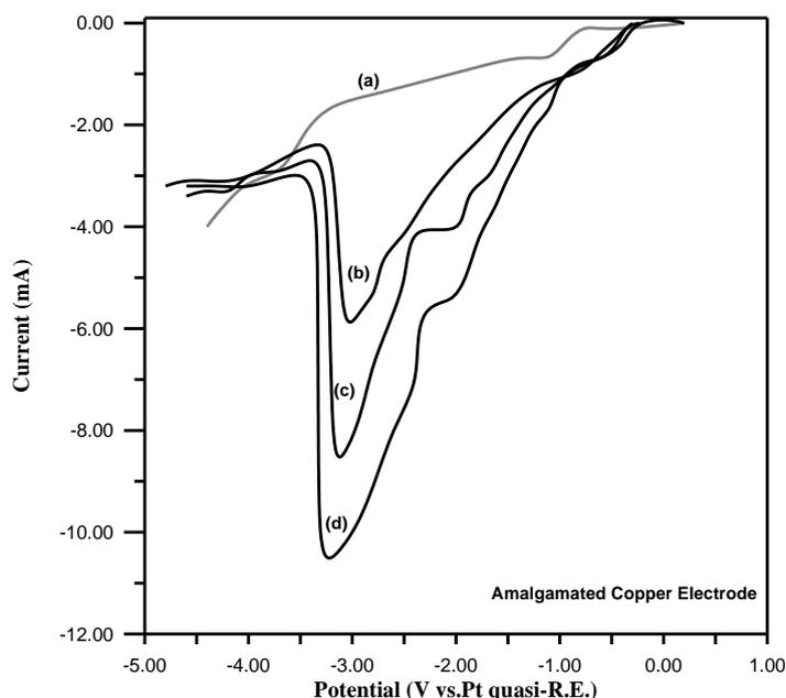
**Figure 4.** Linear sweep voltammograms of phenyltrichlorosilane in TBACl–Acetone electrolyte: a) without phenyltrichlorosilane, b)0.3M ,c)0.6M, d)1.2M. Scan rate: 10m V/s
