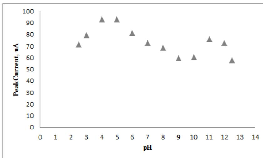
**Figure 9.** Plot of peak current versus pH (from 2 ~ 13) obtained at a SWCNT/ZnO-modified electrode for the oxidation of 3.5 mM ascorbic acid in a 0.1 M  $\text{KH}_2\text{PO}_4$  supporting electrolyte.
