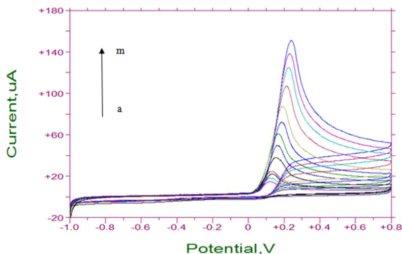
**Figure 6.** Plot of oxidation current versus ascorbic acid concentrations in  $0.1 \text{ M KH}_2\text{PO}_4$  using a SWCNT/ZnO-modified electrode at a scan rate of  $50 \text{ mV}/\text{s}$ . Ascorbic acid concentrations: (a)  $0.2$ , (b)  $0.5$ , (c)  $0.7$ , (d)  $1.0$ , (e)  $2.0$ , (f)  $3.0$ , (g)  $4.0$ , (h)  $5.0$ , (i)  $6.0$ , (j)  $7.0$ , (k)  $8.0$ , (l)  $9.0$  and (m)  $10.0 \text{ mM}$ .
