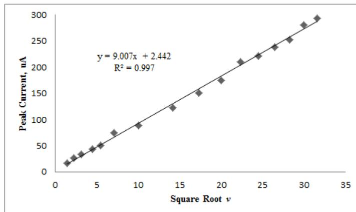
**Figure 4.** Plot of peak current versus square root of  $v$ . Other parameters, same as Fig. 2.
