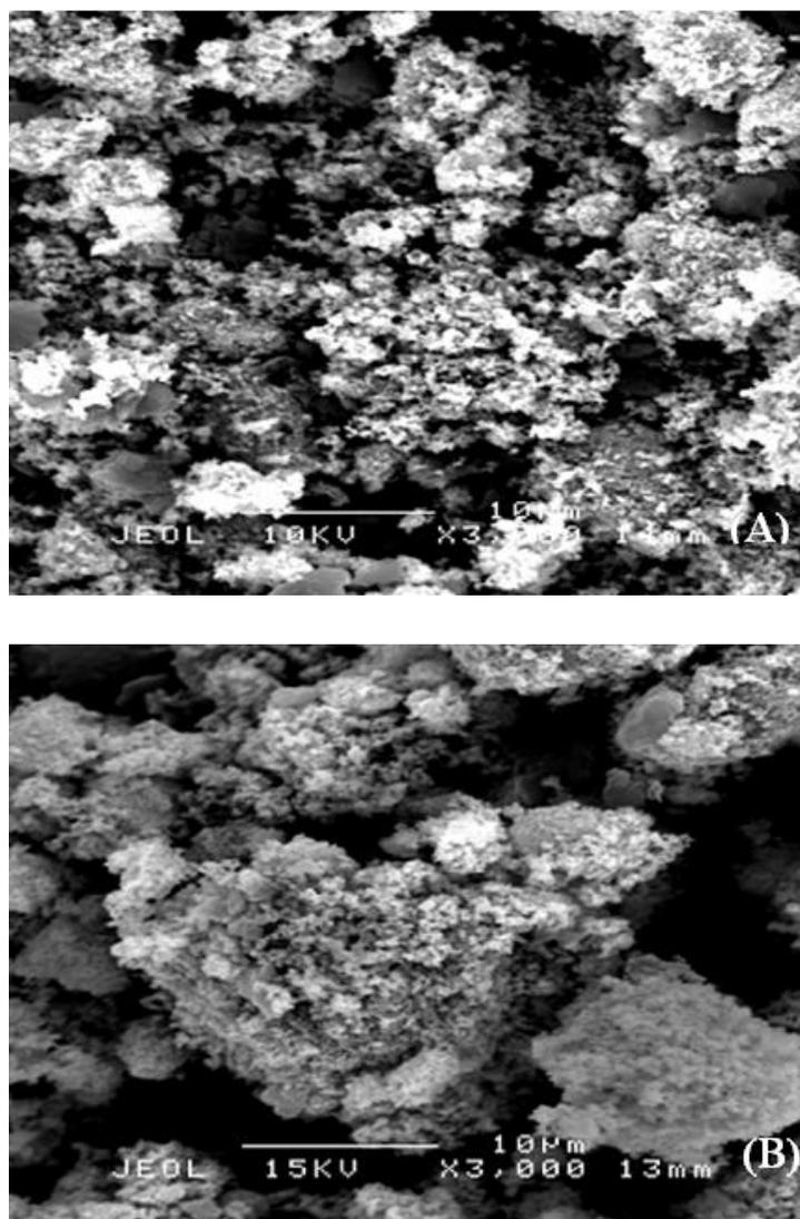
**Figure 10.** Scanning Electron Microscopy (SEM) of SWCNT/ZnO composites on a basal plane pyrolytic graphite electrode (BPPGE, 5 mm diameter) surface via mechanical attachment (A) before and (B) after the electroanalysis.
