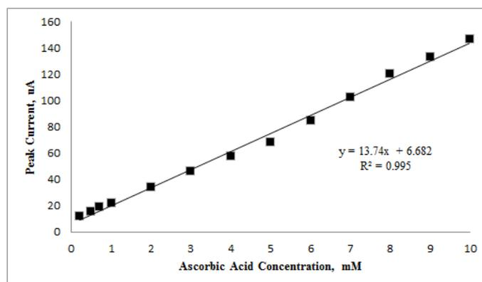
**Figure 7.** Calibration graph of ascorbic acid in  $0.1 \text{ M KH}_2\text{PO}_4$  using a SWCNT/ZnO-modified electrode versus  $\text{Ag}/\text{AgCl}$ .
