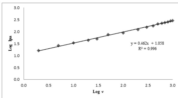
**Figure 3.** Plot of  $\log I_{pa}$  versus  $\log v$ . Other parameters, same as Fig. 2.
