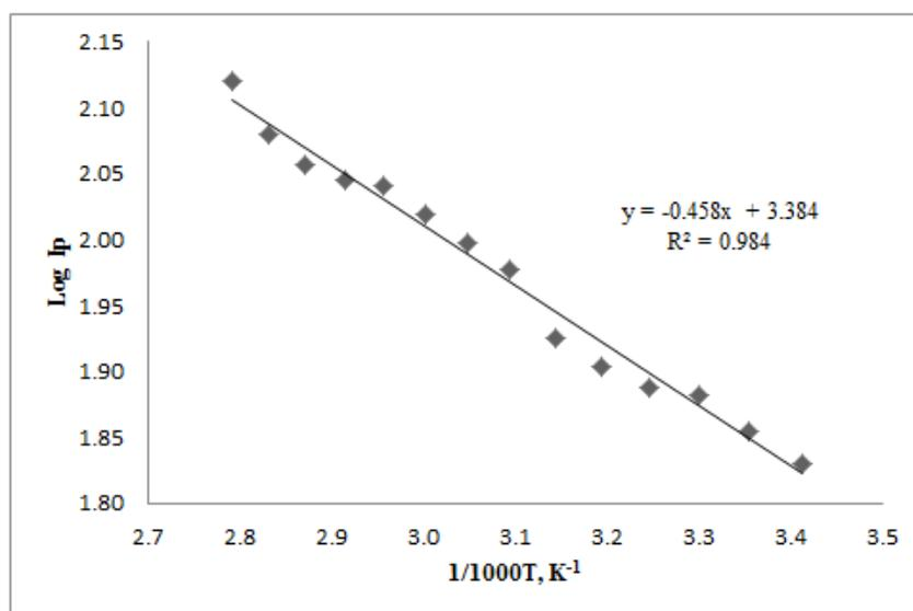
**Figure 8.** Plot of oxidative peak current versus reciprocal of temperature for the electrolysis of 3.5 mM ascorbic acid in 0.1 M  $\text{KH}_2\text{PO}_4$  at SWCNT/ZnO-modified electrode. Scan rate: 50 mV/s.
