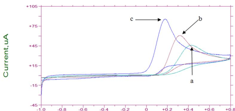
**Figure 1.** Cyclic voltammetry scanning of 3.5 mM ascorbic acid in 0.1 M  $\text{KH}_2\text{PO}_4$  at a scan rate of 50 mV/s for (a) bare electrode, (b) ZnO-modified electrode and (c) SWCNT/ZnO-modified electrode.
