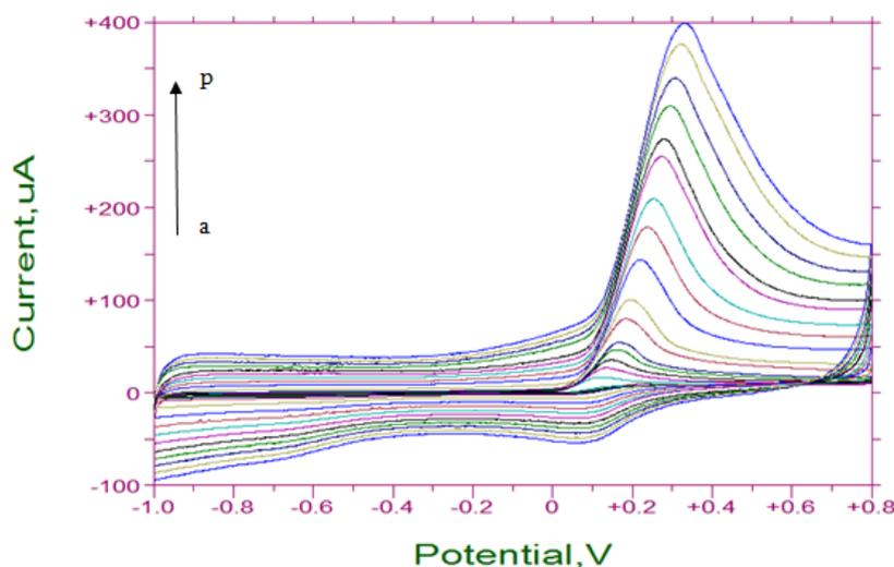
**Figure 2.** Effect of varying scan rate for 3.5 mM ascorbic acid in 0.1 M  $\text{KH}_2\text{PO}_4$  at SWCNT/ZnO-modified electrode versus Ag/AgCl. Scan rates: (a) 2, (b) 5, (c) 10, (d) 20, (e) 30, (f) 50, (g) 100, (h) 200, (i) 300, (j) 400, (k) 500, (l) 600, (m) 700, (n) 800, (o) 900, and (p) 1000 mV/s.
