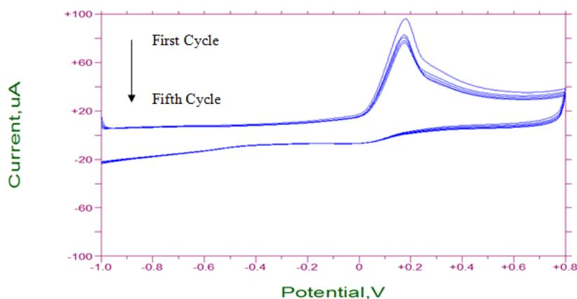
**Figure 5.** Multiple cycle voltammetry for 3.5 mM ascorbic acid in 0.1 M  $\text{KH}_2\text{PO}_4$  at a SWCNT/ZnO-modified electrode. Scan rate: 50 mV/s.
