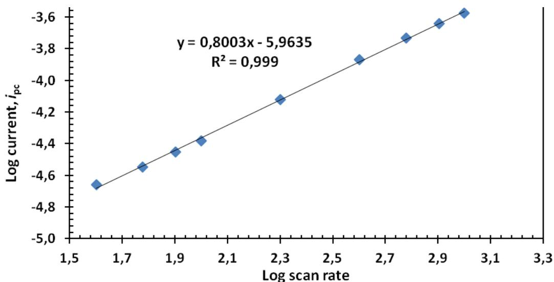
**Figure 7.** Dependence of log cathodic current on log scan rate for Biotinyl peptide/Nafion modified gold electrode in  $10 \text{ mgL}^{-1} \text{ Hg(II)}$  and  $0.1 \text{ M Na}_2\text{SO}_4$  as supporting electrolyte (pH 3) with potential scanning commenced in negative direction over the range 1.5 to  $-0.25 \text{ V vs Ag/AgCl}$  at a scan rate of 10 to  $1000 \text{ mVs}^{-1}$ .
