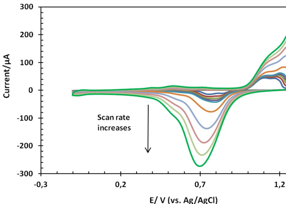
**Figure 6.** Effect of varying the scan rate on the cyclic voltammogram of Biotinyl peptide/Nafion modified gold electrode in  $10 \text{ mgL}^{-1} \text{ Hg(II)}$  and  $0.1 \text{ M Na}_2\text{SO}_4$  as supporting electrolyte (pH 3). Potential scanning commenced in negative direction over the range 1.5 to  $-0.25 \text{ V vs Ag/AgCl}$  at a scan rate 20 to  $1000 \text{ mVs}^{-1}$ .
