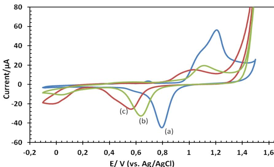
**Figure 2.** Cyclic voltammetry pattern of (a) Biotinyl peptide/Nafion modified gold electrode in  $10 \text{ mgL}^{-1}$  Hg(II), (b) Nafion modified gold electrode in  $10 \text{ mgL}^{-1}$  Hg(II) and (c) Biotinyl peptide/Nafion modified gold electrode without Hg(II) with  $0.1 \text{ M Na}_2\text{SO}_4$  (pH 3) as supporting electrolyte with potential scanning commenced in negative direction over the range  $1.5$  to  $-0.1$  V vs Ag/AgCl.
