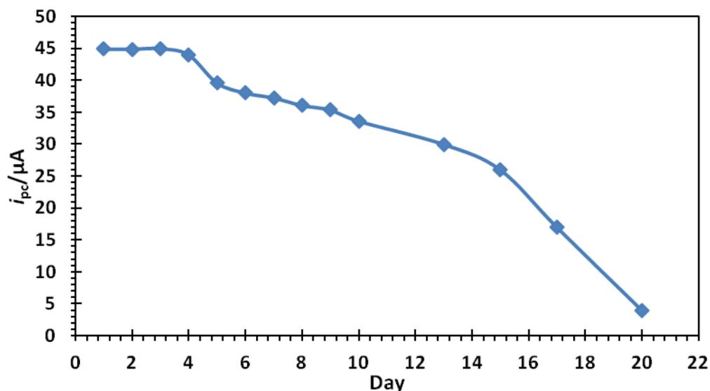
**Figure 4.** A graph of stability study for determination of 10 mgL<sup>-1</sup> Hg(II) using Biotinyl peptide/Nafion modified gold electrode in 0.1 M Na<sub>2</sub>SO<sub>4</sub> (pH 7) as supporting electrolyte. Potential scanning in negative direction from 0.9 to 0.2 V vs Ag/AgCl at a scan rate 100 mVs<sup>-1</sup>.
