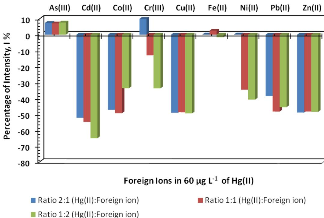
**Figure 9.** Effect of foreign metal ions using Biotinyl peptide/Nafion modified gold electrode in  $0.1 \text{ M Na}_2\text{SO}_4$  (pH 3) as supporting electrolyte. Potential scanning in negative direction from 1.5 to  $-0.25 \text{ V vs Ag/AgCl}$  at a scan rate  $100 \text{ mVs}^{-1}$ .
