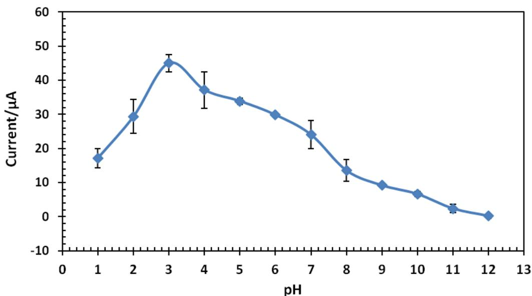
**Figure 3.** Reduction peak current at  $25^\circ\text{C}$  for  $10 \text{ mgL}^{-1}$  Hg(II) in  $0.1 \text{ M Na}_2\text{SO}_4$  as supporting electrolyte as a function of pH using Biotinyl peptide/Nafion modified gold electrode. Potential scanning in negative direction from 1.5 to  $-0.1 \text{ V}$  vs Ag/AgCl at a scan rate  $100 \text{ mVs}^{-1}$ .
