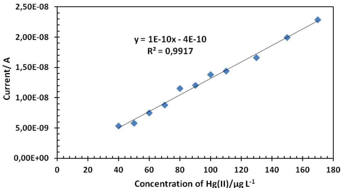
**Figure 11.** Calibration plot of current intensity versus concentration of Hg(II) concentration using Biotinyl peptide/Nafion modified gold electrode in 0.1 M Na<sub>2</sub>SO<sub>4</sub> (pH 3) as supporting electrolyte. Potential scanning in negative direction from 0.95 to 0.6 V vs Ag/AgCl.
