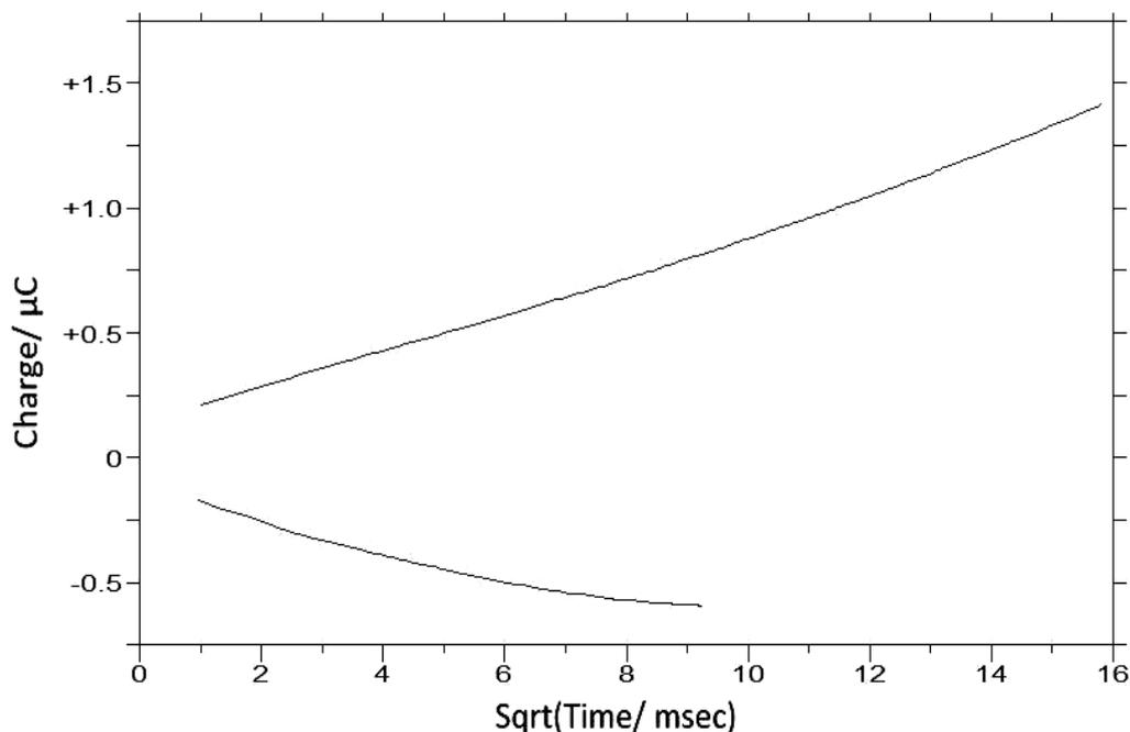
**Figure 8.** Charge versus square root of time of double step chronocoulograms of  $0.5 \text{ mgL}^{-1}$  Hg(II) using Biotinyl peptide/Nafion modified gold electrode in  $0.1 \text{ M Na}_2\text{SO}_4$  (pH 3), potential scanning from 0.07 to 0.17 V vs Ag/AgCl.
