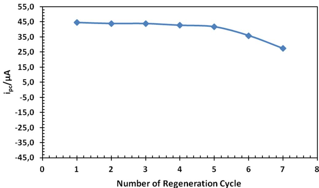
**Figure 5.** A graph of repeatability study for determination of  $10 \text{ mgL}^{-1}$  Hg(II) using Biotinyl peptide/Nafion modified gold electrode in  $0.1 \text{ M Na}_2\text{SO}_4$  (pH 3) as supporting electrolyte. Potential scanning in negative direction from 1.5 to  $-0.25 \text{ V}$  vs Ag/AgCl at a scan rate  $100 \text{ mVs}^{-1}$ .
