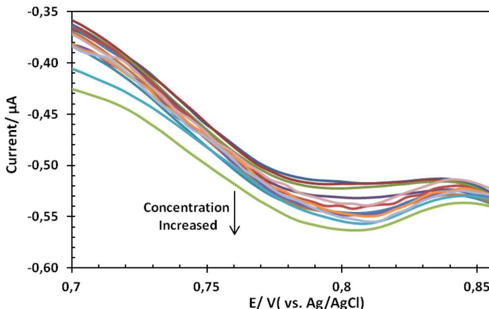
**Figure 10.** Voltammograms of Biotinyl peptide/Nafion modified gold electrode in 0.1 M  $\text{Na}_2\text{SO}_4$  (pH 3) supporting electrolyte with different concentration of Hg(II). Potential scanning in negative direction from 0.95 to 0.6 V vs Ag/AgCl.
