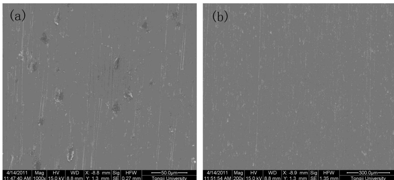
**Figure 1.** SEM images of a magnesium alloy sheet. (a) solvent degreased; (b) etched in phosphoric acid
