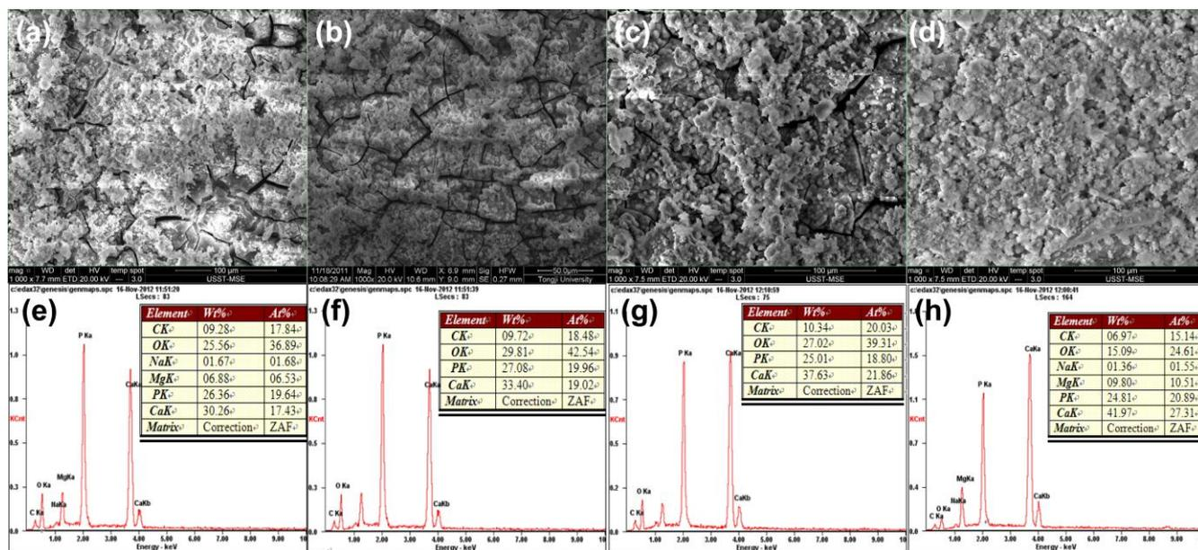
Figure 3. SEM morphologies and corresponding EDS patterns of coated samples. 0.5×R-SBF: (a)/(e) ; 1×R-SBF: (b)/(f); 1.5×R-SBF: (c)/(g); 2×R-SBF: (d)/(h)
