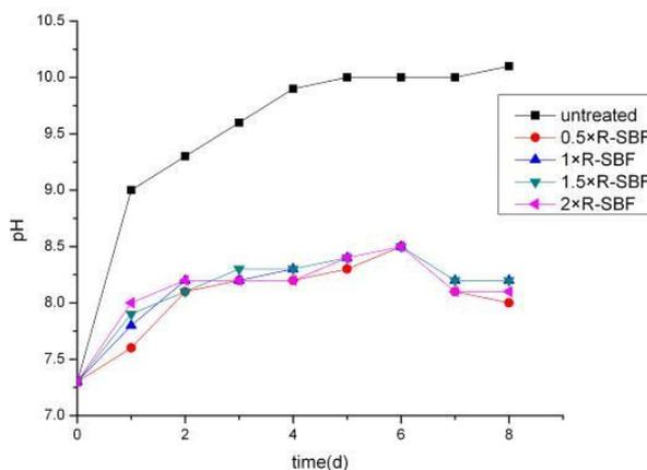
**Figure 6.** Variation of the pH value of SBF solution at different immersion time
