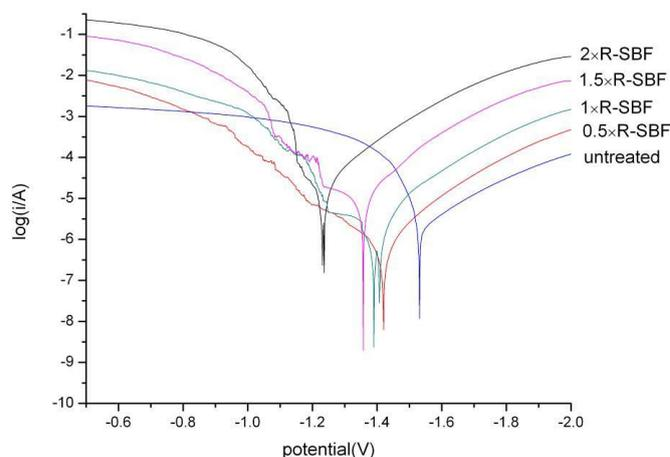
**Figure 4.** Tafel plot of the samples in SBF solution
