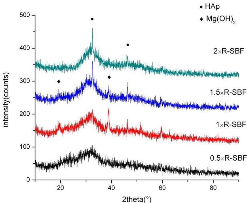
Figure 2. XRD patterns of coating powders in solutions with different Ca/P ratio
