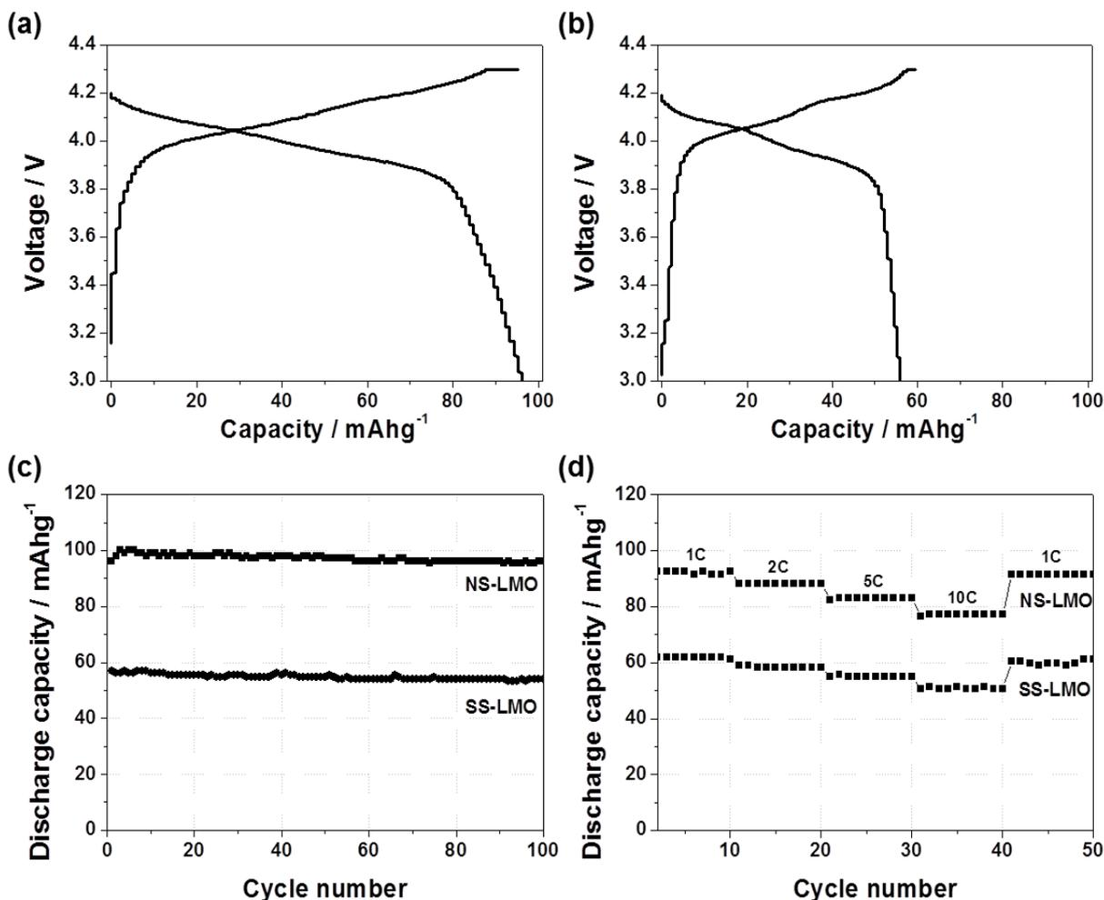
**Figure 4.** Charge-discharge curves of (a) NS-LMO and (b) SS-LMO at 1 C. (c) Cycle performance of NS-LMO and SS-LMO at 1 C for 100 cycles. (d) Rate cycling performance of NS-LMO and SS-LMO from 1 C to 10 C.
