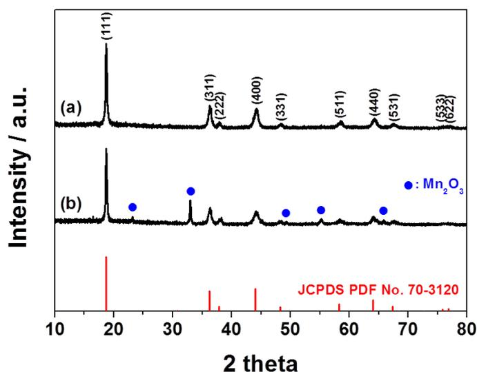
**Figure 1.** XRD patterns of (a) NS-LMO and (b) SS-LMO.
