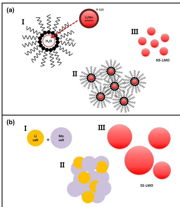
**Scheme 1.** Schematic representation of synthesis of NS-LMO using PT method and SS-LMO using SSR method.
