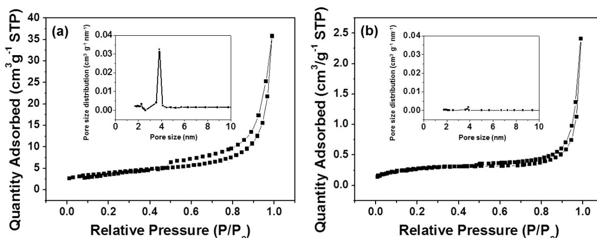
**Figure 3.** Nitrogen adsorption/desorption isotherms for (a) NS-LMO and (b) SS-LMO. The insets are pore size distributions of the samples.
