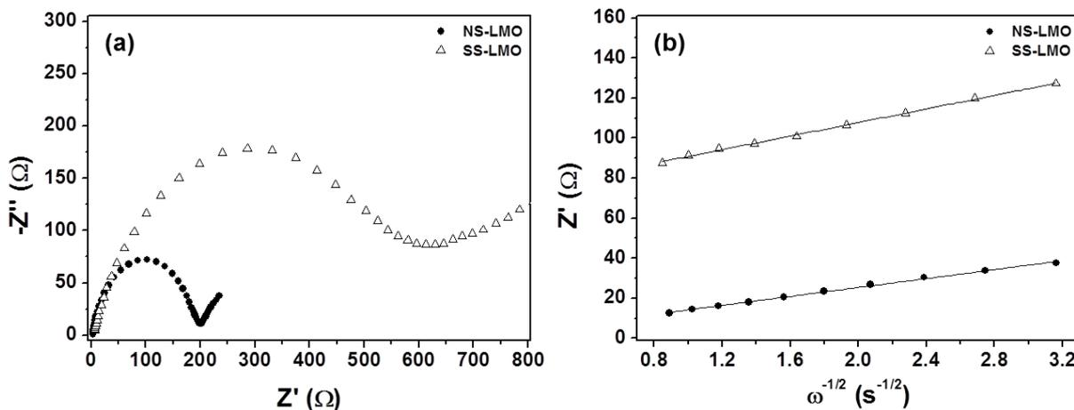
**Figure 5.** (a) Nyquist plots of NS-LMO and SS-LMO at 1 C in the frequency ranged between 100 kHz and 10 mHz.
