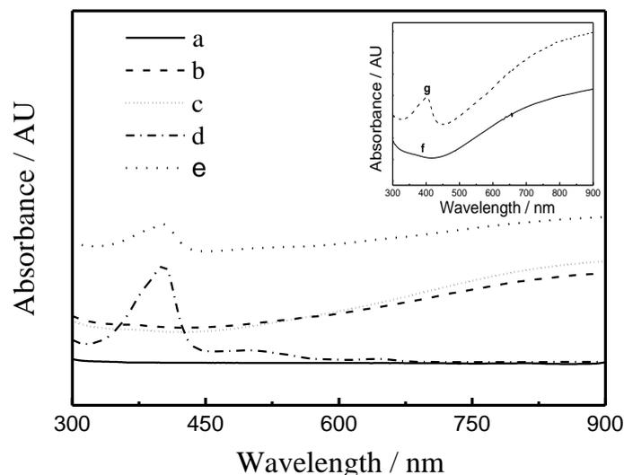
**Figure 2.** UV-vis absorption spectra of (a) Nafion, (b) PEDOT:PSS, (c) PEDOT:PSS-Nafion mixture, (d) HRP in pH 7.0 PBS, and (e) HRP in PEDOT:PSS-Nafion mixture. Inset: UV-vis absorption spectra of (f) AgNPs/PEDOT:PSS-Nafion and (g) Nafion/HRP/AgNPs/PEDOT:PSS-Nafion.
