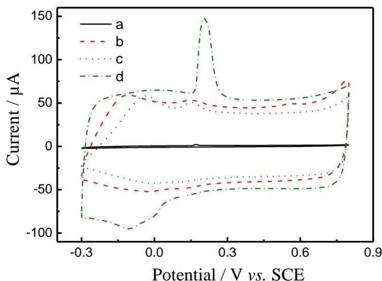
**Figure 4.** CVs of 40  $\mu\text{M}$   $\text{H}_2\text{O}_2$  in 0.1 M PBS (pH 7.0) at different electrodes: (a) bare GCE, (b) PEDOT:PSS-Nafion/GCE, (c) Nafion/HRP/PEDOT:PSS-Nafion/GCE, (d) Nafion/AgNPs/HRP/PEDOT:PSS-Nafion/GCE. Scan rate: 50  $\text{mV s}^{-1}$ .
