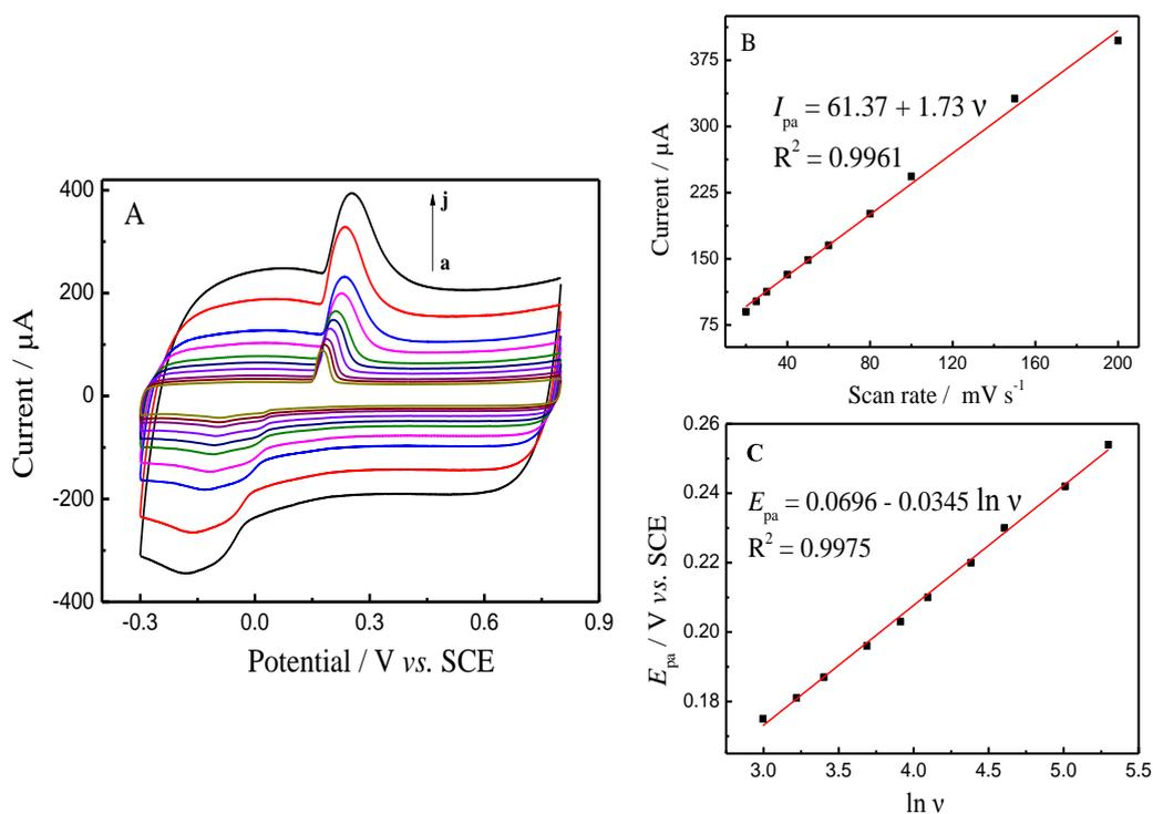
**Figure 6.** (A) CVs of 40  $\mu\text{M}$   $\text{H}_2\text{O}_2$  in 0.1 M PBS (pH 7.0) with different scan rates: 20, 25, 30, 40, 50, 60, 80, 100, 150, and 200  $\text{mV s}^{-1}$  (from a to j). (B) The plot of anodic peak currents vs. scan rate. (C) The plot of anodic peak potentials vs.  $\ln v$ .
