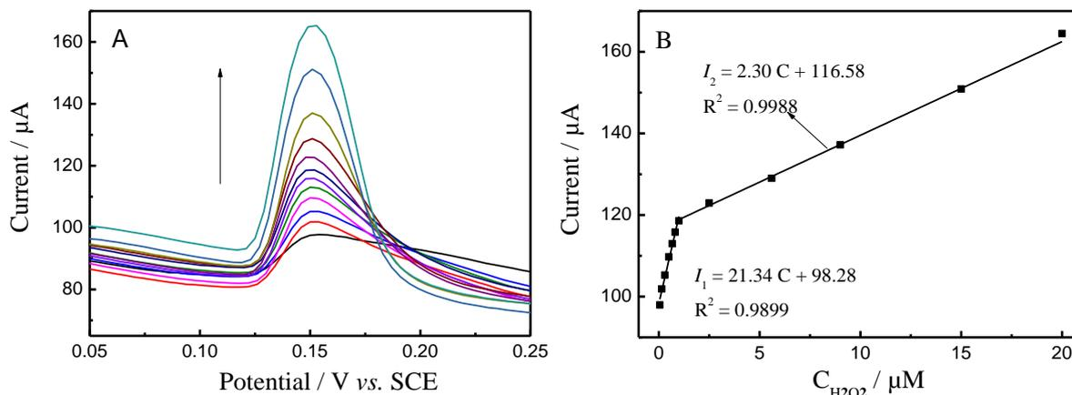
**Figure 7.** (A) DPVs of various concentrations of  $\text{H}_2\text{O}_2$  at Nafion/HRP/AgNPs/PEDOT:PSS-Nafion/GCE in 0.1 M PBS (pH 7.0).  $\text{H}_2\text{O}_2$  concentrations (from bottom to top): 0.05, 0.15, 0.3, 0.5, 0.67, 0.81, 1.0, 2.5, 5.6, 9, 15, and 20  $\mu\text{M}$ . Scan rate: 50  $\text{mV s}^{-1}$ . (B) The linear relationship between peak current and concentration of  $\text{H}_2\text{O}_2$ .
