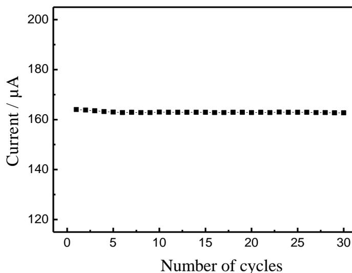
**Figure 8.** The stability of Nafion/HRP/AgNPs/PEDOT:PSS-Nafion/GCE containing 40  $\mu\text{M}$   $\text{H}_2\text{O}_2$  in 0.1 M PBS (pH 7.0). Scan rate: 50  $\text{mV s}^{-1}$ .
