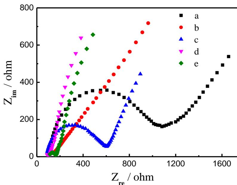
**Figure 3.** EIS for (a) bare GCE, (b) PEDOT:PSS-Nafion/GCE, (c) Nafion/HRP/PEDOT:PSS-Nafion/GCE, (d) AgNPs/PEDOT:PSS-Nafion/GCE, (e) Nafion/AgNPs/HRP/PEDOT:PSS-Nafion/GCE, in 5 mM  $[\text{Fe}(\text{CN})_6]^{4-/3-}$  containing 0.1 M KCl. The frequencies swept from 100 mHz to 10 kHz
