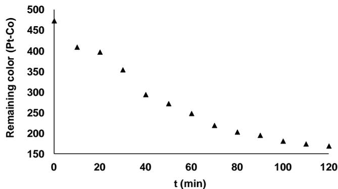
**Figure 6.** Remaining color as function of contact time of the wastewater treated in the ozone-electrocoagulation process.
