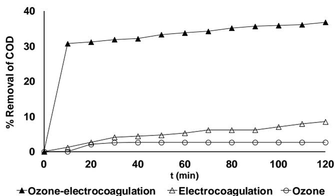
**Figure 3.** COD removal efficiency in the wastewater treated by means of three different processes
