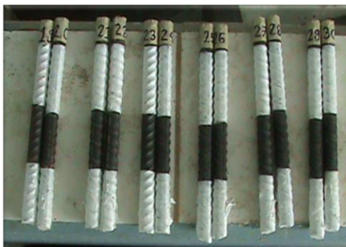
Figure 4. Distribution of rebars in the soil, for their monitoring.
