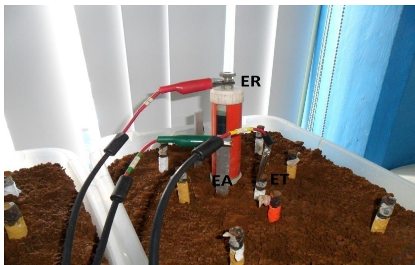
Figure 5. Electrochemical cell for experimentation.
