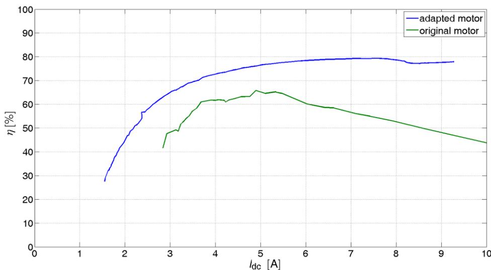
Figure 8. b) The dependences of the resultant efficiency  $\eta$  on the current  $I_{dc}$  taken from the AEROPACK
