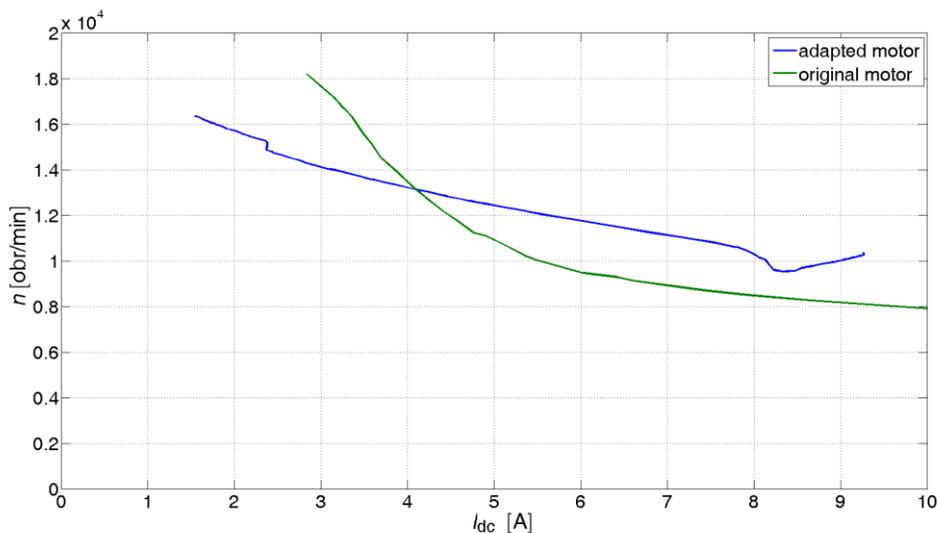
Figure 8. a) The dependences of the propeller speed  $n$  on the current  $I_{dc}$  taken from the AEROPACK
