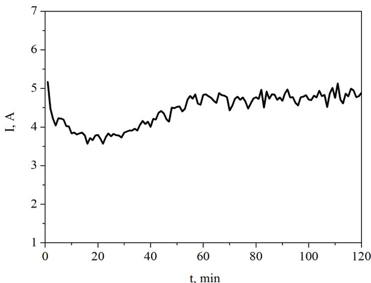
**Figure 5. b)** dependence of the current ( $I$ ) on the time during loading with the constant voltage  $U = 24$  V
