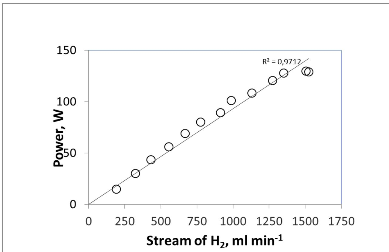
**Figure 4.** The dependence of the stream of hydrogen on the electric power produced by the AEROPACK fuel cell stack.
