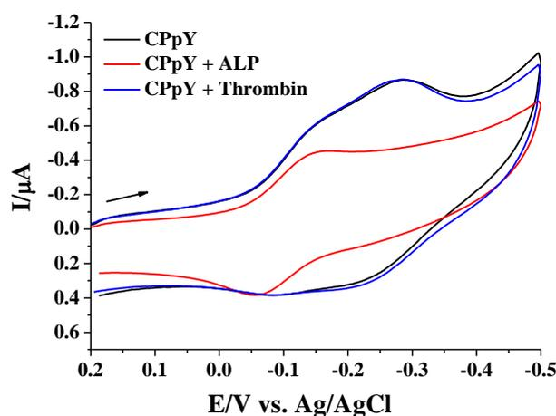
**Figure 4.** CVs acquired at the electrode pretreated with CPpY alone, CPpY/ALP and CPpY/thrombin before the modification of MCH. The scan rate was 100 mV/s. The concentration of both ALP and thrombin was 200 ng/mL.
