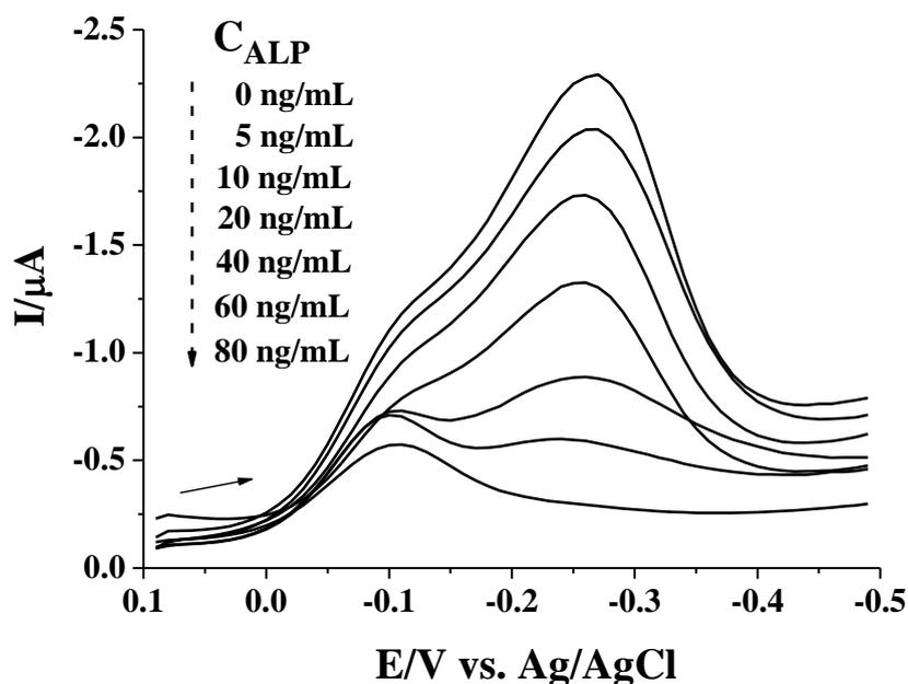
**Figure 6.** DPVs acquired at the electrode pretreated with CPpY and different concentrations of ALP before the modification of MCH. The other experimental conditions were the same as those in Fig. 4.
