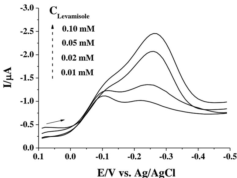
**Figure 7.** DPVs acquired at the electrode pretreated with CPyY/ALP in the presence of different concentrations of levamisole. The concentration of ALP was 80 ng/mL. The other experimental conditions were the same as those in Fig. 4.
