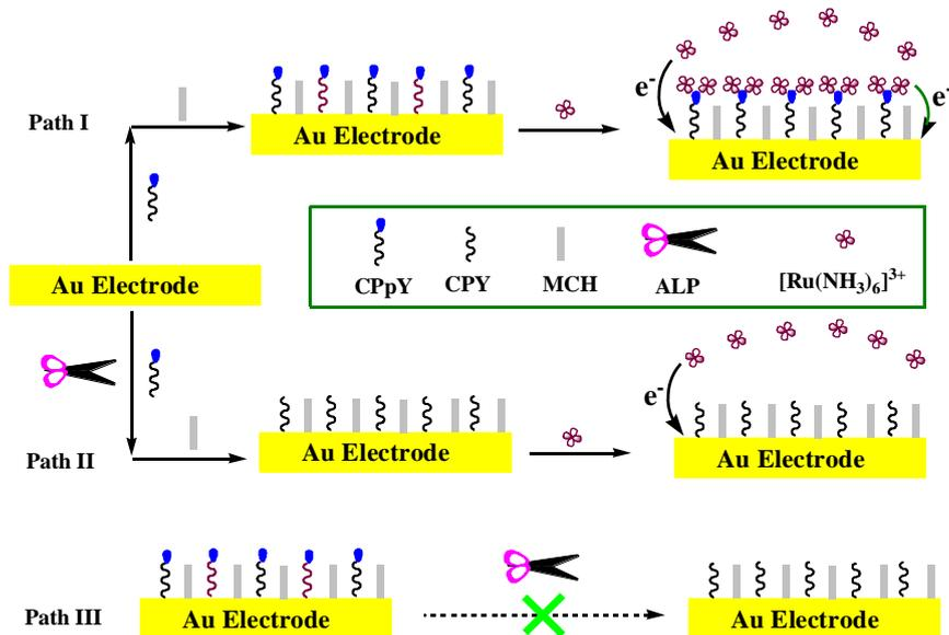
**Figure 1.** Scheme representation showing the strategy for probing of ALP activity based on the difference of interfacial features of the electrode.
