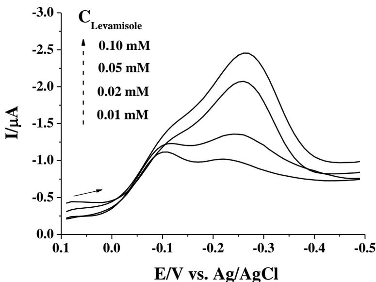
**Figure 7.** DPVs acquired at the electrode pretreated with CPpY/ALP in the presence of different concentrations of levamisole. The concentration of ALP was 80 ng/mL. The other experimental conditions were the same as those in Fig. 4.
