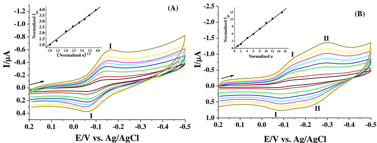
**Figure 3.** CVs acquired at CPY/MCH- (A) and CPpY/MCH- (B) covered electrodes in  $[\text{Ru}(\text{NH}_3)_6]^{3+}$  solution at different scan rate (10, 20, 40, 60, 80, 100, 120 and 150 mV/s). The arrow indicates the scan direction.
